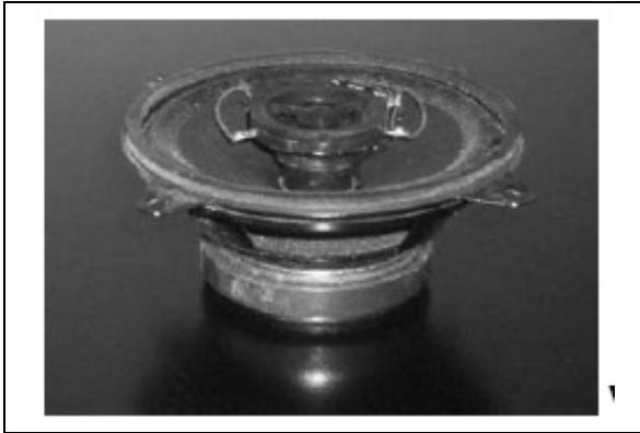
FIGURE 10: 10CM COAXIAL SPEAKER
