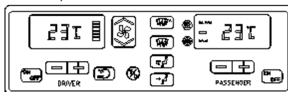
FIGURE 5: CENTRAL HVAC SYSTEM CONTROL UNIT 22296
