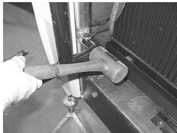
FIGURE 63: PANTOGRAPH ARM ADJUSTMENT
