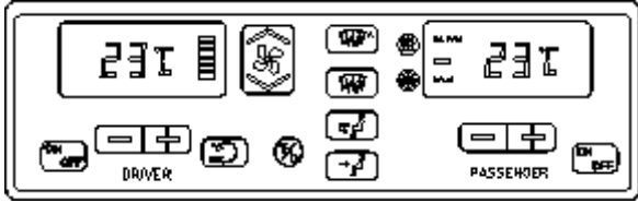
FIGURE 6: CENTRAL HVAC SYSTEM CONTROL UNIT
