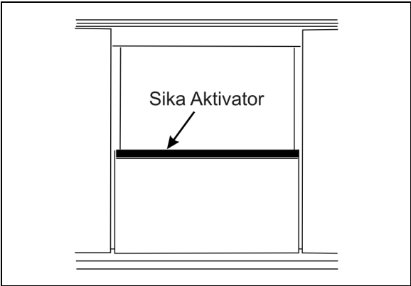
FIGURE 72 : SLIDING WINDOW - SIKa AKTIVATOR
