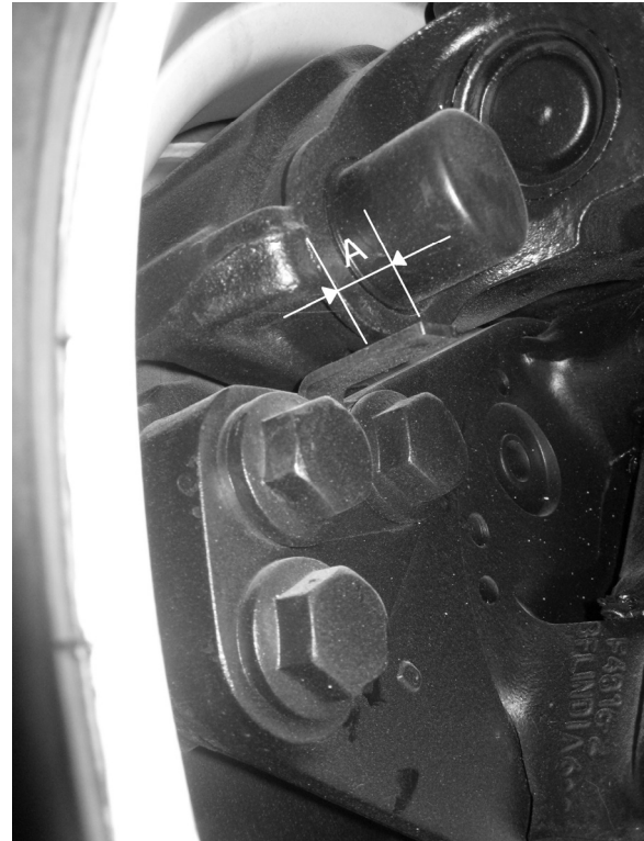
FIGURE 25: BRAKE PAD WEAR INSPECTION 12119
