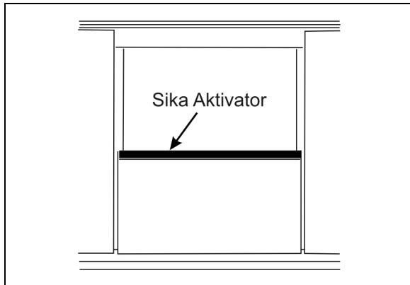
FIGURE 72 : SLIDING WINDOW - SIKA AKTIVATOR
