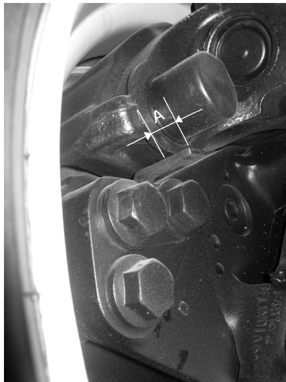
FIGURE 25: BRAKE PAD WEAR INSPECTION
