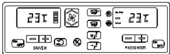
CENTRAL HVAC SYSTEM CONTROL MODULE
