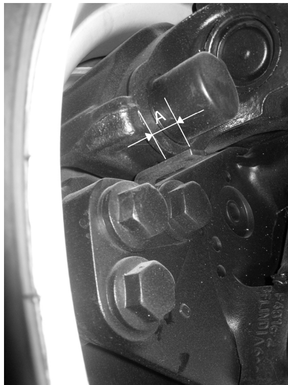
FIGURE 25: BRAKE PAD WEAR INSPECTION
