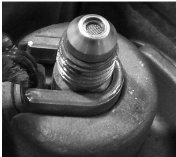
FIGURE 13 : AFTERTREATMENT FUEL INJECTOR INLET SCREEN
