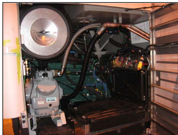
FIGURE 7: REAR ELECTRICAL PANEL, JUNCTION PANEL & BATTERY COMPARTMENT
