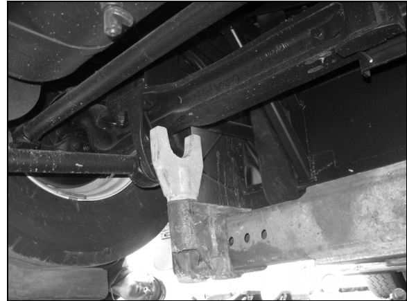
LIFTING FROM UNDER THE FRONT AXLE
