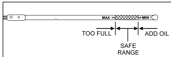
VOLVO D13 ENGINE OIL LEVEL DIPSTICK
