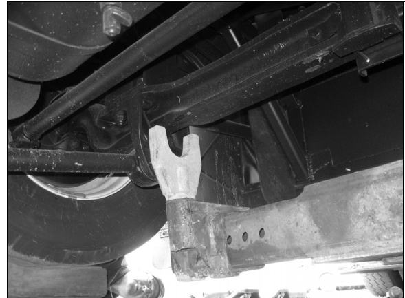
LIFTING FROM UNDER THE FRONT AXLE
