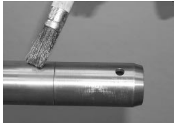
FIGURE 18: APPLY GLEITMO 805 GREASE
