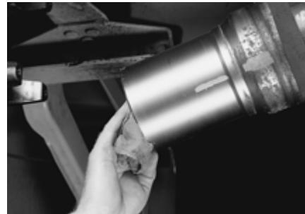
FIGURE 22: CLEAN GREASE FROM SPLINE SLEEVE
