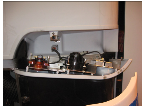
FIGURE 41: HEADLIGHT ASSEMBLY OPENED FOR BULB REPLACEMENT 06547
