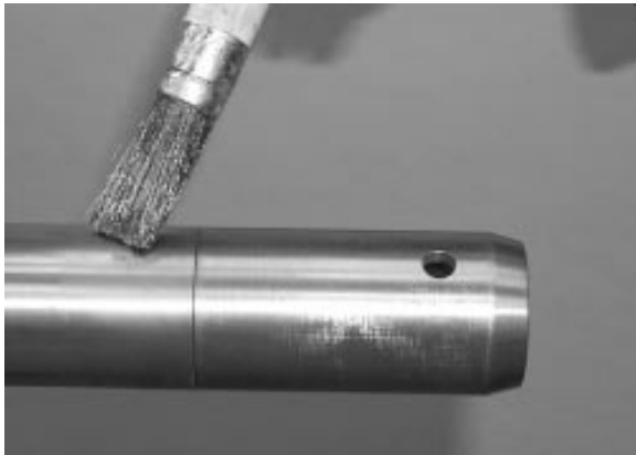
FIGURE 9: APPLY GLEITMO 805 GREASE
