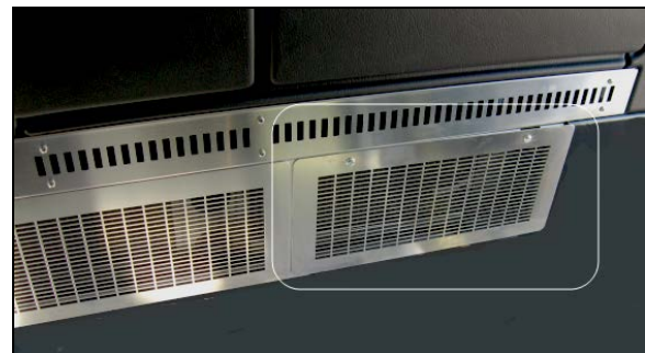
ACCESS TO DRIVER'S HVAC UNIT AIR FILTERS
