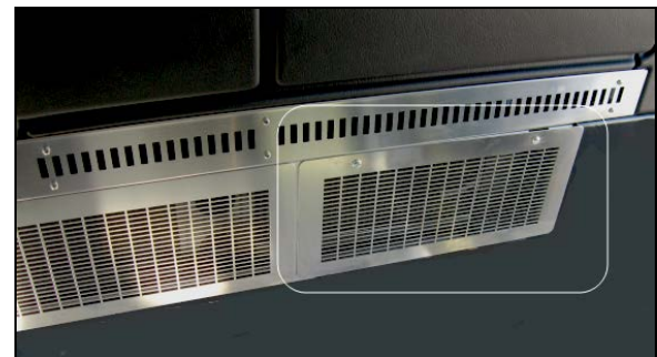
ACCESS TO DRIVER'S HVAC UNIT AIR FILTERS
