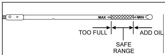
VOLVO D13 ENGINE OIL LEVEL DIPSTICK
