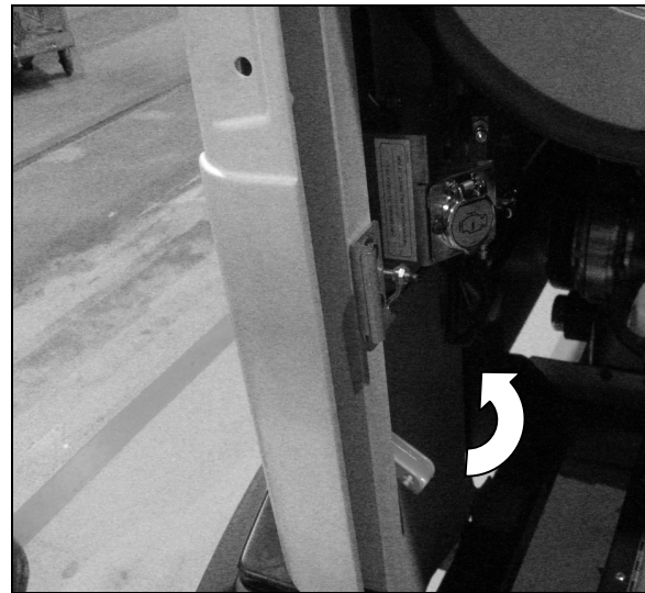
OPENING THE ENGINE COMPARTMENT REAR DOOR FROM R.H. SIDE DOOR 18608
