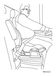
Tether straps are installed on all suspension/type seats. Tether straps help secure the seat to the floor and are intended to restrain the seat and safety belt in case of an accident or sudden stop. The tether are no adjustable and do not need any adjustment.
