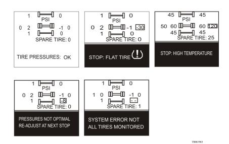
A rectangle around each pressure/temperature reading of the tires that have an issue is blinking to draw the attention to the defective tires.
