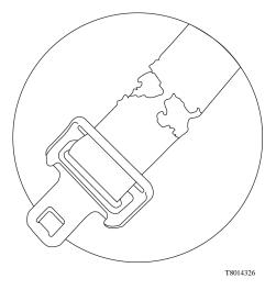
Check the buckle by inserting the latch and verifying proper operation. Determine if the latch plat is worn or deformed. Check the buckle and latch casing for cracks or breakage
