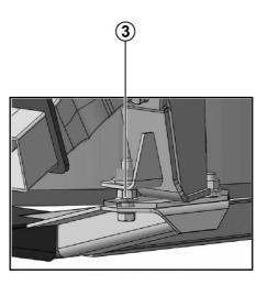
Rotate the front under run protection brace upward (1) and install the brackets with the screws (2,3).
