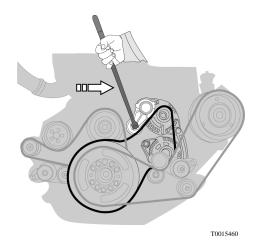
Turn the belt and pass it through the damper and intermediate pulley, and pull down.
