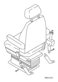
All hardware for safety belt mounting points should be evaluated for corrosion. All attachment points of the system should be checked for tightness of mounting hardware.
