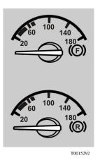
F. Air Pressure, front brake circuit R. Air pressure, rear brake circuit
