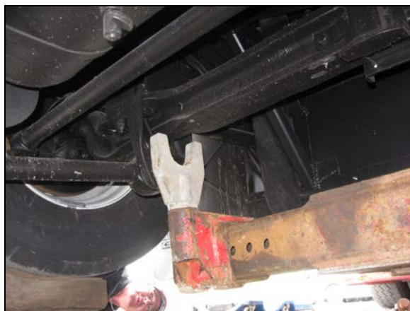
LIFTING FROM UNDER THE FRONT AXLE
