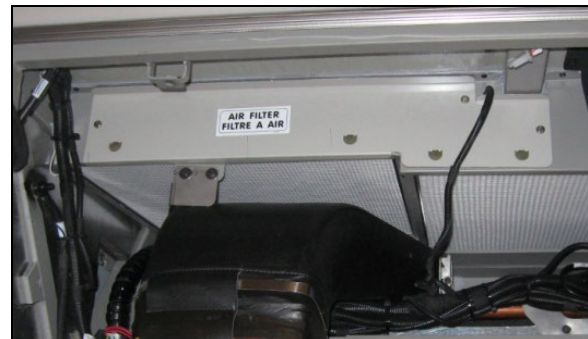
PASSENGERS AREA AIR FILTER REMOVAL
