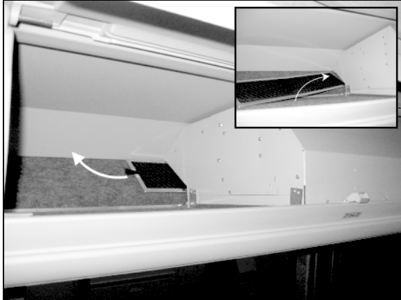
OVERHEAD COMPARTMENT FAN AIR FILTER
