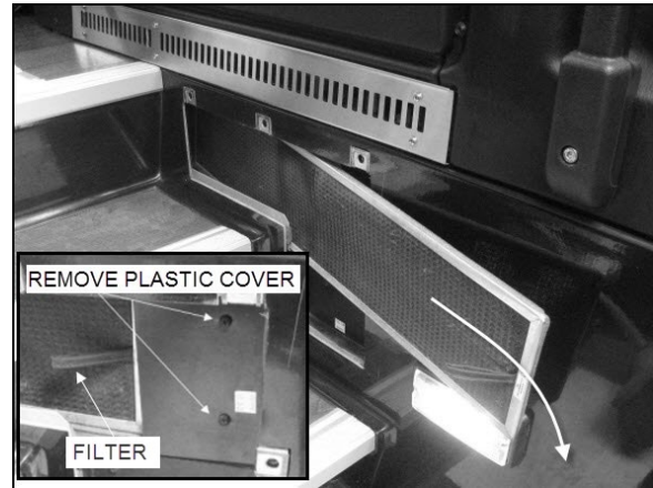
REMOVING DRIVER'S SECTION AIR FILTER
