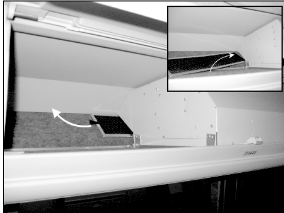
OVERHEAD COMPARTMENT FAN AIR FILTER
