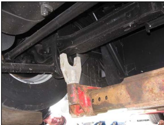
LIFTING FROM UNDER THE FRONT AXLE
