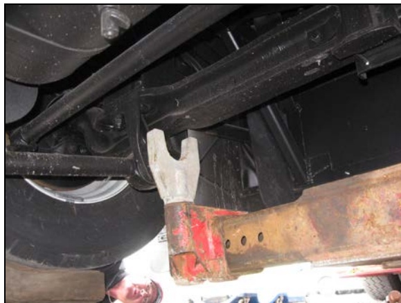
LIFTING FROM UNDER THE FRONT AXLE
