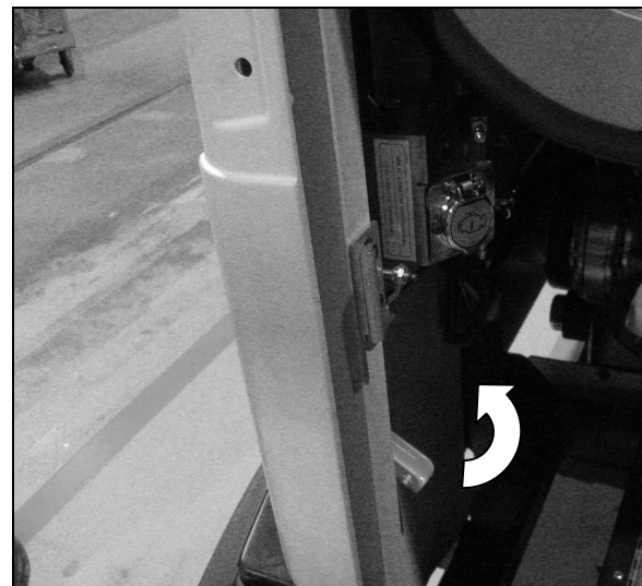
OPENING ENGINE COMPARTMENT REAR DOOR 18608
