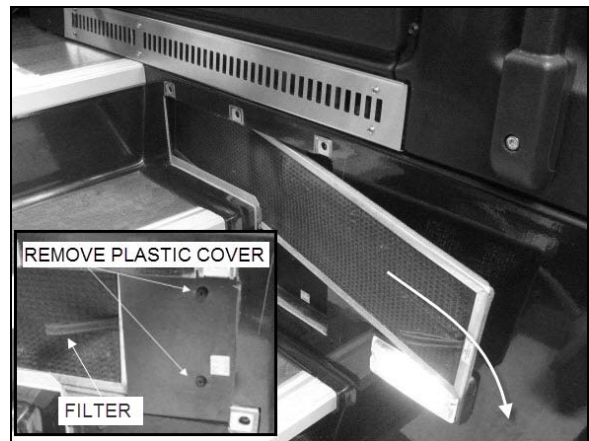
REMOVING DRIVER'S SECTION AIR FILTER
