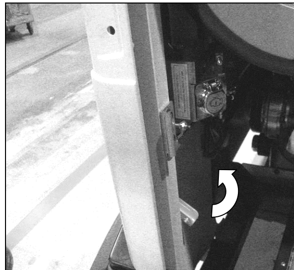
OPENING ENGINE COMPARTMENT REAR DOOR
