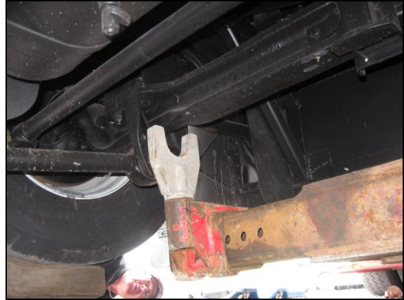
LIFTING FROM UNDER THE FRONT AXLE
