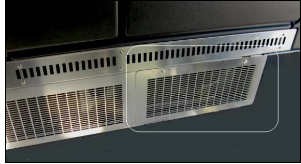
ACCESS TO DRIVER'S HVAC UNIT AIR FILTER
