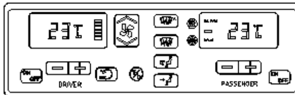
CENTRAL HVAC SYSTEM CONTROL MODULE 22296
