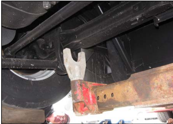
LIFTING FROM UNDER THE FRONT AXLE
