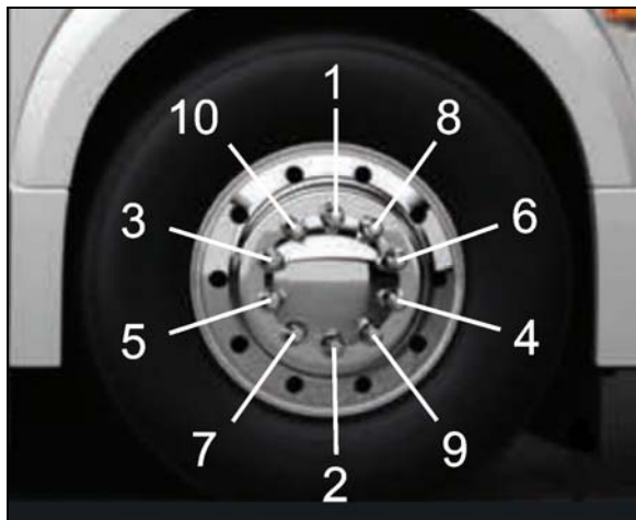
TIGHTENING SEQUENCE
