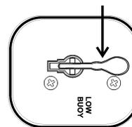
COMMANDE DU SYSTÈME D'ABAISSMENT DE LA SUSPENSION 12165
