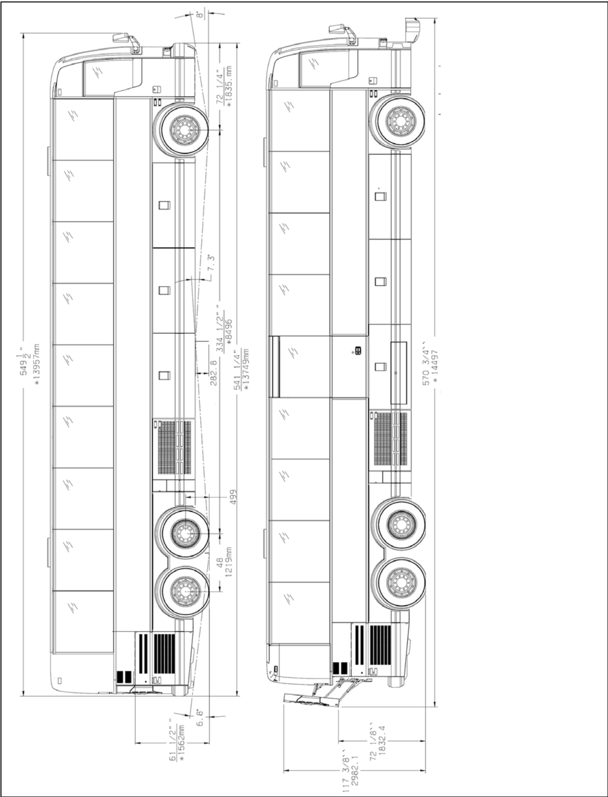
X3-45 OVERALL DIMENSIONS (SIDE ELEVATION)
