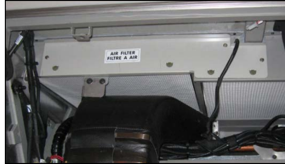
PASSENGERS AREA AIR FILTER REMOVAL
