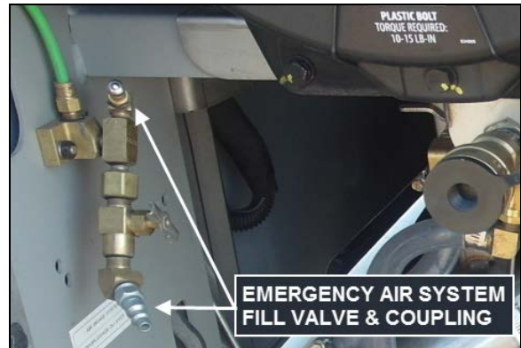
EMERGENCY AIR SYSTEM FILL VALVE AND COUPLING
