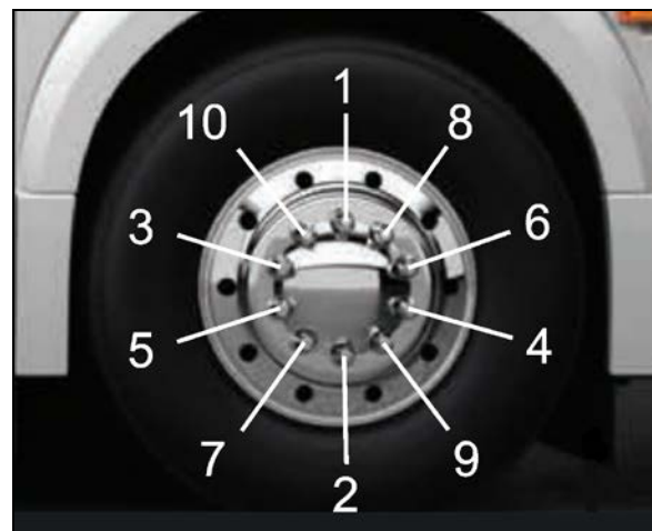
TIGHTENING SEQUENCE
