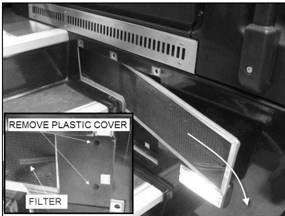
REMOVING DRIVER'S SECTION AIR FILTER
