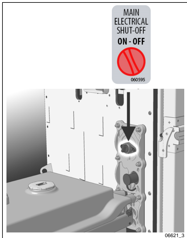
MAIN ELECTRICAL SHUT-OFF SWITCH
