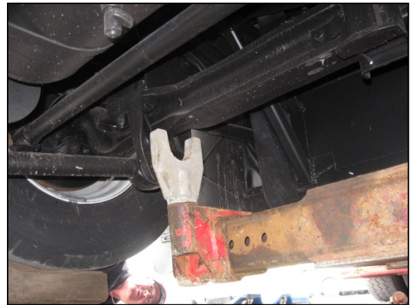
LIFTING FROM UNDER THE FRONT AXLE
