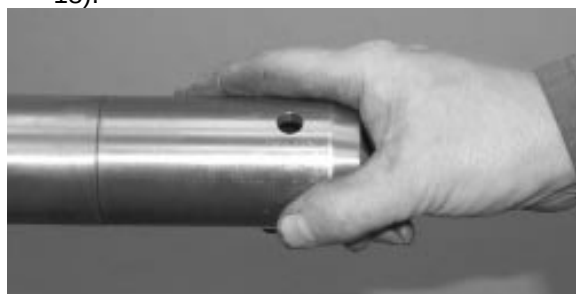
FIGURE 18: OUTIL D'INSERTION NIP PREVOST 491115
