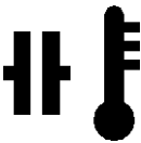
These icons will appear on the cluster if clutch overheats
