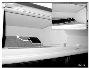
OVERHEAD COMPARTMENT FAN AIR FILTER
