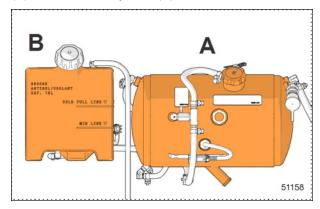
Check the coolant level into the recovery tank (B) when the engine is cold (room or ambient temperature).
