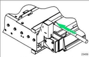
4. Rotate the keyed release shaft ¼-turn (as indicated on adjacent decal) while lifting stow lock lever simultaneously.
