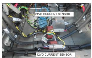
12VD / 24VD CURRENT SENSORS IN MPC
