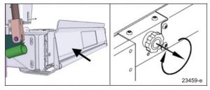
Close the backup pump release valve by pushing the actuating rod (A) DOWN (release valve should already be closed).
