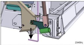
2. Raise the platform to stow height; position the top surface of the platform lifting frame arm at the same height as the top surface of the carriage. If the exact height cannot be obtained, a slightly low platform is preferred to slightly high. This alignment eliminates interference between the platform and enclosure when pushing the platform into the enclosure.
