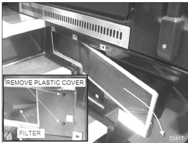
REMOVING DRIVER'S SECTION AIR FILTER
