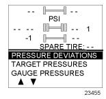
As illustrated, the pressure readings will appear replacing the dash lines as the TPMS display starts to receive pressure data from the TPMS receiver. It can take 1 minute to get all pressure readings updated since the sensors transmit at a one minute interval.
