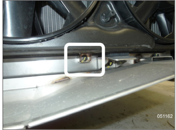
FAN SHROUD TOP & BOTTOM HOLD-DOWN SCREWS
