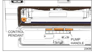
3. Engage either keyed release shaft with the pump handle.
