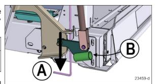
6. Push the backup pump release valve actuating rod back DOWN until lightly-snug.
