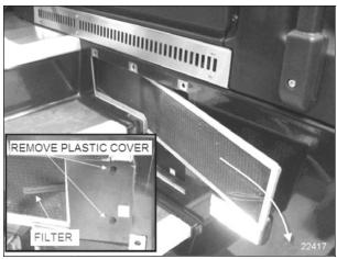
REMOVING DRIVER'S SECTION AIR FILTER
