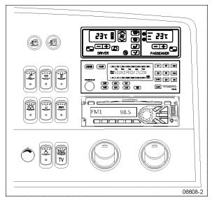
Controls for passenger entertainment are grouped on the R.H. dashboard panel. The HVAC control module as well as the cluster dimmer switch, miscellaneous control switches and air vents are also located on this side of the dashboard.
