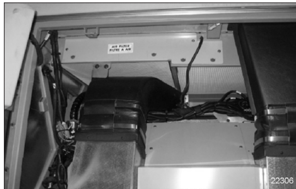
PASSENGERS AREA AIR FILTER REMOVAL
