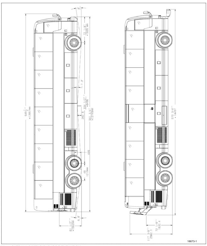
X3-45 OVERALL DIMENSIONS (SIDE ELEVATION)
