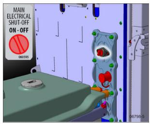
MAIN ELECTRICAL SHUT-OFF SWITCH (X3 SERIES)
