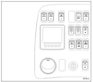
The L.H. dashboard panel includes controls for the operation of the coach; it also includes the ignition switch and an adjustable air register.
