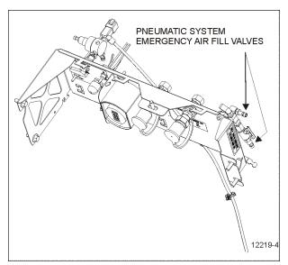
**FILL FITTING IN ENGINE COMPARTMENT**
