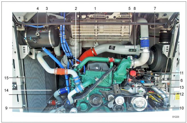
**ENGINE COMPARTMENT FEATURING VOLVO D13 ENGINE**
