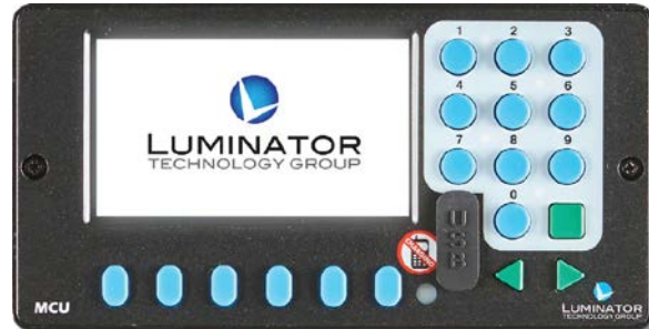
Destination Sign Controller
