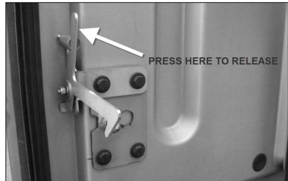
EVAPORATOR COMPARTMENT DOOR SECONDARY LOCK LEVER
