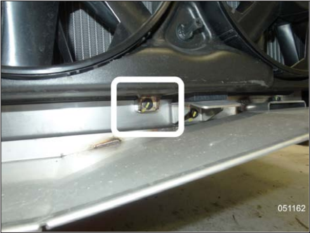
FAN SHROUD TOP & BOTTOM HOLD-DOWN SCREWS
