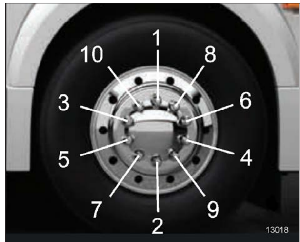
TIGHTENING SEQUENCE
