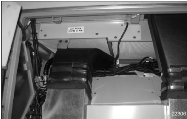
CABIN AREA AIR FILTER REMOVAL
