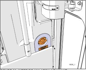
FIGURE 36: INTERIOR UNLATCH AIR VALVE
