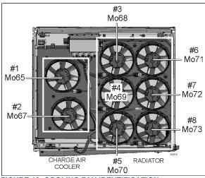
FIGURE 12: COOLING FAN IDENTIFICATION
