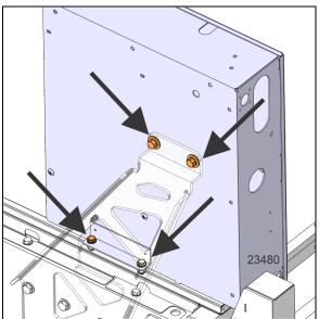
FIGURE 48: CONTROL BOX DISMOUNTING
