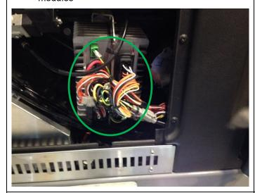
Disconnect the ACM connector (A137A)
