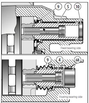
FIGURE 49: CHECKING OF GUIDE PIN AND SEALS
