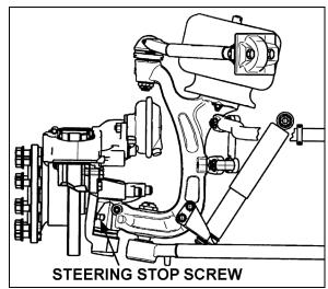
FIGURE 16: STEERING STOP SCREW ON IFS
