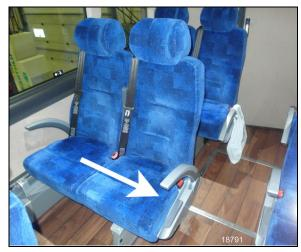
FIGURE 32: PULL TO UNLOCK THE ROTATION
