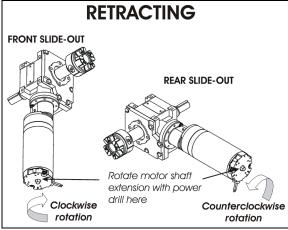
FIGURE 13: SLIDE-OUT MOTOR ROTATION
