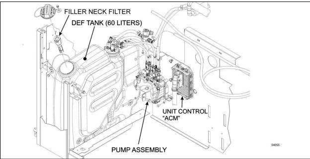
FIGURE 12 X SERIES DEF TANK AND PUMP
