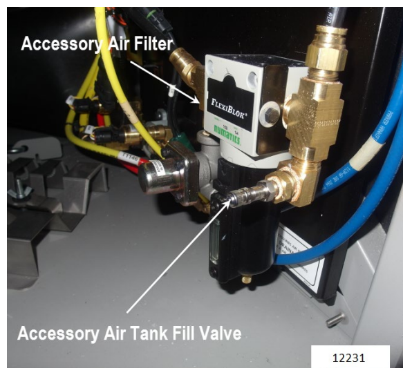
FIGURE 4: FRONT SERVICE COMPARTMENT
