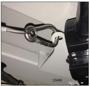
FIGURE 44: PROTECTIVE WIRE INSTALLATION
