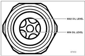
FIGURE 18: SIGHT GLASS FOR CHECKING OIL LEVEL
