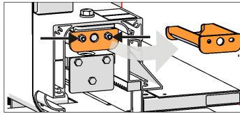
FIGURE 5 EXTENSION STOPPER REMOVAL
