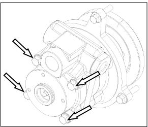
FIGURE 8: POWER STEERING PUMP REMOVAL
