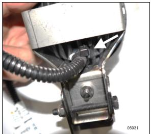
FIGURE 116: FOG LIGHT INSTALLATION
