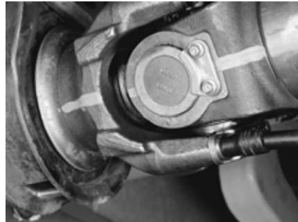
FIGURE 25: ALIGN THE PHASING MARKS BETWEEN THE YOKE AND PROPELLER SHAFT
