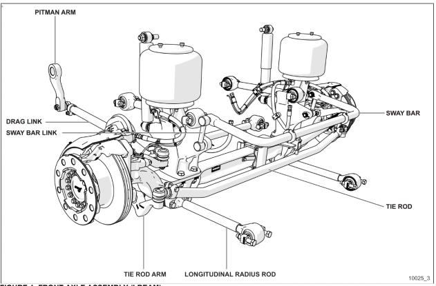
FIGURE 1: FRONT AXLE ASSEMBLY (I-BEAM)
