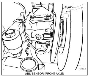
FIGURE 55: ABS SENSOR LOCATION
