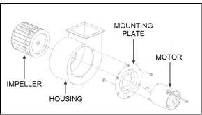
FIGURE 26: FAN ASSEMBLY COMPONENTS
