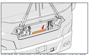
FIGURE 27: DRIVER HVAC SYSTEM FRESH AIR FILTER
