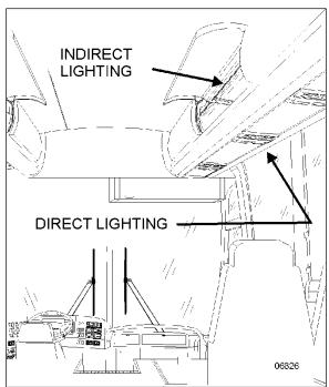
FIGURE 127: OVERHEAD COMPARTMENT LIGHTING
