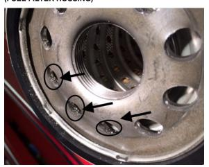
ALUMINUM PARTICLES FOUND ON A PRE-GHG17 FILTER CAUSED BY GRINDING OF THE TOP OF THE FILTER INTO THE FILTER RESTRICTOR
