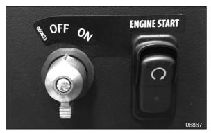
FIGURE 65: SWITCH ARRANGEMENT WITH STARTING MODULE
