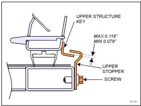
FIGURE 27: UPPER INNER STOPPERS ADJUSTMENT
