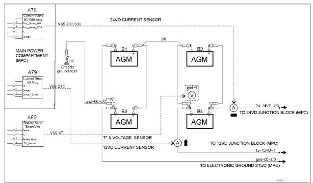
FIGURE 41: BATTERY CONNECTIONS SCHEMATIC - X3 SERIES
