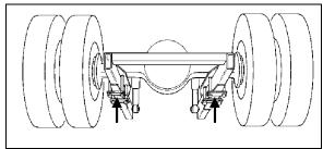
FIGURE 6: JACKING POINTS ON DRIVE AXLE H3B762
