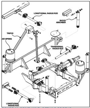
FIGURE 35: DRIVE AXLE, DETAILS OF REAR SUSPENSION
