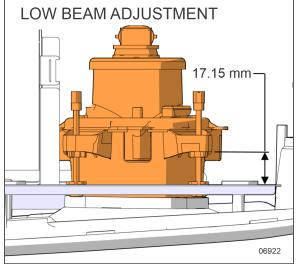
FIGURE 87: LOW BEAM ADJUSTMENT
