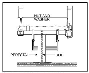
FIGURE 35: SEAT PEDESTAL ASSEMBLY
