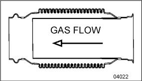
FIGURE 2: FLEXIBLE COUPLING
