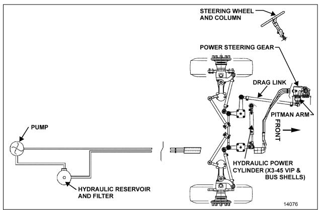
FIGURE 2: IFS STEERING SYSTEM SETUP
