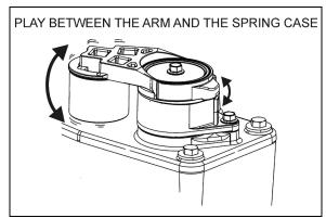
FIGURE 26: CHECKING BUSHING WEAR
