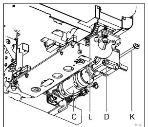
FIGURE 59: EXTENSION MOTOR (FORE SHOWN)
