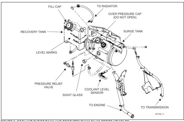
FIGURE 2: COOLANT SURGE TANK AND RECOVERY TANK ON X3 SERIES VEHICLES
