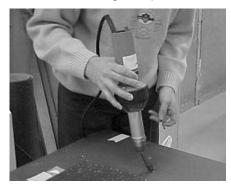
Once the welding torch is ready, insert the filler bead into the nozzle and immediately start welding. Move in a regular manner while pressing slightly with torch.
