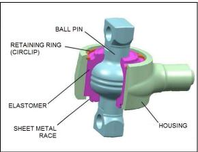
FIGURE 6: BALL PIN JOINT CONSTRUCTION
