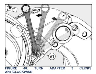
15. As a visual aid, position a ring spanner or socket onto the adjuster (including Adapter (61)) as shown. Apply the brakes 5 to 10 times, the spanner or socket should turn clockwise (viewed from actuator side) in small increments if the adapter is functioning correctly (see Figure 41 and note below).
