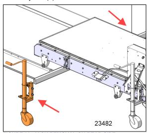
FIGURE 39: JACK REMOVAL ON REAR SIDE
