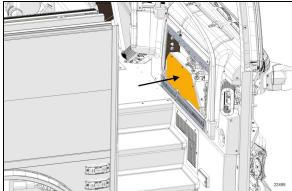
FIGURE 105:REMOVE FRONT A/C COVER TO ACCESS MODULES
