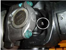
FIGURE 3: BEARING LUBRICATION ZIRK
