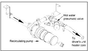
FIGURE 78: HOT WATER CIRCULATING PUMF INSTALLATION (SMALL HVAC SYSTEM) 22292
