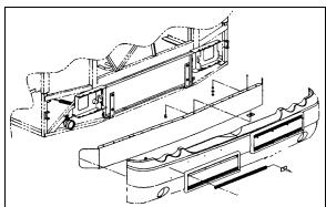
FIGURE 97: FRONT BUMPER REMOVAL
