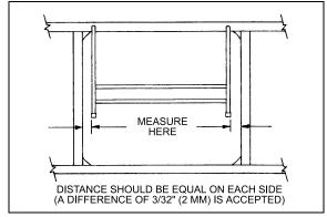
FIGURE 80: PANTOGRAPH DOOR ADJUSTMENT 18063
