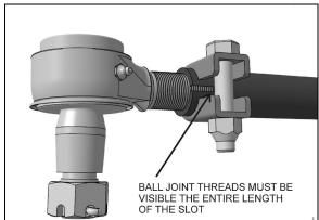
FIGURE 21: ADEQUATE CLAMPING CONDITION
