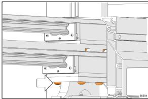
FIGURE 47: LOWER CARRIAGE MOUNTING SCREWS
