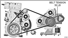
FIGURE 40: BELT LAYOUT WITH SMALL A/C COMPRESSOR H-SERIES
