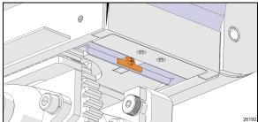
FIGURE 23: TAB AND RETAINING SCREW
