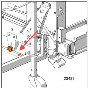
FIGURE 51: SLIDE THE CASSETTE INSIDE THE COMPARTMENT
