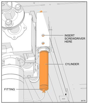
FIGURE 32: SECURITY PIN AIR CYLINDER REMOVAL
