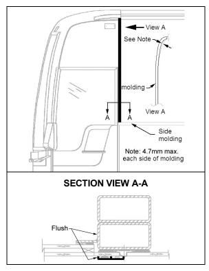
Position and fix horizontal molding (gutter). Lean gutter against vertical molding. Position gutter just above Sika finishing joint.
