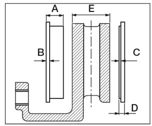
FIGURE 27: BRAKE PADS DIMENSIONS
