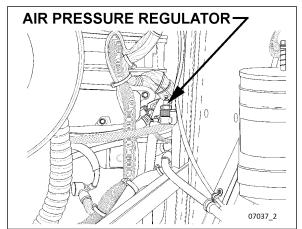
FIGURE 14: AIR PRESSURE REGULATOR (TYPICAL)
