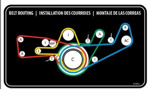
FIGURE 20: VIP BELT ROUTING - SMALL A/C SYSTEM,
