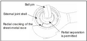
FIGURE 26: BALL PIN BUSHING
