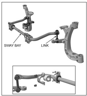
FIGURE 34: SWAY BAR (INDEPENDENT FRONT SUSPENSION)
