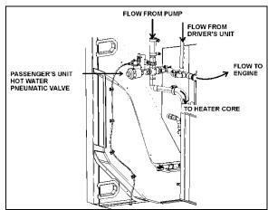
FIGURE 87: PASSENGER UNIT PNEUMATIC HOT WATER VALVE ASSEMBLY 22240
