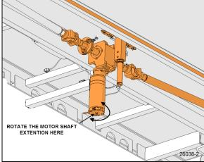
FIGURE 13: SLIDE-OUT MOTOR ROTATION
