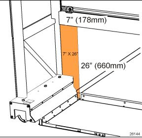
FIGURE 74: "NO DRILLING" ZONE (FORE AND AFT)
