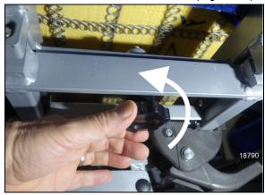
FIGURE 87: LOOSEN THE KNOB
