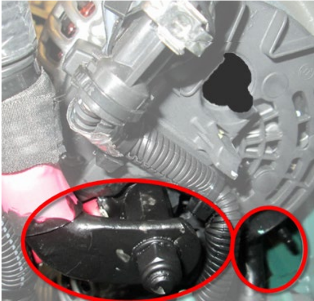
Figure 27: Upper R.H. side Bosch alternator power cable lug protected with Color Guard rubber coating.
