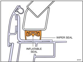
FIGURE 31: INFLATABLE SEAL ASSEMBLY
