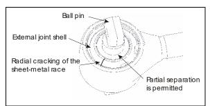
FIGURE 7: BALL PIN BUSHING
