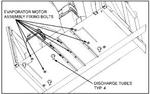
FIGURE 56: EVAPORATOR MOTOR BOLTS
