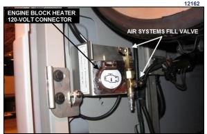
FIGURE 45: REAR VALVE LOCATION ON X3 SERIES
