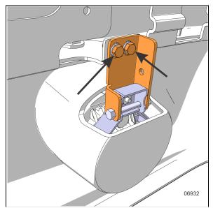
FIGURE 117: FOG LIGHT MOUNTING BOLT
