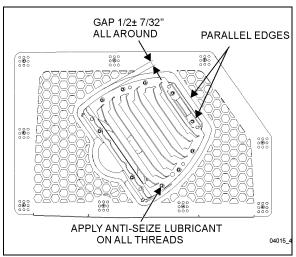
FIGURE 8: DIFFUSER POSITION ADJUSTMENT
