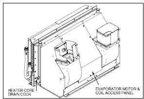
FIGURE 30: PASSENGER UNIT EVAPORATOR COIL
