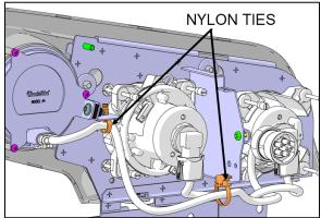
FIGURE 75: TYPICAL CABLE ROUTING WITH TWO HALOGEN HEADLAMPS
