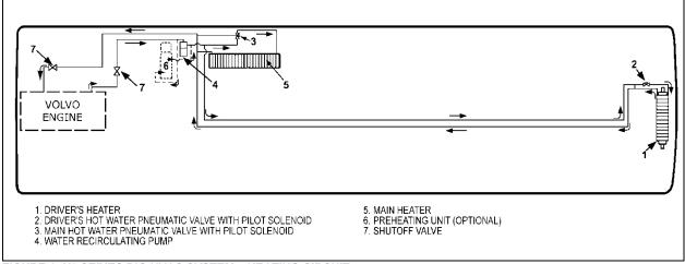
FIGURE 6: X3 SERIES BIG HVAC SYSTEM - HEATING CIRCUIT
