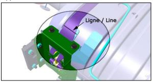
Mark, with a vertical line the central position of the lower and upper clamps with regard to the emboss located at the bottom and at the top of the catalytic converter.
