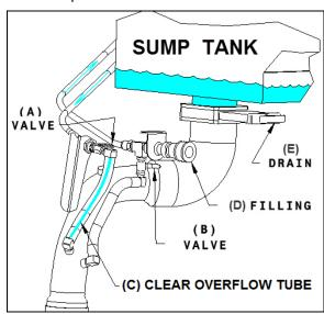
FIGURE 29: SUMP TANK SERVICE VALVES
