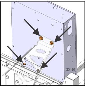
FIGURE 63: CONTROL BOX DISMOUNTING
