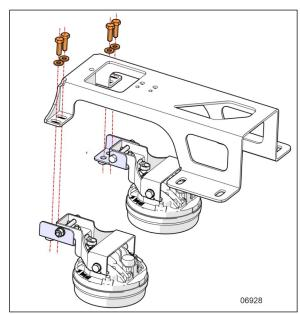
FIGURE 113: FOG LIGHT SUBASSEMBLY DISMOUNT
