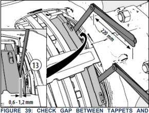
FIGURE 39: CHECK GAP BETWEEN TAPPETS AND INBOARD PAD
