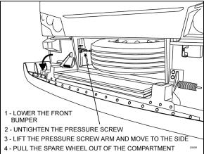
FIGURE 44: H3 SERIES SPARE WHEEL AND TIRE
