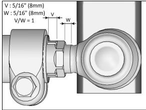
FIGURE 24: DRAG LINK ADJUSTMENT SYSTEM
