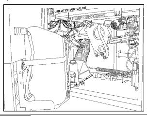
FIGURE 35: EXTERIOR UNLATCH AIR VALVE 12209
