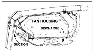
FIGURE 84: OVERHEAD COMPARTMENT VENTILATION SYSTEM 22211
