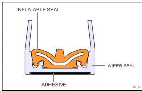
FIGURE 8: TWO-PART SEAL ASSEMBLY
