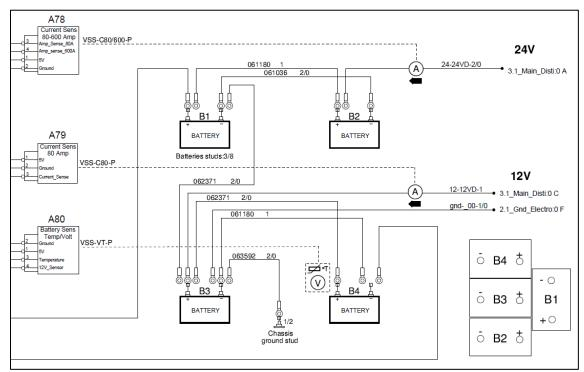
FIGURE 43: BATTERY CONNECTIONS SCHEMATIC - H3 SERIES
