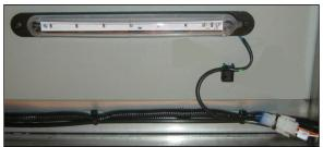
FIGURE 120: BAGGAGE COMPARTMENT LIGHTS LED SEALED UNIT
