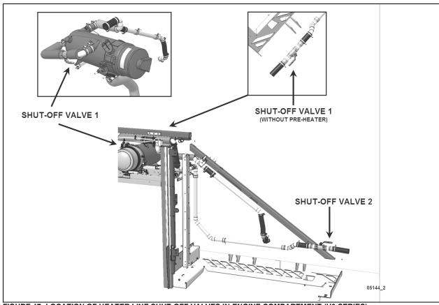
FIGURE 17: LOCATION OF HEATER LINE SHUT-OFF VALVES IN ENGINE COMPARTMENT (H3 SERIES)
