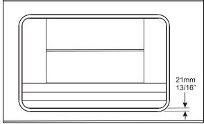
FIGURE 5: SLIDE-OUT LEVEL ADJUSTMENT
