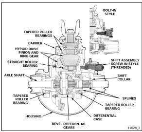
FIGURE 3: DRIVER-CONTROLLED DIFFERENTIAL LOCK
