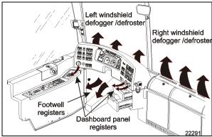
FIGURE 102: DRIVER UNIT AIR CIRCULATION
