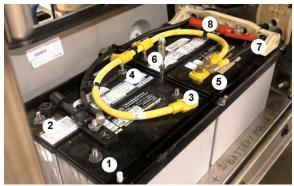
FIGURE 49: DISCONNECT 8 CABLE TERMINALS
