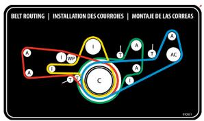
FIGURE 21: VIP BELT ROUTING - SMALL A/C SYSTEM, 5 ALTERNATORS
