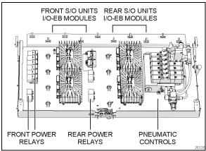
FIGURE 50: SLIDE-OUT CONTROL PANEL
