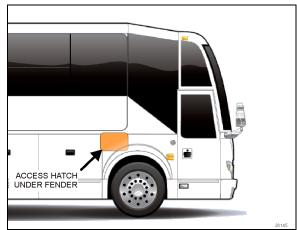
FIGURE 66: ACCESS TO LEVELING SCREWS, FORE
