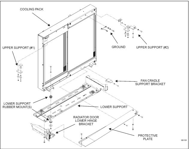
FIGURE 48: COOLING PACK SUPPORTS AND COMPONENTS
