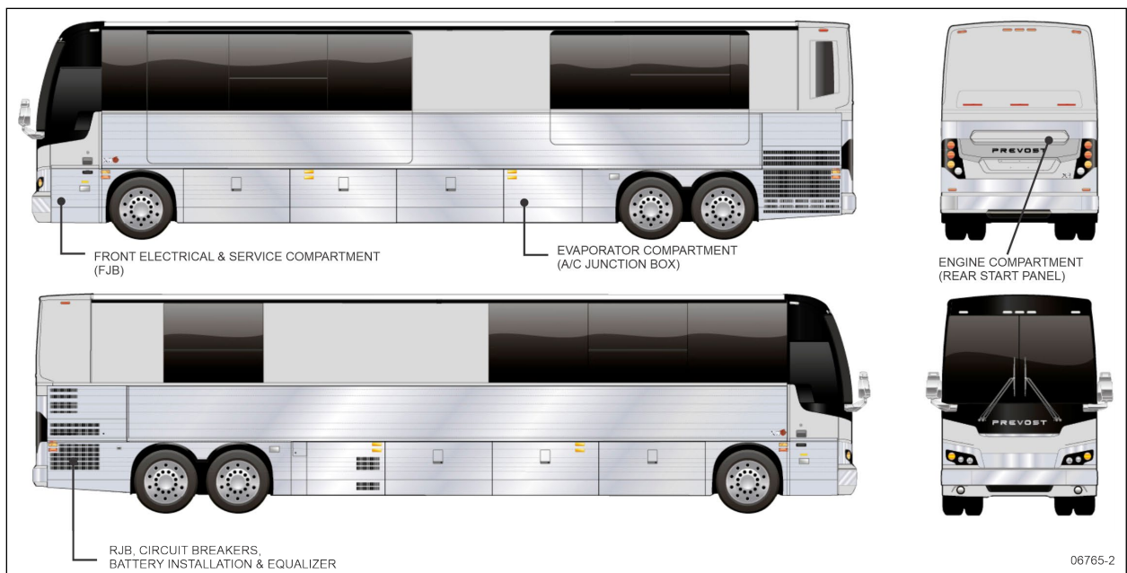
FIGURE 19: ELECTRICAL COMPARTMENTS (X3-45 VIP)
