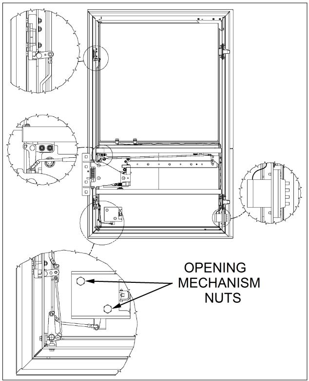
FIGURE 76: WCL SLIDING DOOR OPENING MECHANISM
