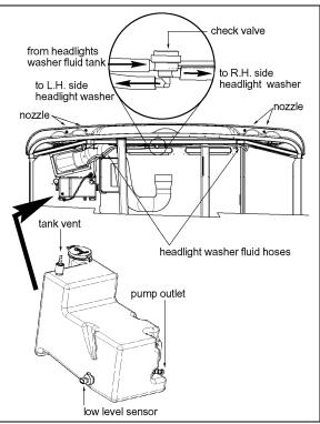
FIGURE 32: HEADLIGHTS CLEANING SYSTEM
