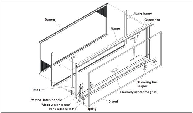
FIGURE 104: ELECTRIC AWNING WINDOW EXPLODED VIEW (FRAME) 18586
