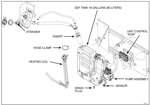
FIGURE 11: H SERIES DEF TANK AND PUMP
