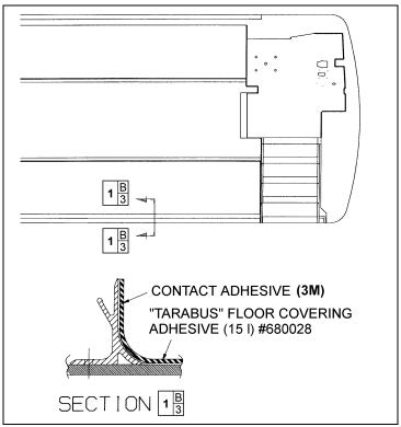
FIGURE 29: TARABUS FLOOR COVERING ADHESIVE APPLICATION
