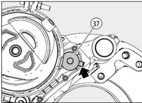
FIGURE 42: TAB POSITIONING OF THE CAP
