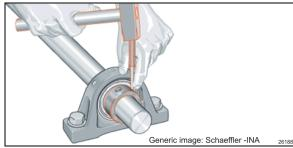
FIGURE 44: ECCENTRIC COLLAR TENSION APPLICATION
