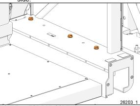
FIGURE 45: TOP RAIL SCREWS
