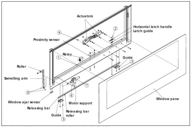
FIGURE 45: ELECTRIC AWNING WINDOW EXPLODED VIEW (SASH) 18583
