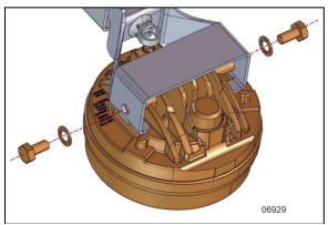
FIGURE 114: FOG LIGHT REMOVAL
