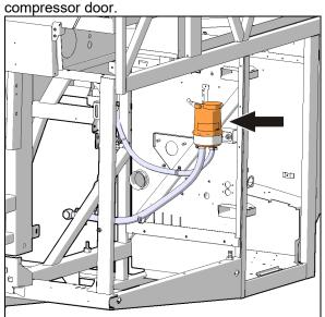
FIGURE 25: H SERIES POWER STEERING RESERVOIR
