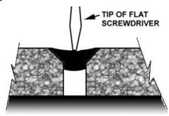
13. If welding was not performed properly, there will be a loss of adhesion on one side. If this is the case, repair the joint.
