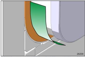
FIGURE 20: PLASTIC SHEET -WIPER SEAL PROTECTION
