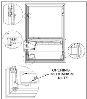
FIGURE 79: WCL SLIDING DOOR OPENING MECHANISM 18740
