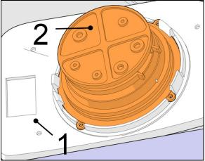
FIGURE 104: (1) CONVEX GLASS MIRROR; (2) MOTOR
