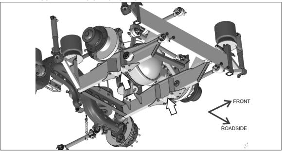
FIGURE 11: DRIVE AXLE SUB FRAME HOISTING POINTS.
