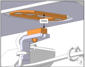
FIGURE 53: SENSOR VERTICAL ADJUSTMENT
