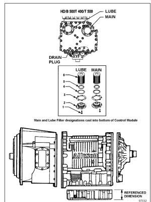
FIGURE 7: DRAIN PLUG AND FILTERS
