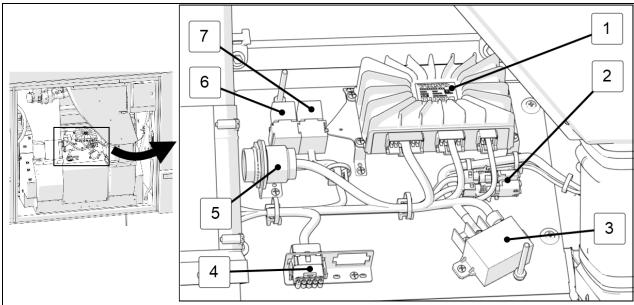
FIGURE 34: EVAPORATOR COMPARTMENT CONTROL PANEL
