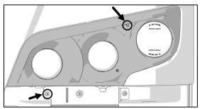
FIGURE 77: HEADLAMPS ASSEMBLY FIXING SCREWS
