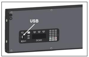
FIGURE 19: DESTINATION SIGN LCD DISPLAY (SERIES 600 SHOWN) 23123-1
