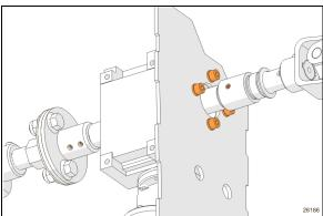
FIGURE 42: DRIVE MOTOR/GEARBOX ASSEMBLY MOUNTING BOLTS
