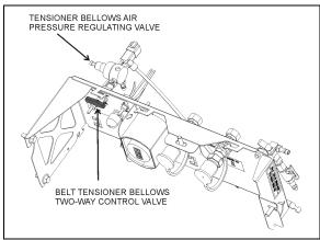
FIGURE 39: BELT TENSIONER CONTROL VALVE - H3
