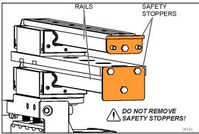
FIGURE 11: SAFETY STOPPERS ON RAILS
