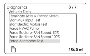
To initiate the test, use the Driver Information Display (DID) DIAGNOSTICS menu. Select VEHICLE TESTS submenu and then FORCE ALTERNATORS TEST. Press ENTER button to start the test. This feature will activate one alternator at a time during 5 seconds, cycling between alternator 1, 2 & 3.
