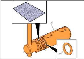
FIGURE 8: INSPECT THE O-RING (4) IN THE SPINDLE (2)
