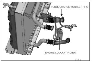
FIGURE 19: COOLANT FILTER (X3 SERIES SHOWN)
