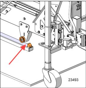
FIGURE 40: SLIDE THE CASSETTE INSIDE THE COMPARTMENT
