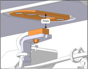
FIGURE 52: SENSOR VERTICAL ADJUSTMENT
