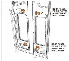
FIGURE 38: DOOR PANEL ADJUSTMENTS
