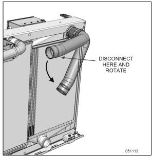
FIGURE 58: ROTATE CAC UPPER PIPE (X3 SERIES ONLY)
