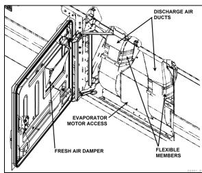
FIGURE 55: X3 SERIES EVAPORATOR COMPARTMENT
