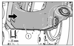
FIGURE 47: FREE MOVEMENT OF CALIPER > 0.984 IN / 25 MM
