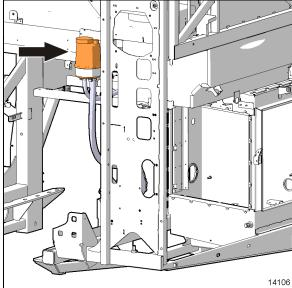
Figure 26: X SERIES POWER STEERING RESERVOIR
