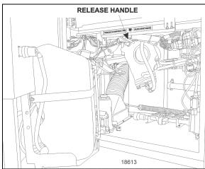
FIGURE 12: FRONT BUMPER RELEASE HANDLE 18613
