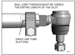
FIGURE 40: ADEQUATE CLAMPING CONDITION
