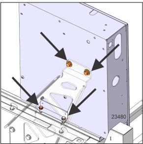
FIGURE 54: CONTROL BOX DISMOUNTING
