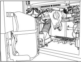
FIGURE 4: FRONT SERVICE COMPARTMENT
