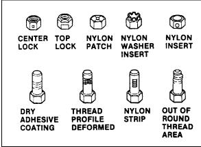
FIGURE 13: SELF-LOCKING FASTENERS
