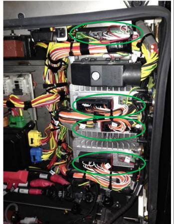
6 Disconnect the control connector from the battery equalizer
