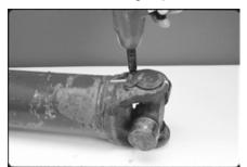
FIGURE 15: SPRING TAB BOLTS REMOVAL
