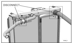
FIGURE 30: RADIATOR & CAC UPPER CONNECTION
