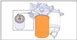
FIGURE 5: SECONDARY FUEL FILTER
