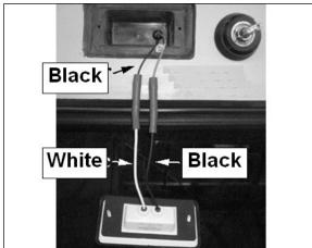
FIGURE 110: LED SEALED UNIT WIRE CONNECTION
