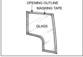
FIGURE 42: ADHESIVE-MOUNTED WINDOW
