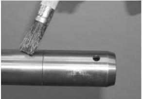
FIGURE 19: APPLY GLEITMO 805 GREASE
