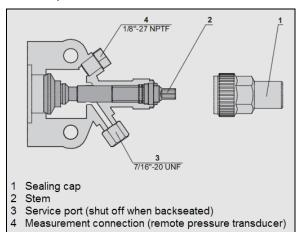
FIGURE 96: COMPRESSOR SHUT-OFF VALVE IN FRONT SEATED POSITION
