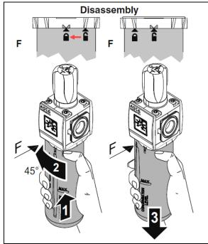
FIGURE 8: ACCESSORY AIR FILTER BOWL REMOVAL
