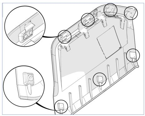
FIGURE 9: ATTACHMENT POINTS AT THE BACK OF THE PANEL
