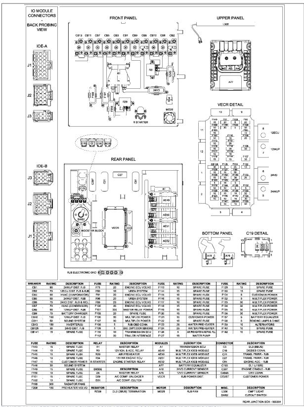
FIGURE 26: X3 SERIES MAIN POWER COMPARTMENT COMPONENTS IDENTIFICATION
