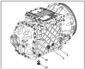
FIGURE 17: I-SHIFT TRANSMISSION OIL CHANGE
