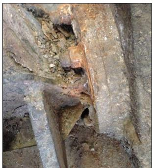
FIGURE 4: METAL FLAKING ON TAG AXLE - ACCUMULATED MATTER WILL RETAIN WATER THUS CREATING CONDITIONS PROMOTING ADDITIONAL CORROSION
