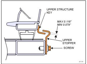
FIGURE 64: UPPER INNER STOPPERS ADJUSTMENT
