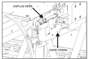
FIGURE 73: MOBILE FLOOR HAND CRANK HEX SOCKET LOCATION
