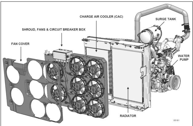
FIGURE 1: COOLING ASSEMBLY & RELATED COMPONENTS (X3 SERIES SHOWN)
