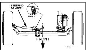
FIGURE 30: STEERING STABILIZER (DAMPER)
