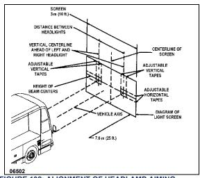
FIGURE 102: ALIGNMENT OF HEADLAMP AIMING SCREEN
