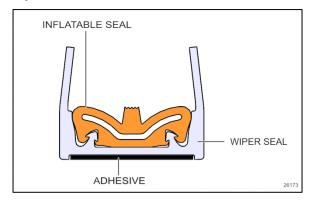
FIGURE 1: TWO-PART SLIDE-OUT SEAL
