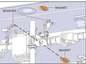
FIGURE 50: SENSORS & MAGNETS (FRONT S/C SHOWN)
