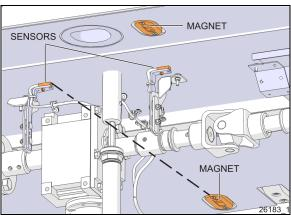
FIGURE 51: SENSORS & MAGNETS (FRONT S/C SHOWN)
