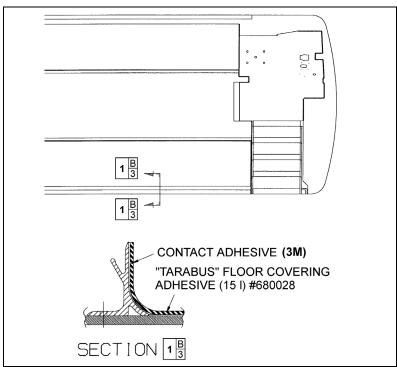
FIGURE 92: TARABUS FLOOR COVERING ADHESIVE APPLICATION
