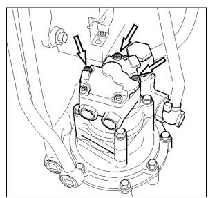
FIGURE 6: FUEL PUMP REMOVAL
