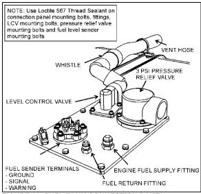
FIGURE 20: FUEL TANK CONNECTION PANEL
