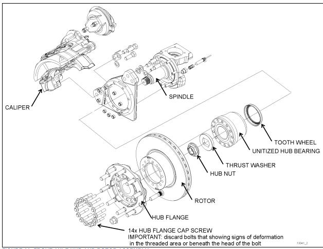
FIGURE 36: FRONT AXLE HUB AND ROTOR ASSEMBLY
