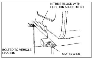
FIGURE 21: FUEL TANK SUPPORT MOUNTING BOLTS
