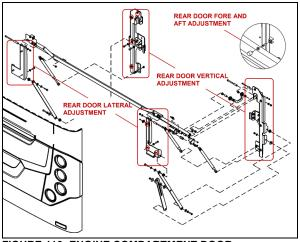
FIGURE 113: ENGINE COMPARTMENT DOOR
