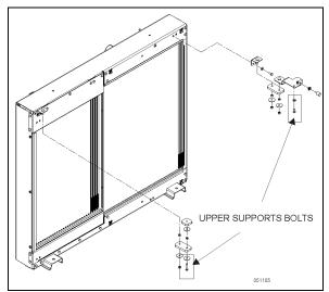
FIGURE 52: UPPER SUPPORTS MOUNTING BOLTS
