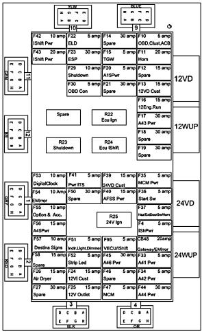
FIGURE 33: VECF - FUSE IDENTIFICATION
