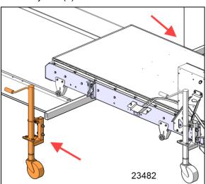
FIGURE 50: JACKS REMOVAL ON REAR SIDE Install the fasteners on the dismounted jacks.
