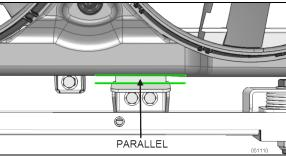
FIGURE 56: FAN SHROUD PARALLEL TO SUPPORT
