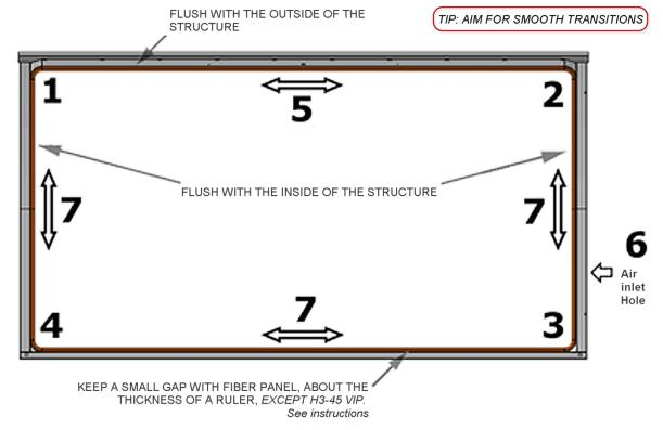
FIGURE 7: SEAL INSTALLATION POSITION AND SEQUENCE OVERVIEW
