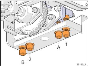
FIGURE 4: LEVELING & TILTING SCREWS
