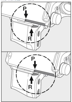
FIGURE 35: PAD WEAR CHECK FRONT AND TAG AXLE
