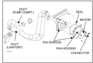
FIGURE 25: VENTILATION FAN INSTALLATION
