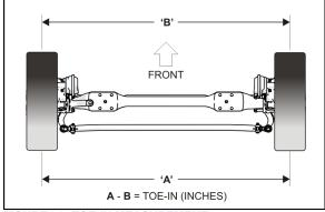
FIGURE 48: TOE-IN MEASUREMENT
