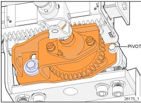
FIGURE 34: PINION ASSEMBLY
