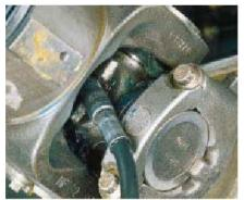
FIGURE 4: BEARING LUBRICATION
