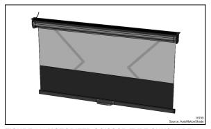
FIGURE 23: MOTORIZED SCISSOR TYPE SUNSHADE
