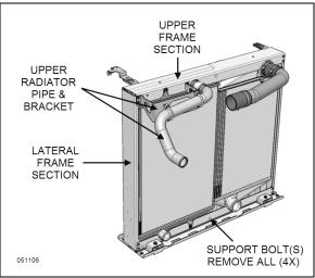
FIGURE 53: COOLING PACK PARTS TO BE REMOVED FOR RADIATOR REPLACEMENT
