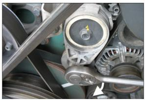
FIGURE 69: 1/2" SOCKET DRIVE WRENCH
