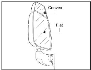
FIGURE 99: REAR VIEW MIRROR (RAMCO)
