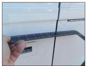
FIGURE 66: USE A RULER (SHOWN IN BLACK) TO CHECK THAT SURFACES ARE EVEN
