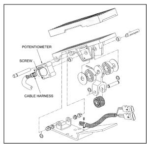
FIGURE 18: ELECTRONIC FOOT PEDAL ASSEMBLY 3035
