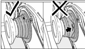
FIGURE 51: CHECK RUBBER BOOTS FOR DAMAGE
