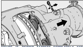
FIGURE 45: REWIND TAPPETS COMPLETELY AND PUSH CALIPER IN DIRECTION OF MIDDLE OF VIEW
