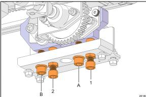
FIGURE 4: LEVELING & TILTING SCREWS
