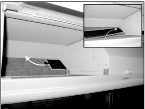
FIGURE 34: OVERHEAD COMPARTMENT FAN AIR FILTER (X3 SERIES) 22201
