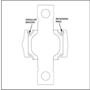
FIGURE 27: LOWER A-ARM BALL PIN BUSHING 16047
