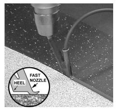
9. Allow cooling down of filler bead (about 5 minutes).
