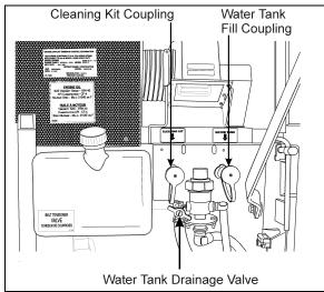
FIGURE 27: FRESH WATER TANK SERVICE VALVES
