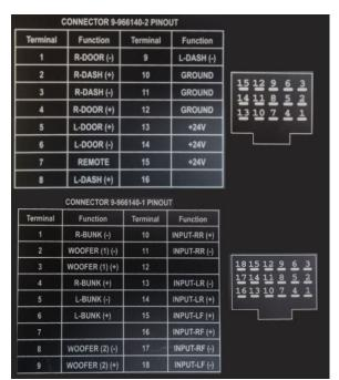
FIGURE 9: AMPLIFIER CONNECTORS PINOUT
