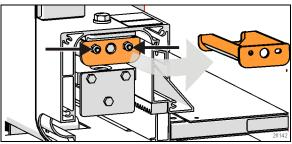
FIGURE 10 EXTENSION STOPPER REMOVAL
