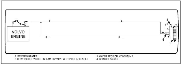
FIGURE 10: X3 SERIES SMALL HVAC SYSTEM - HEATING CIRCUIT
