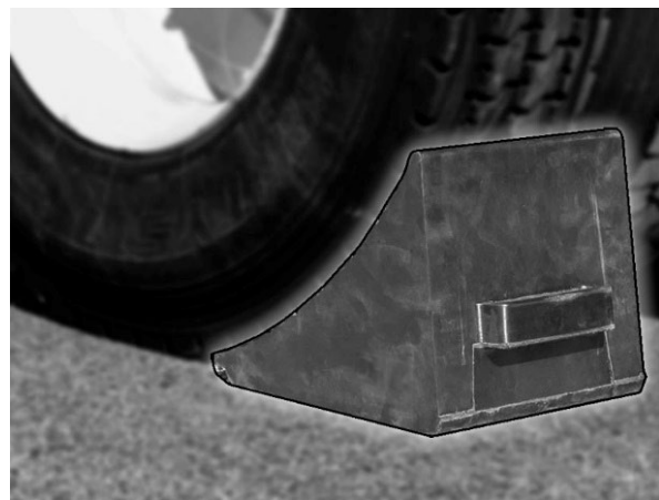
FIGURE 21 CHOCK THE FRONT AND REAR WHEELS
