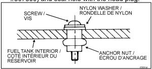
FIGURE 17: FUEL TANK REPAIR
