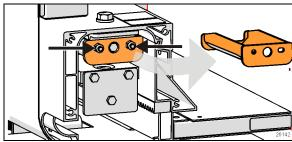
FIGURE 10 EXTENSION STOPPER REMOVAL
