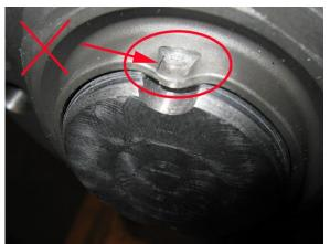
FIGURE 26: BROCKEN OR TORN LIP - REJECTED
