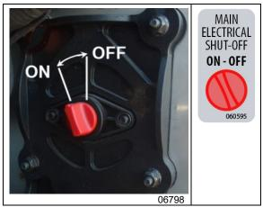
FIGURE 45: X3 SERIES MAIN ELECTRICAL SHUT-OFF SWITCH
