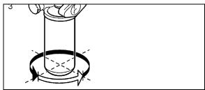
FIGURE 11: OIL FILTER REPLACEMENT
