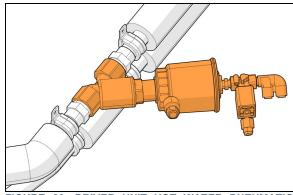
FIGURE 86: DRIVER UNIT HOT WATER PNEUMATIC VALVE ASSEMBLY
