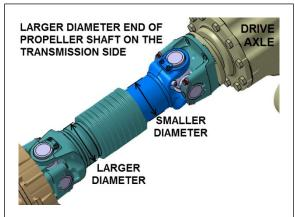
FIGURE 11: PROPELLER SHAFT PROPER ORIENTATION
