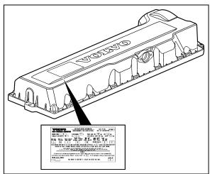
FIGURE 1: VOLVO D13 ENGINE DATA PLATE
