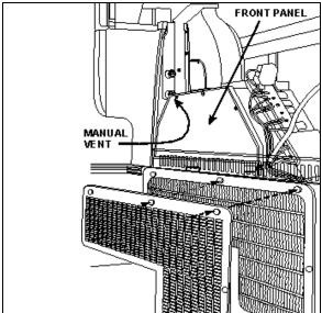
FIGURE 88: DRIVER'S HVAC/DEFROST UNIT
