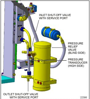
FIGURE 62: RECEIVER TANK (H3 SERIES)
