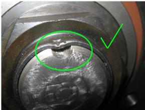
FIGURE 24: CORRECT - PREVENTS THE NUT FROM GETTING LOOSE
