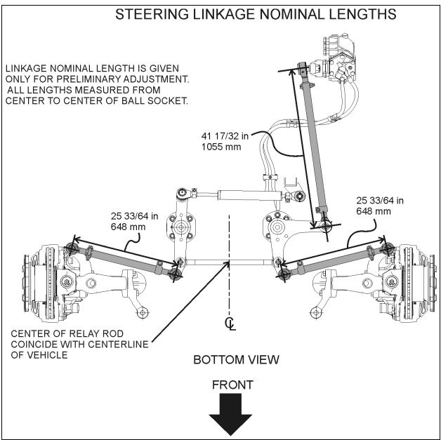
FIGURE 19: STEERING LINKAGE NOMINAL LENGTHS
