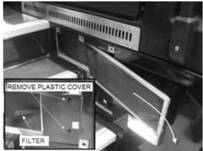
FIGURE 26: REMOVING DRIVER'S SECTION AIR FILTERS
