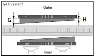
FIGURE 29: EXAGGERATED TANGENTIAL OBLIQUE WEAR OF BRAKE PADS
