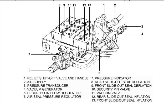
FIGURE 49: PNEUMATIC COMPONENT PANEL
