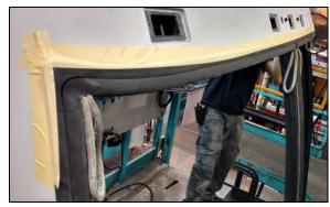
FIGURE 63: MASKING TAPE APPLICATION
