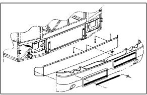
FIGURE 14: FRONT BUMPER REMOVAL
