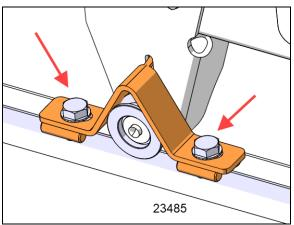
FIGURE 53: ANCHOR BOLTS INSTALLATION
