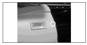
Apply a double-face self adhesive tape 1/8 by ¼ inch inside the molding onto the whole length.
