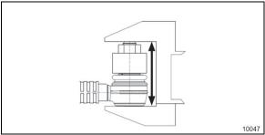
FIGURE 36: MEASURING AXIAL PLAY, TIE ROD JOINTS
