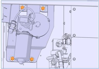
Figure 5: CURB SIDE DRIVE MOTOR
