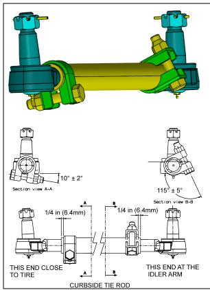
FIGURE 17: CURBSIDE TIE ROD - CLAMPS POSITION
