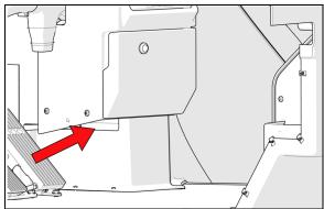
FIGURE 28: ACCESS TO THE RECIRCULATING AIR FILTERS
