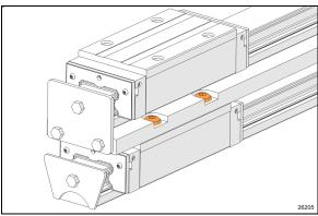
FIGURE 48: BEARING CARRIAGE MOUNTING SCREWS
