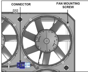
FIGURE 23: CONNECTOR & MOUNTING SCREW LOCATION
