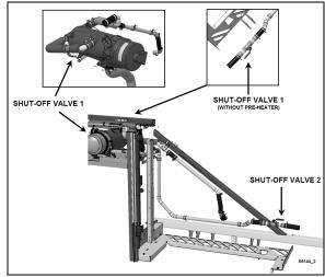
FIGURE 28: HEATER SHUT-OFF VALVES POSITION
