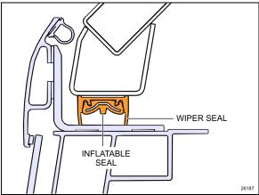
FIGURE 31: INFLATABLE SEAL ASSEMBLY
