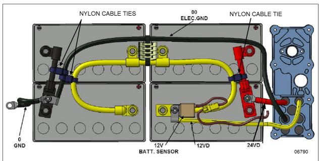
FIGURE 42: AGM BATTERY CONNECTIONS - X3 SERIES
