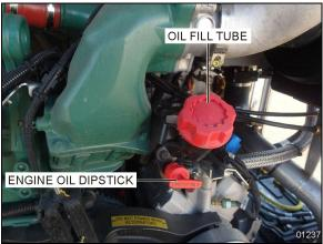
FIGURE 12: TYPICAL ENGINE OIL FILLING TUBE
