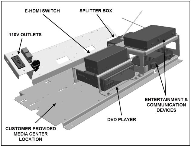
FIGURE 1: AUDIO-VIDEO PANEL IN OVERHEAD COMPARTMENT
