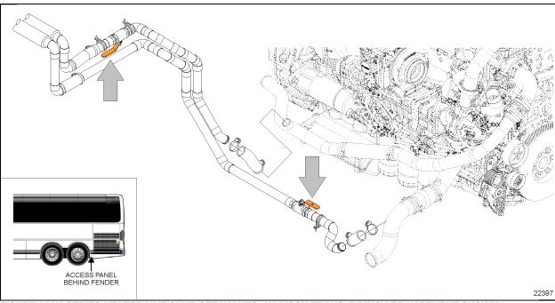
FIGURE 92 X3 SERIES HEATER LINE SHUT-OFF VALVES- (ALLISON TRANS. PIPING ARRANGEMENT SHOWN)
