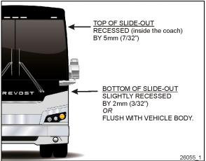
FIGURE 6: TILT ADJUSTMENT VALUES
