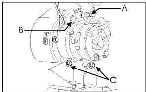
FIGURE 52: COMPRESSOR MOUNTING H-SERIES
