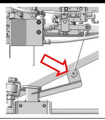
5. Loosen the lower mounting bolt shown.
