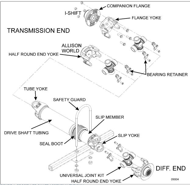
FIGURE 1: PROPELLER SHAFT ASSEMBLY (TYPICAL)
