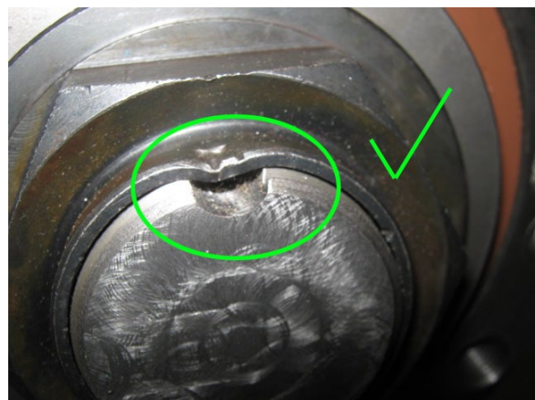
FIGURE 24: CORRECT - PREVENTS THE NUT FROM GETTING LOOSE
