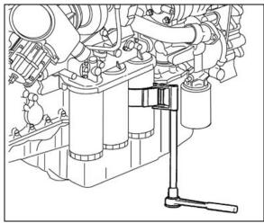
FIGURE 10: OIL FILTER WRENCH
