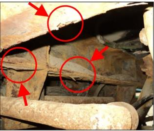
FIGURE 3: METAL FLAKING AND ACCUMULATED SAND
