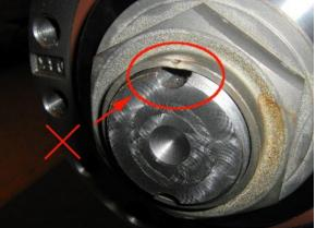
FIGURE 27: LIP INADEQUATELY PRESSED IN - REJECTED
