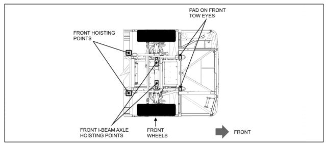
FIGURE 13: OPTIONAL FRONT CHASSIS HOISTING POINTS
