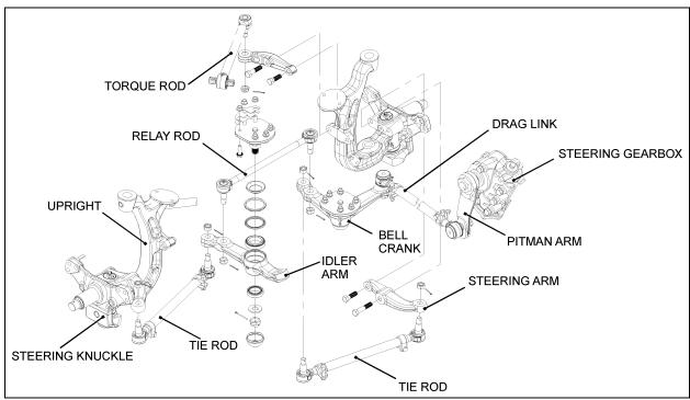
FIGURE 10: IFS STEERING LINKAGE OVERVIEW
