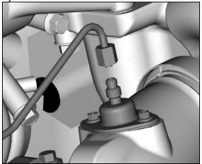
FIGURE 14: AFTERTREATMENT HYDROCARBON DOSER
