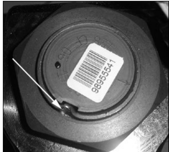
FIGURE 20: FIXING NUT PUNCH MARK
