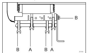
FIGURE 65: TILT AND LEVELING SCREWS
