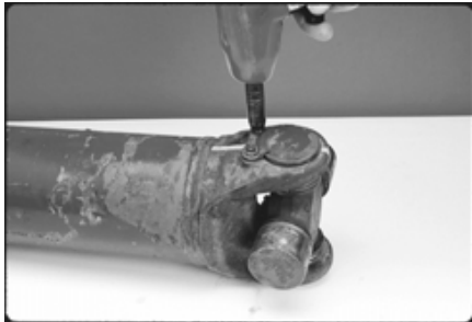
FIGURE 15: SPRING TAB BOLTS REMOVAL
