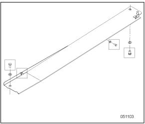
FIGURE 34: PROTECTIVE PLATE MOUNTING BOLTS
