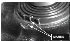
FIGURE 11: STEERING GEARBOX INPUT SHAFT MARKS
