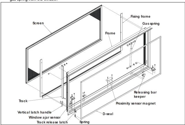
FIGURE 44: ELECTRIC AWNING WINDOW EXPLODED VIEW (FRAME)
