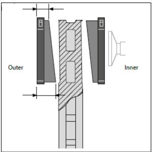
FIGURE 30: BRAKE PAD WITH EXAGGERATED TAPER WEAR
