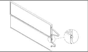
FIGURE 32: PASSENGER UNIT 2-PART AIR FILTER H3 SERIES
