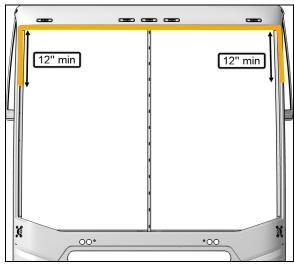
FIGURE 64: MASKING TAPE APPLICATION
