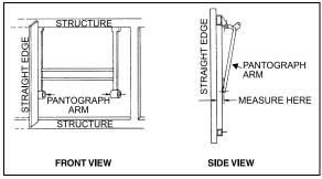
FIGURE 79: PANTOGRAPH DOOR ADJUSTMENT 1806
