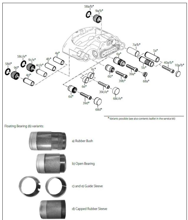
FIGURE 24: IDENTIFICATION OF GUIDE & SEAL VARIANTS
