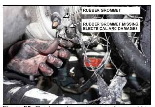
Figure 25: Fire in engine compartment caused by rubbing of power cable against metal edge of Bosch T1 alternator rear cover. Lower rubber grommet was missing when fire occured. Evidence of electrical arc can be seen.
