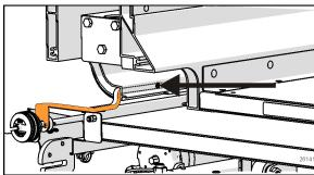
FIGURE 69: POSITION RING PUSH-PULL TAE REMOVAL.
