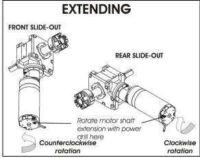
FIGURE 15: SLIDE-OUT MOTOR ROTATION
