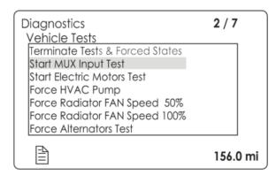
To initiate the test, use the Driver Information Display (DID) DIAGNOSTICS menu. Select VEHICLE TESTS submenu and then START MUX INPUT TEST. Press ENTER button to start the test. The DID status line will show TEST to confirm the test mode is active. To exit test, press ESCAPE button, select TERMINATE TESTS & FORCED STATES submenu and then press ENTER button twice. TEST will disappear from the DID status line.
