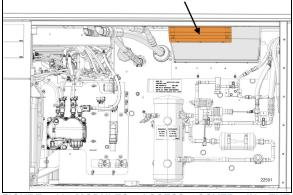
FIGURE 107:MODULES ACCESS COVER IN THE CONDENSER COMPARTMENT
