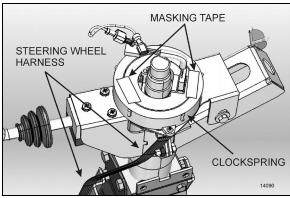
FIGURE 13: LOCKING THE CLOCKSPRING IN PLACE
