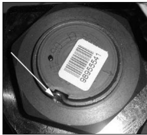
FIGURE 20: FIXING NUT PUNCH MARK
