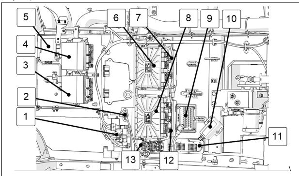
FIGURE 38: DASHBOARD CONTROL PANEL - H3 SERIES SHOWN
