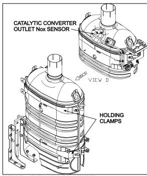
FIGURE 6: CATALYTIC CONVERTER
