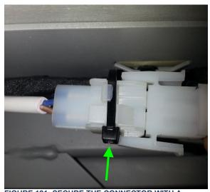
FIGURE 121: SECURE THE CONNECTOR WITH A NYLON TIE
