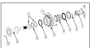
FIGURE 41: ZF A-132 DRIVE AXLE HUB ASSEMBLY
