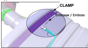
Using the lines made earlier, line up the lower and upper clamps with regard to the emboss of the converter and afterward, line up the lines made earlier on the clamps with regard to the clamp supports on the catalytic converter.
