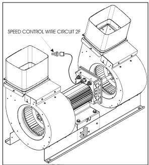
FIGURE 57: EVAPORATOR MOTOR ASSEMBLY
