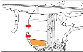
FIGURE 22: DRIVER UNIT CORE ACCESS - H3 SERIES
