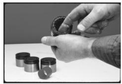
FIGURE 27: GREASING BEARING CUP
