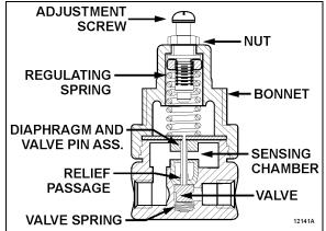
FIGURE 15: AIR PRESSURE REGULATING VALVE
