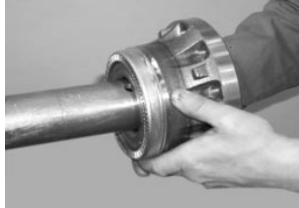
FIGURE 20: SLIP UNITIZED HUB BEARING OVER SPINDLE
