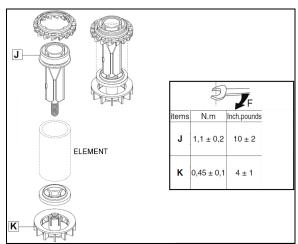
FIGURE 10: ACCESSORY AIR FILTER ARRANGEMENT
