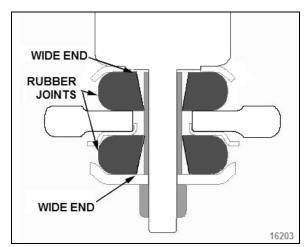
FIGURE 33: LOWER SHOCK MOUNTING BUSHINGS
