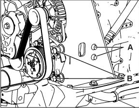
FIGURE 53: COMPRESSOR MOUNTING X-SERIES
