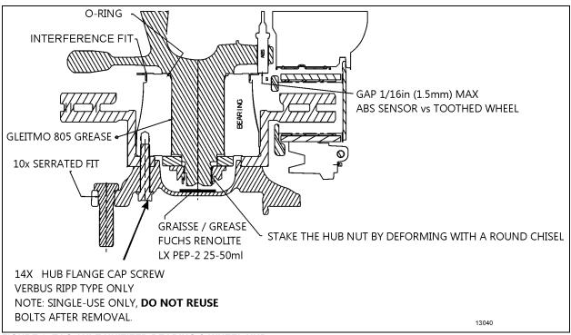
FIGURE 8: TAG AXLE UNITIZED BEARING & WHEEL HUB
