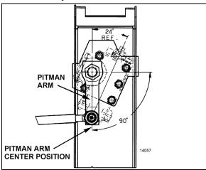
FIGURE 19: IFS PITMAN ARM ADJUSTMENT
