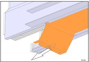
FIGURE 24: PULLING THE FLEXIBLE COVER OUT.
