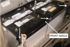
FIGURE 51: REMOVE THE FRONT ANGLE
