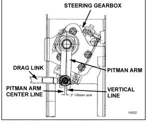
FIGURE 5: PITMAN ARM ADJUSTMENT
