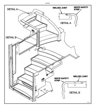
5. Apply contact adhesive (3M) (684655 or 684654) onto both surfaces to glue (fiberglass and back of white safety strip). Drying time: 4 to 5 minutes.
