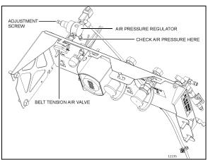
FIGURE 16: AIR PRESSURE REGULATOR (H-SERIES)
