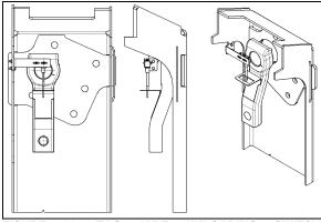
FIGURE 21: TAG AXLE UNLOADING SWITCH ADJUSTMENT
