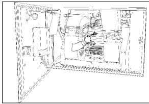
FIGURE 23: EVAPORATOR COIL CLEANING WITH LOW-PRESSURE AIR JET 22373
