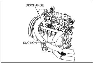
FIGURE 42: SUCTION AND DISCHARGE HOSE
