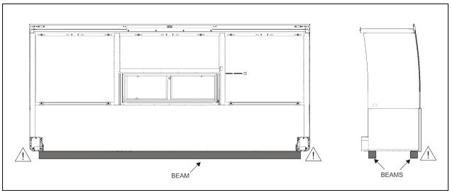
FIGURE 1: BEAM PLACEMENT
