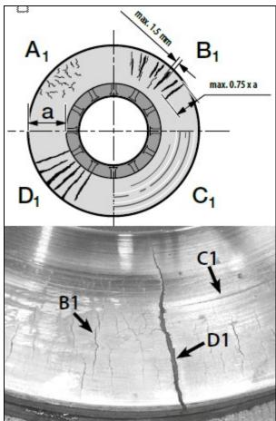
FIGURE 32: TOLERANCES AND EXAMPLES OF CRACKS AND GROOVES
