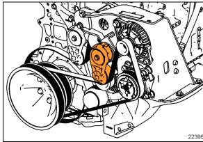
FIGURE 41: BELT LAYOUT WITH SMALL A/C COMPRESSOR X-SERIES
