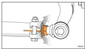
FIGURE 49: FINE ADJUSTER SLEEVE ON TIE ROD
