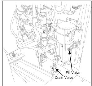
FIGURE 46: FRONT VALVE LOCATION ON H3 SERIES
