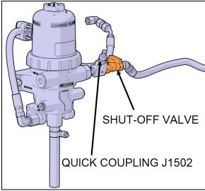
FIGURE 7: DAVCO FUEL PRO 386 WITH MANUAL SHUT-OFF VALVE
