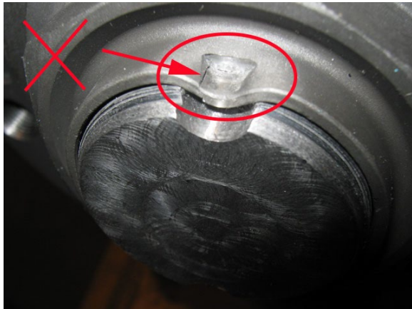
FIGURE 26: BROCKEN OR TORN LIP – REJECTED
