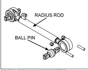
FIGURE 5: TYPICAL RADIUS ROD SETUP
