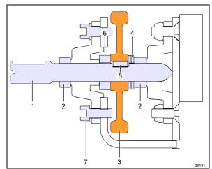
FIGURE 40: PINION ASSEMBLY SECTION VIEW.
