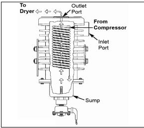
FIGURE 14: HALDEX CONSEP CONDENSER SEPARATOR
