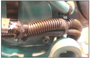
Figure 13: starter cables in a corrugated protective sheath.
