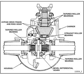
FIGURE 2: DIFFERENTIAL ASSEMBLY
