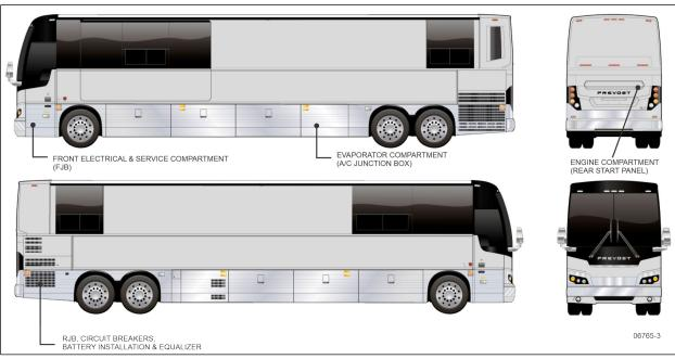
FIGURE 20: ELECTRICAL COMPARTMENTS (X3-45 VIP COMMERCIAL BUS SHELL)
