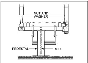
FIGURE 91: SEAT PEDESTAL ASSEMBLY
