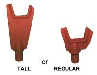
5. Deploy the tow truck stinger arm. Place the axle forks under the rear tow eyes if equipped or under the side members (Figure 60).
