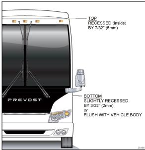
FIGURE 6: TILT ADJUSTMENT VALUES
