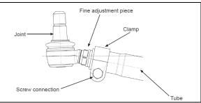
FIGURE 34:TIE ROD COMPONENTS
