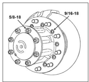
FIGURE 9: FASTENER SIZE IDENTIFICATION
