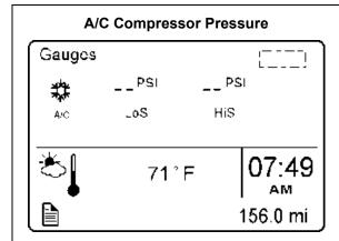
Displays the A/C system's suction pressure value (LoS=low side) and discharge pressure value (HiS=high side).
