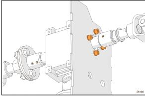
FIGURE 41: DRIVE MOTOR/GEARBOX ASSEMBLY MOUNTING BOLTS
