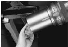
FIGURE 22: CLEAN GREASE FROM SPLINE SLEEVE
