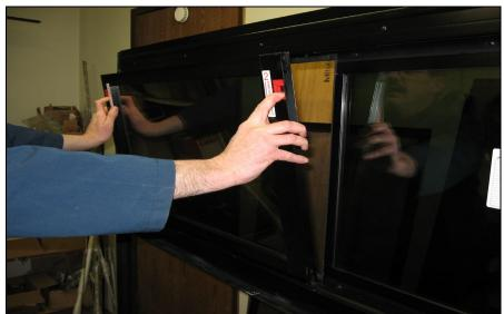
FIGURE 107: REMOVING THE SASH
