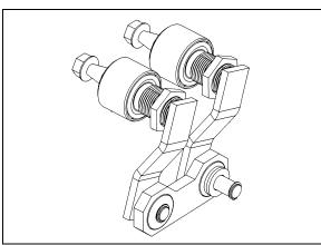
FIGURE 40: DRIVING MECHANISM (DRIVER SIDE) 23284
