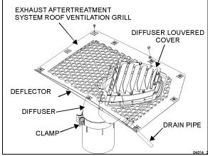
FIGURE 7: DIFFUSER ASSEMBLY
