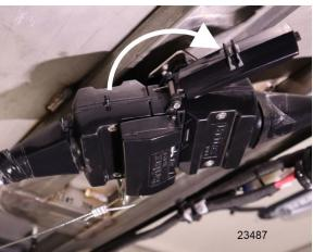
FIGURE 57: ELECTRICAL DISCONNECTION
