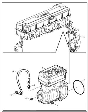
FIGURE 17: AIR COMPRESSOR LOCATION
