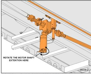
FIGURE 15: SLIDE-OUT MOTOR ROTATION
