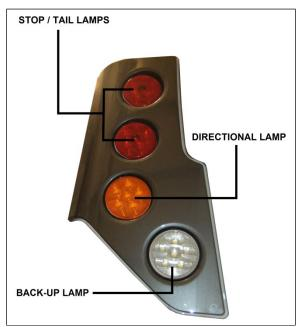
FIGURE 107: X3-SERIES REAR TAIL LAMPS, SOME VEHICLES MAY HAVE THE DIRECTIONAL LAMP MAY BE MOUNTED ON TOP POSITION
