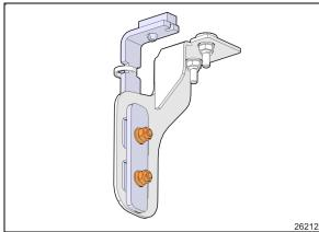
FIGURE 52: SENSOR BRACKET (FRONT)
