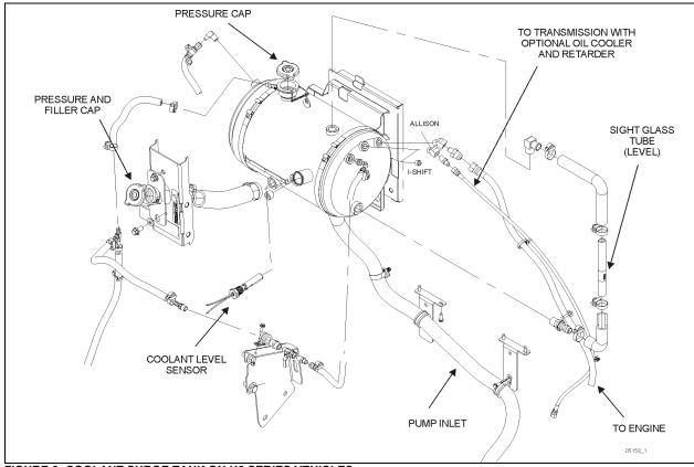
FIGURE 3: COOLANT SURGE TANK ON H3 SERIES VEHICLES
