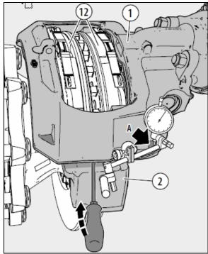
FIGURE 48: OBTAINING MAXIMUM VALUE OF BEARING CLEARANCE
