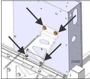
FIGURE 59: CONTROL BOX DISMOUNTING
