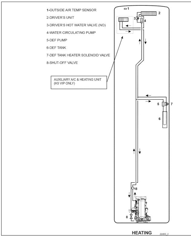
FIGURE 9: H3-45 VIP SMALL HVAC SYSTEM - HEATING
