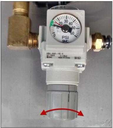
FIGURE 31: ADJUST TO 15 PSI ± 5 PSI
