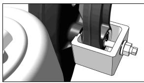
FIGURE 15: INSTALLING EXTRACTOR TOOL
