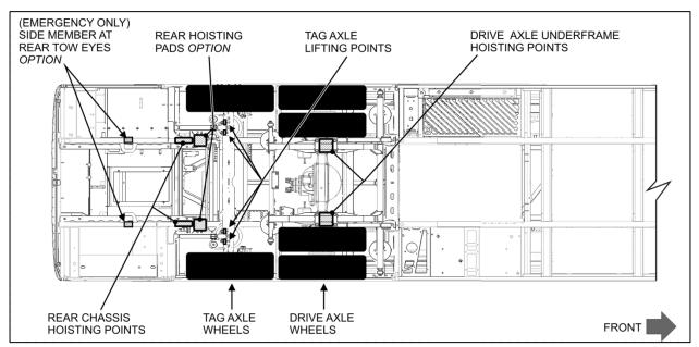
FIGURE 14 : X-SERIES OPTIONAL REAR CHASSIS HOISTING POINTS
