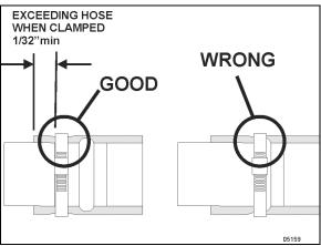
FIGURE 13: PROPER HOSE CLAMP INSTALLATION
