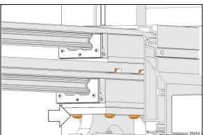
FIGURE 46: LOWER CARRIAGE MOUNTING SCREWS
