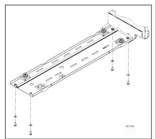
FIGURE 51: LOWER SUPPORT MOUNTING BOLTS
