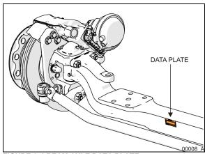
FIGURE 6: I-BEAM AXLE DATA PLATE
