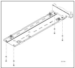
FIGURE 35: LOWER SUPPORT MOUNTING BOLTS
