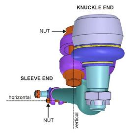
FIGURE 10: NOTE THE HORIZONTAL ORIENTATION OF THE CLAMP BOLT AT THE SLEEVE END AND ON WHICH SIDE THE NUT MUST BE POSITIONED
