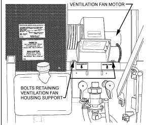
FIGURE 25: VENTILATION FAN INSTALLATION
