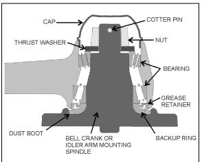
FIGURE 14: BELL CRANK OR IDLER ARM HUB
