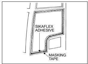
FIGURE 43: ADHESIVE-MOUNTED WINDOW
