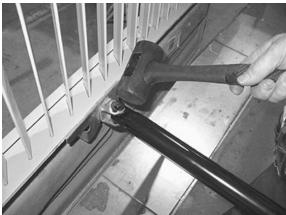
FIGURE 85: DOOR LATERAL ADJUSTMENT
