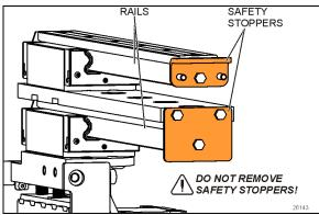
FIGURE 11: SAFETY STOPPERS ON RAILS
