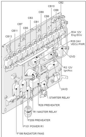
FIGURE 30: H3 SERIES MAIN POWER COMPARTMENT
