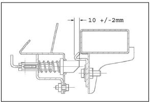
FIGURE 89: DOOR LATCHES ADJUSTMENT
