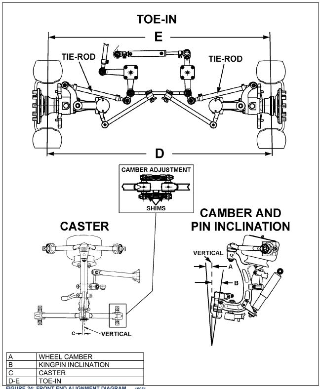
FIGURE 24: FRONT END ALIGNMENT DIAGRAM
