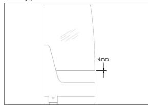
• Apply some masking tape **1mm** from window edge and body panel.
