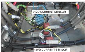
FIGURE 24: 12VD / 24VD CURRENT SENSORS IN MPC
