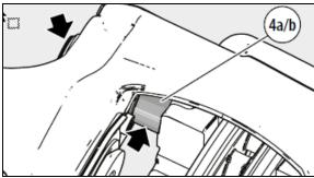
FIGURE 46: FREE GUIDE PIN OF DIRT
