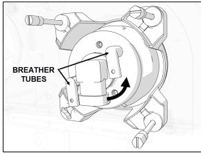
FIGURE 79: HALOGEN BULB REMOVAL
