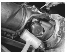
FIGURE 13: UNSEATING BEARING CUP ASSEMBLIES
