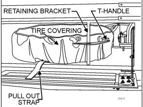
FIGURE 43: X3 SERIES SPARE WHEEL AND TIRE
