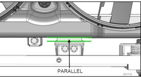
FIGURE 40: FAN SHROUD PARALLEL TO SUPPORT
