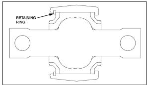
FIGURE 28: UPPER A-ARM BALL PIN BUSHING
