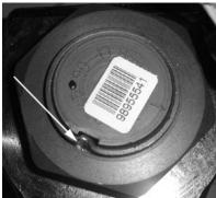
FIGURE 13: FIXING NUT PUNCH MARK
