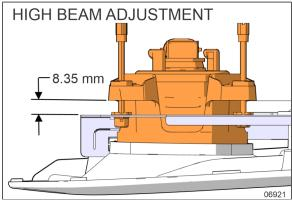
FIGURE 86: HIGH BEAM ADJUSTMENT
