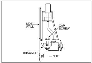
FIGURE 34: SIDE WALL MOUNTING
