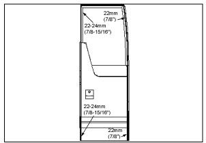
FIGURE 29: SEAL COMPRESSION ADJUSTMENT
