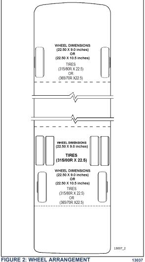
FIGURE 2: WHEEL ARRANGEMENT
