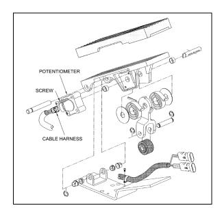
FIGURE 37: ELECTRONIC FOOT PEDAL ASSEMBLY 03035
