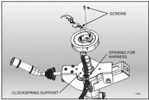
FIGURE 14: CLOCKSPRING INSTALLATION
