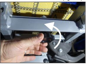
FIGURE 31: LOOSEN THE KNOB
