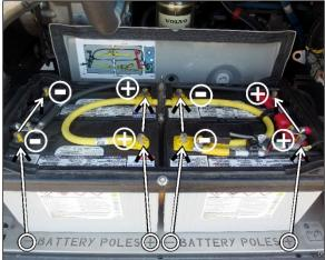
FIGURE 40: BATTERY INSTALLATION
