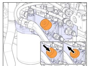
FIGURE 6: HAND PRIMING PUMP
