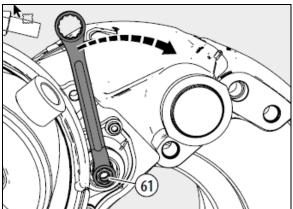
FIGURE 41: APPLY THE BRAKE 5-10 TIMES, SPANNER TURNS CLOCKWISE
