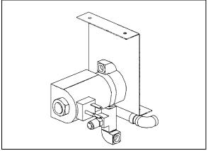
**FIGURE 31: AIR HORN VALVE**
