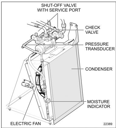
FIGURE 14: X3-45 VIP CONDENSER ARRANGEMENT
