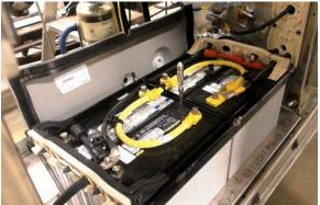
FIGURE 47: BATTERY BANK COVER REMOVED
