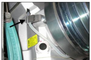
FIGURE 44: SHAFT SEAL OIL COLLECTING TUBE
