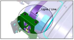
Before tightening the parts, make sure that the catalytic converter lower support is well centered with the exhaust inlet of the catalytic converter.
