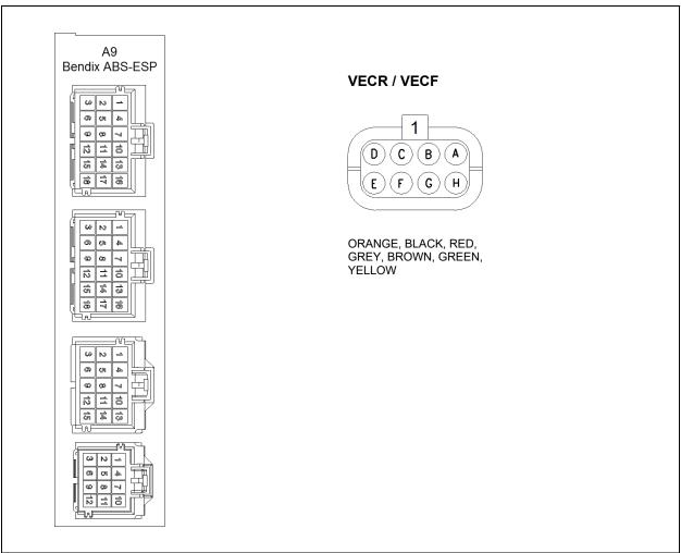
FIGURE 14: ELECTRONIC MODULES CONNECTORS PIN-OUT - BACK PROBING VIEW
