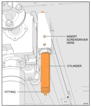
FIGURE 32: SECURITY PIN AIR CYLINDER REMOVAL
