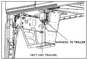
FIGURE 36: VECT (CURB SIDE) ON AIR FILTER BRACKET
