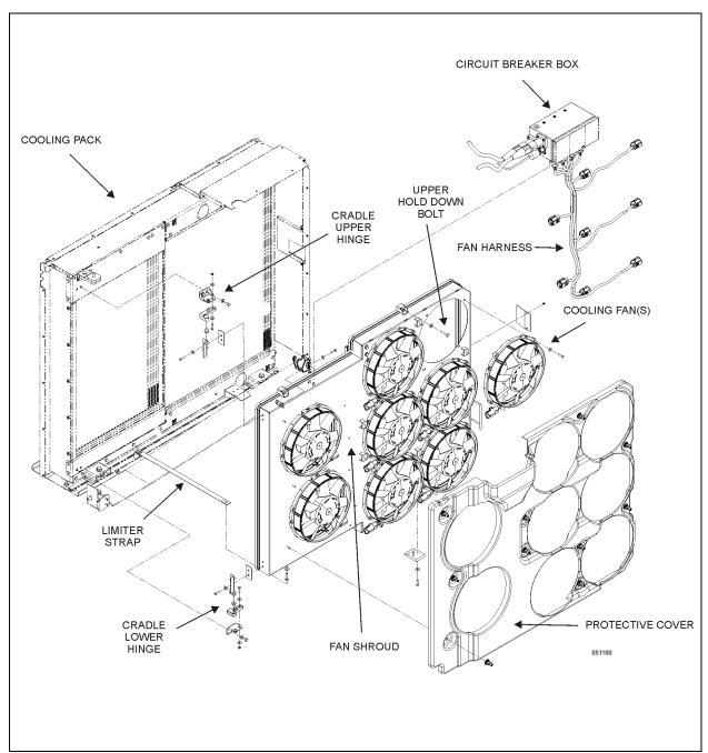
FIGURE 21: COOLING ASSEMBLY MAIN COMPONENTS
