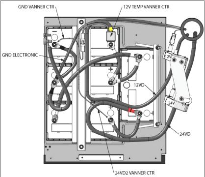
FIGURE 44: AGM BATTERY CONNECTIONS - H3 SERIES
