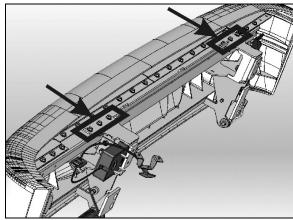
FIGURE 8: BUMPER ATTACHING BOLTS
