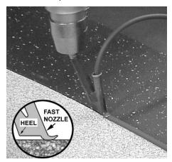
Allow cooling down of filler bead (about 5 minutes).
