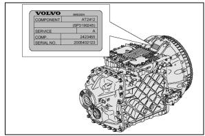
FIGURE 3: I-SHIFT TRANSMISSION
