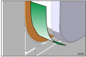
FIGURE 20: PLASTIC SHEET -WIPER SEAL PROTECTION
