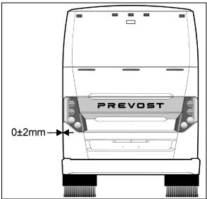
FIGURE 87: DOOR DEPTH ADJUSTMENT
