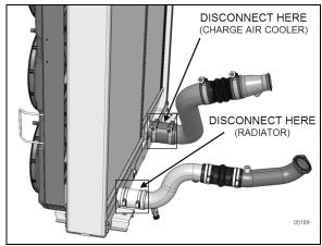
FIGURE 46: RADIATOR & CAC LOWER CONNECTION
