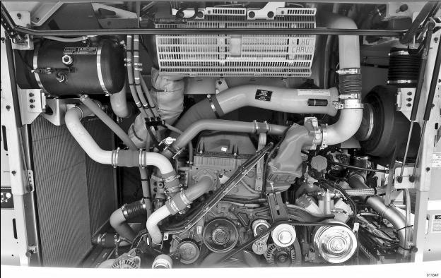
FIGURE 16: TYPICAL X SERIES ENGINE COMPARTMENT
