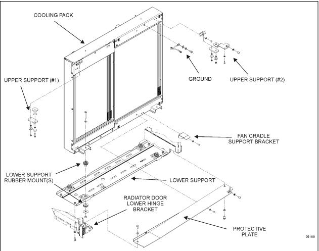
FIGURE 33: COOLING PACK SUPPORTS AND COMPONENTS
