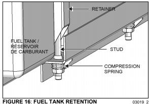
FIGURE 16: FUEL TANK RETENTION
