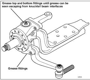
FIGURE 2: FRONT AXLE GREASING POINTS
