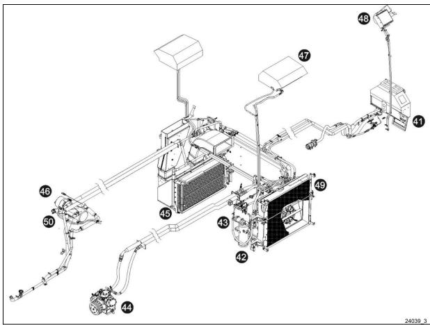
FIGURE 3: LUBRICATION AND SERVICING POINTS - HVAC UNIT
