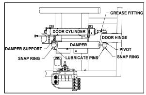
FIGURE 15: DOOR CYLINDER AND DAMPER
