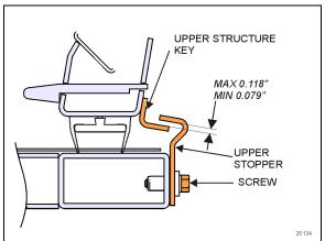
FIGURE 27: UPPER INNER STOPPERS ADJUSTMENT
