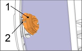
FIGURE 103: (1) LOCK RING; (2) TAB
