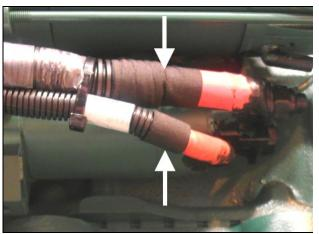
Stud terminal nuts properly tightened. Use a nut with nylon insert to replace a similar nut where applicable. Protect ring cable lugs against tightening force by placing a flat washer between nut and ring cable lug.
