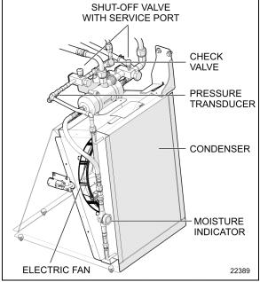
FIGURE 61 X3 SERIES SMALL A/C CONDENSER ASSEMBLY.
