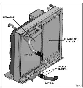
FIGURE 11: COOLANT FLOW (X3 SERIES SHOWN)
