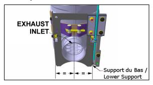
While tightening the bolts, keep in mind to respect the alignment of the parts and keep the lower support as centered as possible with the catalytic converter exhaust inlet.
