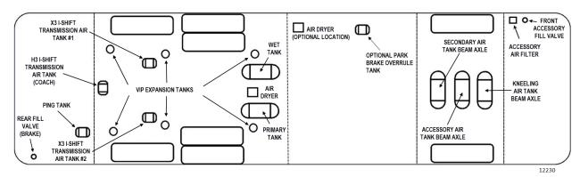
FIGURE 3: I-BEAM AXLE SUSPENSION AIR TANKS LOCATIONS (TYPICAL WITH VIP EXPANSION TANKS)
