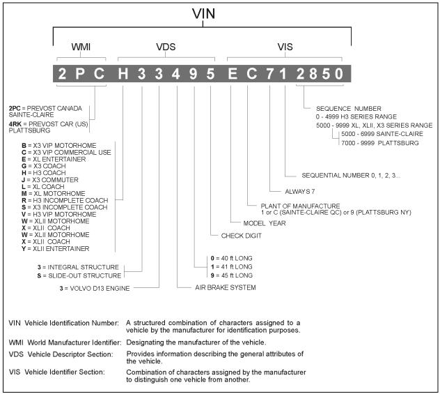
FIGURE 10: VEHICLE IDENTIFICATION NUMBER
