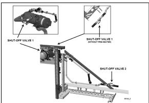
FIGURE 93: H3 SERIES HEATER LINE SHUTOFF VALVES 05144
