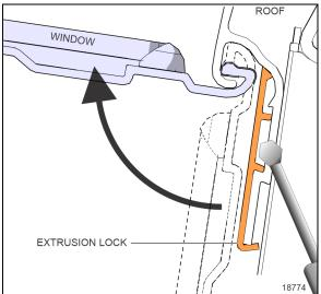
FIGURE 41: EMERGENCY EXIT WINDOW REMOVAL
