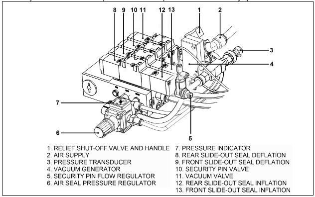
FIGURE 48: PNEUMATIC COMPONENT PANEL
