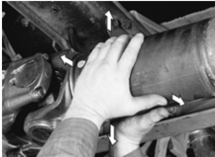
FIGURE 6: CHECK FOR LOOSENESS
