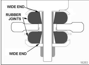
FIGURE 40: LOWER SHOCK MOUNTING BUSHINGS
