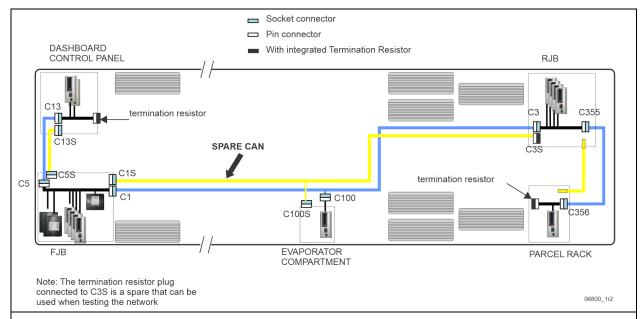
If all modules (AE41 to AE58) are showed as Not Responding and Active Fault, the problem could be:
