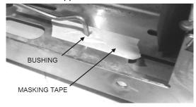
Install CAC on the vehicle and secure to the lower support using both lower hex bolts, washers and remaining plastic insulating bushings.
