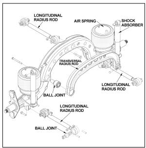
FIGURE 36: TAG AXLE SUSPENSION
