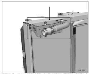
FIGURE 41: INSTALLED RADIATOR UPPER PIPE & BRACKET
