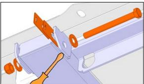
FIGURE 29: SHIM INSTALLATION, TRANSVERSE SCREW, ARRANGEMENT MAY VARY
