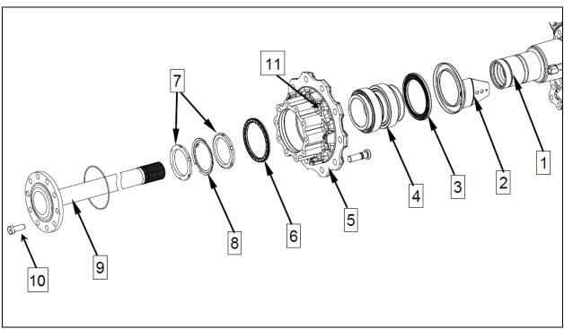
FIGURE 12: ZF A-132 DRIVE AXLE HUB ASSEMBLY
