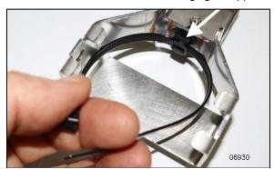
FIGURE 115: CABLE TIE INSTALLATION
