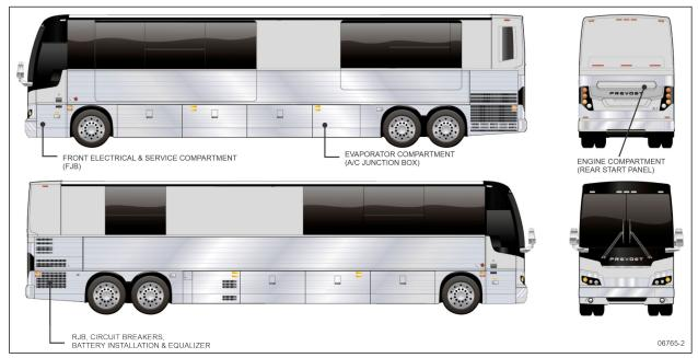
FIGURE 19: ELECTRICAL COMPARTMENTS (X3-45 VIP)
