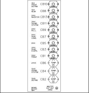
FIGURE 81: H3 SERIES MAIN CIRCUIT BREAKERS
