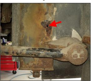
FIGURE 7: HOLE DRILLED IN STRUCTURAL MEMBER
