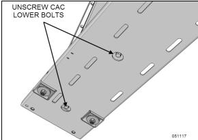
FIGURE 64: LOWER CAC INSULATED BOLTS
