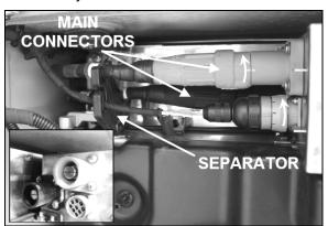
FIGURE 24: CIRCUIT BREAKER BOX CONNECTIONS
