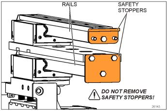
FIGURE 6: SAFETY STOPPERS ON RAILS
