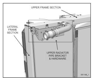
FIGURE 37: COOLING PACK PARTS TO BE REMOVED FOR RADIATOR REPLACEMENT
