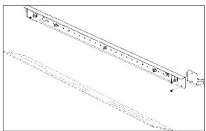
FIGURE 129: LED DIRECT LIGHTING AND LENS
