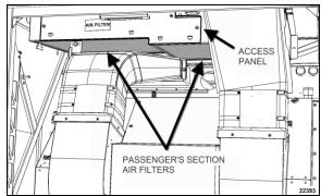
FIGURE 33: PASSENGERS' SECTION AIR FILTER
