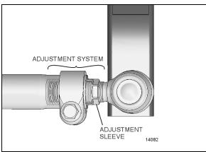
FIGURE 23: DRAG LINK ADJUSTMENT SYSTEM
