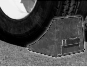
FIGURE 21 CHOCK THE FRONT AND REAR WHEELS
