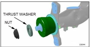
FIGURE 21: INSTALL THRUST WASHER AND HUB NUT
