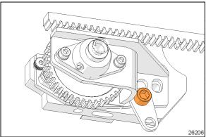
FIGURE 36: LOWER SCREW, TENSION RELIEVED
