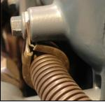
Figure 22: P-clamp with appropriate diameter prevents the power cable or corrugated protective sheath from moving and rubbing inside the clamp.
