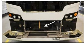
FIGURE 13: FRONT BUMPER AND SPARE TIRE
