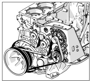
FIGURE 100 X3 SERIES SMALL A/C COMPRESSOR
