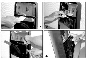
FIGURE 17: REAR VIEW MIRROR GLASS REMOVAL
