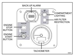
FIGURE 37: REAR START PANEL WITH TACHOMETER
