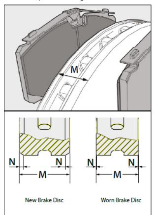
FIGURE 31: BRAKE DISC THICKNESSES AND OPTICAL WEAR INDICATOR
