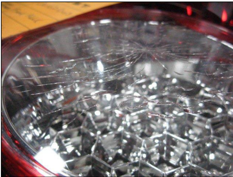
FIGURE 3: Cracking of the outer surface of the taillight due to the use of engine degreaser
