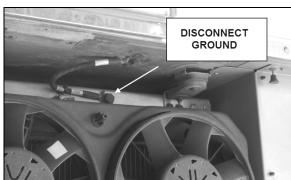
FIGURE 32: COOLING ASSEMBLY GROUND
