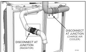
FIGURE 45: RADIATOR & CAC UPPER CONNECTION
