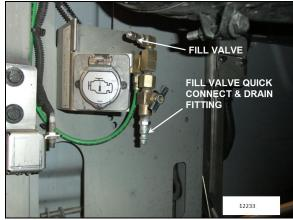
FIGURE 12: REAR VALVE LOCATION (TYPICAL)
