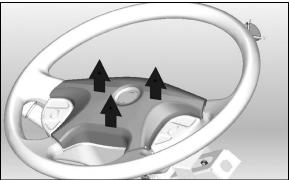
FIGURE 11: REMOVING THE HORN PAD
