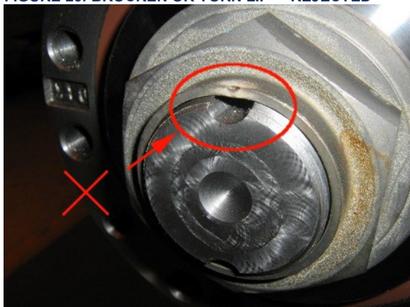
FIGURE 27: LIP INADEQUATELY PRESSED IN – REJECTED
