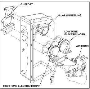
FIGURE 31: ELECTRIC & AIR HORN INSTALLATION 23420
