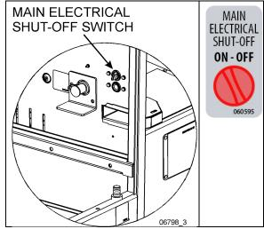
FIGURE 46: H3 SERIES MAIN ELECTRICAL SHUT-OFF SWITCH
