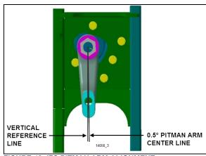
FIGURE 42: IFS PITMAN ARM ALIGNMENT
