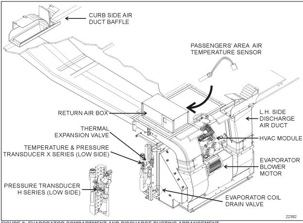
FIGURE 8: EVAPORATOR COMPARTMENT AND DISCHARGE DUCTING ARRANGEMENT
