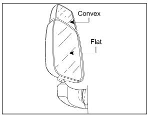
FIGURE 15: REAR VIEW MIRROR (RAMCO)
