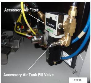
FIGURE 4: FRONT SERVICE COMPARTMENT
