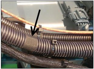
Figure 14: Two layers of fabric tape applied every 3 Figure 15: The ends of the corrugated protective to 6 inches to prevent the cable from coming out of sheath should be covered with fabric tape. the corrugated protective sheath.
