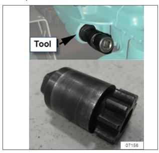
FIGURE 10: VOLVO ENGINE TURNING TOOL #88800014
