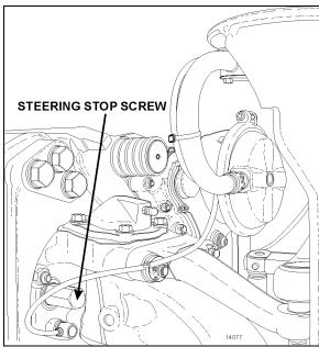
FIGURE 17: STEERING STOP SCREW ON I-BEAM AXLE
