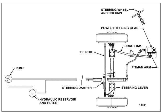
FIGURE 1: I-BEAM AXLE STEERING SYSTEM SETUP
