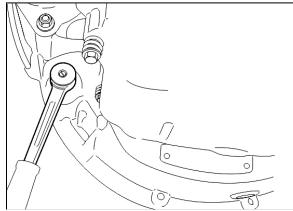
FIGURE 16: VOLVO ENGINE CRANKING POSITION
