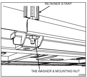
FIGURE 23: FUEL TANK STRAP MOUNTING
