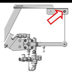
5. Loosen the lower mounting bolt shown.
