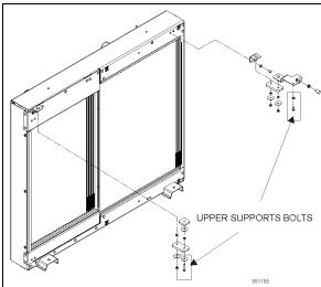
FIGURE 36: UPPER SUPPORTS MOUNTING BOLTS
