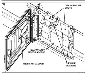
FIGURE 83: X3 SERIES PASSENGERS' AREA FRESH AIR DAMPER
