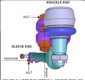
FIGURE 5: NOTE THE VERTICAL ORIENTATION OF THE CLAMP BOLT AT THE KNUCKLE END AND ON WHICH SIDE THE NUT MUST BE POSITIONED
