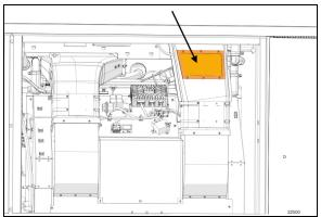
FIGURE 106:MODULES ACCESS COVER IN THE EVAPORATOR COMPARTMENT
