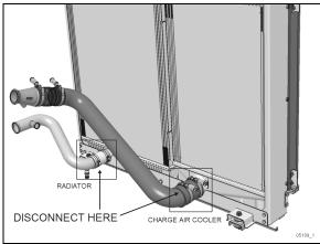
FIGURE 31: RADIATOR & CAC LOWER CONNECTION
