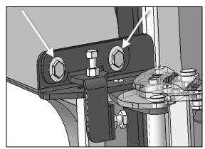
3. Using the top adjusting screws, adjust door to get a 6mm gap at the top.
