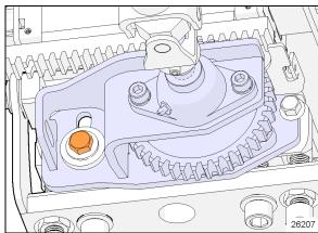
FIGURE 35: REMOVE TENSION. SLIGHTLY UNSCREW.
