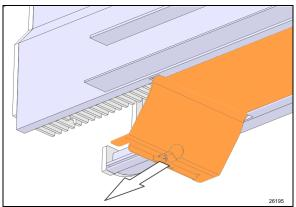
FIGURE 24: PULLING THE FLEXIBLE COVER OUT.
