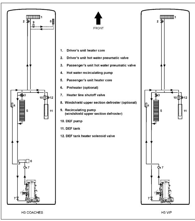
FIGURE 2: H3 SERIES BIG HVAC SYSTEM - HEATING CIRCUIT
