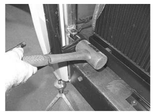
FIGURE 84: PANTOGRAPH ARM ADJUSTMENT
