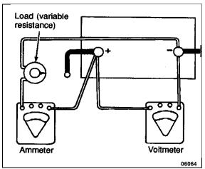
FIGURE 60: LOAD TEST
