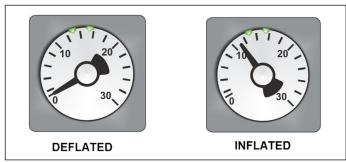
FIGURE 7: INFLATABLE SEAL PRESSURE GAGE
