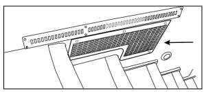
FIGURE 25: R.H CONSOLE AIR FILTER ACCESS GRILL (COACHES) 18505
