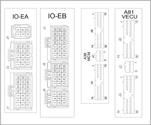
FIGURE 13: ELECTRONIC MODULES CONNECTOR PIN-OUT - BACK PROBING VIEW
