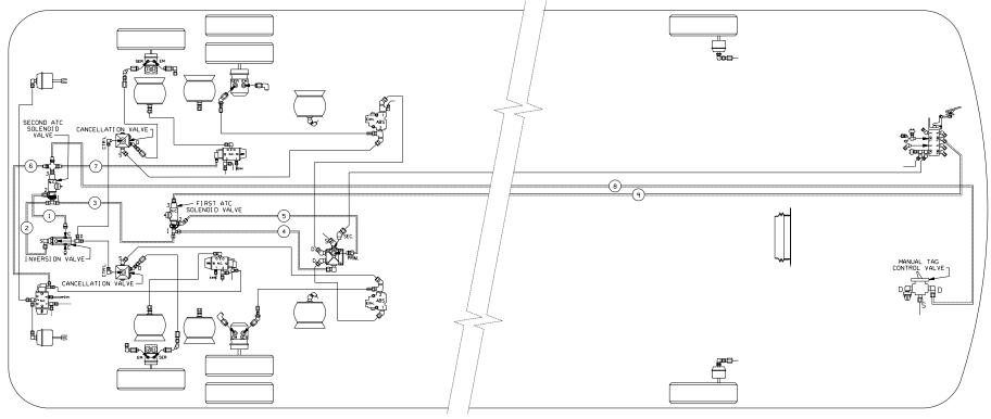
Traction Control(ATC) with ABS
