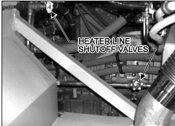
FIGURE 7: HEATER LINE SHUTOFF VALVES 05041
