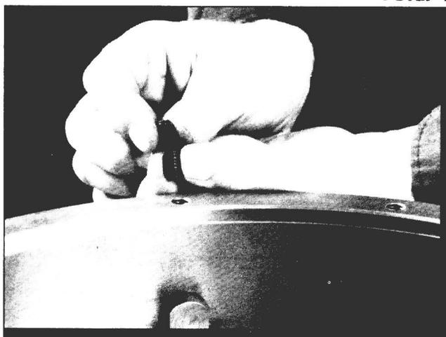
Mark the flywheel to crankshaft position with a piece of soapstone or chalk and remove the crankshaft bolts. Remove the flywheel and set it on a flat work surface.
