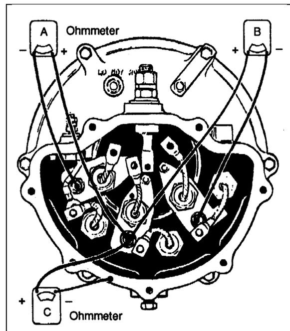
FIGURE 26: CHECKING STATOR WINDING FOR "OPEN" AND GROUND
