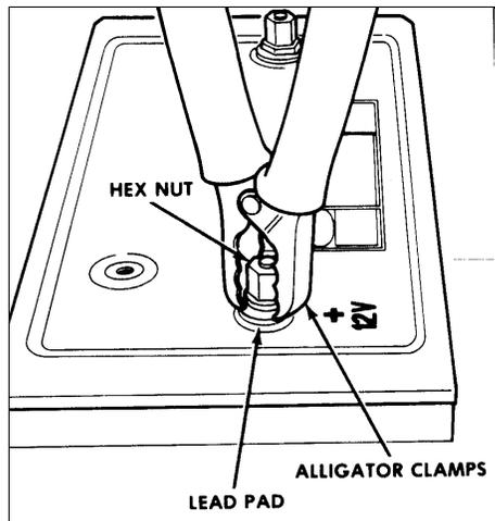
FIGURE 19: ALLIGATOR CLAMPS AND BATTERY
