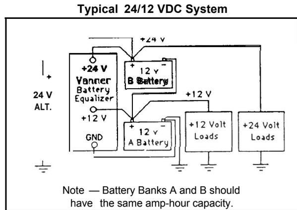
A key advantage of the *VoltMaster* Battery Equalizer, when compared to DC converters, is that *voltMaster*'s unique system design enables it to sustain momentary current surges in excess of its rated capacity. If the 12 volt load requires a momentary surge in current, the *VoltMaster* will permit that extra current to be drawn from Battery A. The Battery Equalizer will then replenish the energy to Battery A after the surge has passed.
