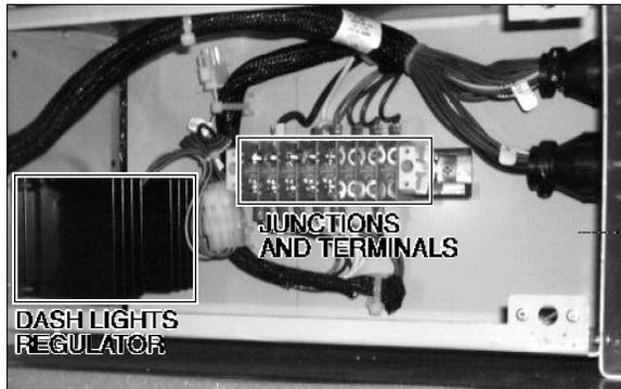
FIGURE 13: IN ALARM JUNCTION BOX 06060
