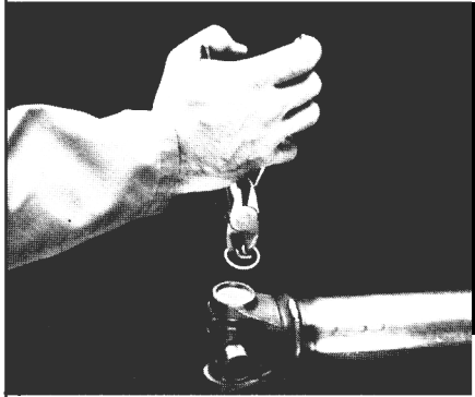
4. Install a snap ring.
