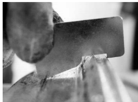
Photo 1. Acceptable Rim Flange Wear Condition
