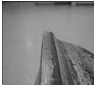
Photo 8. Severe rim flange wear.
