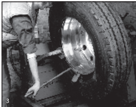
3 Lubricate the second tire bead. Start second bead into the well, holding it in position with the clamp to the rim flange. Lubricate bead half way around. With curved end of tool between tire bead and flange, and the stop towards the wheel, push tool outward to work tire over flange. Continue to pry bead over flange using the tool until remaining bead is over flange. Seat the tire bead using an air ring or other mechanical bead seating aid.
