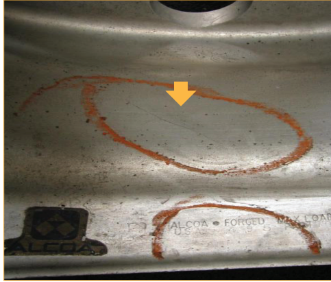
Drop center crack
