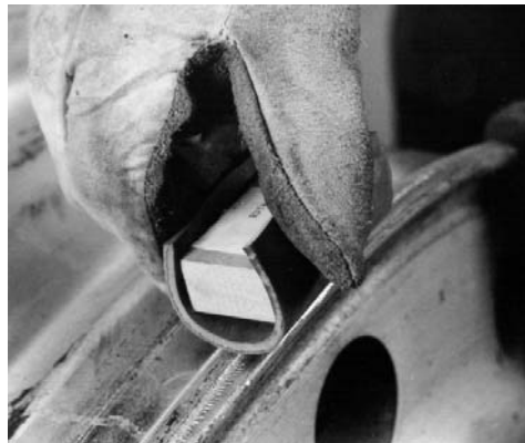
Photo 2. A rubber sharpness gauge constructed from a section of tire side wall or a suitable piece of rubber attached to a block of wood.
