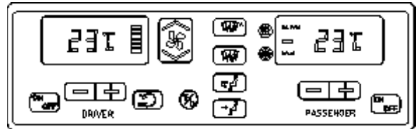
FIGURE 5: CENTRAL HVAC SYSTEM CONTROL UNIT 22296
