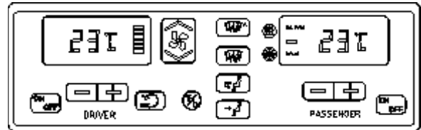
FIGURE 5: CENTRAL HVAC SYSTEM CONTROL UNIT 22296
