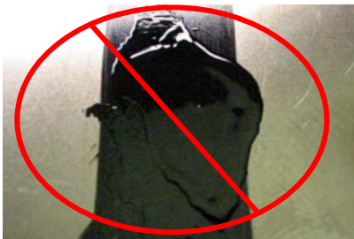
Dripping, avoid excessive accumulation
