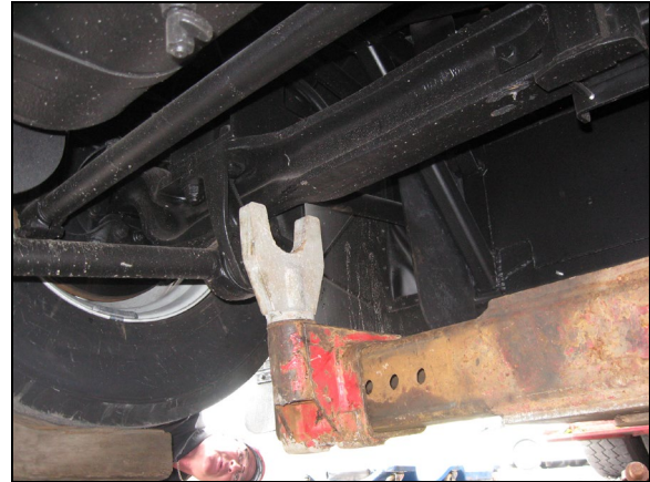
LIFTING FROM UNDER THE FRONT AXLE
