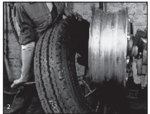
2 Insert curved end of tool between bead and wheel flange with tool stop against flange. In circular motion, use short successive bites to work the bead over the flange. Push down on tool as bead is worked over flange.
