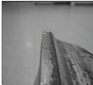
Photo 8. Severe rim flange wear.
