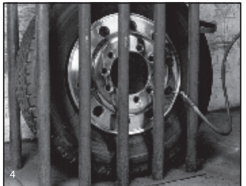
4 Place tire/wheel assembly inside safety cage or other suitable restraint (refer to OSHA rule 1910.177, paragraph b, see Section 7). Refer to tire manufacturer's recommendation for proper tire pressure. Using a clip-on air chuck or a self-locking straight chuck with remote valve and pressure gauge, inflate the tire/wheel assembly to proper pressure. If air escapes, roll tire or use bead expander to force tire beads against rim. Be sure to stay out of the path of potential exploding parts or air blasts.
