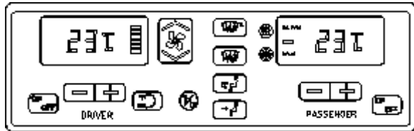
FIGURE 6: CENTRAL HVAC SYSTEM CONTROL UNIT
