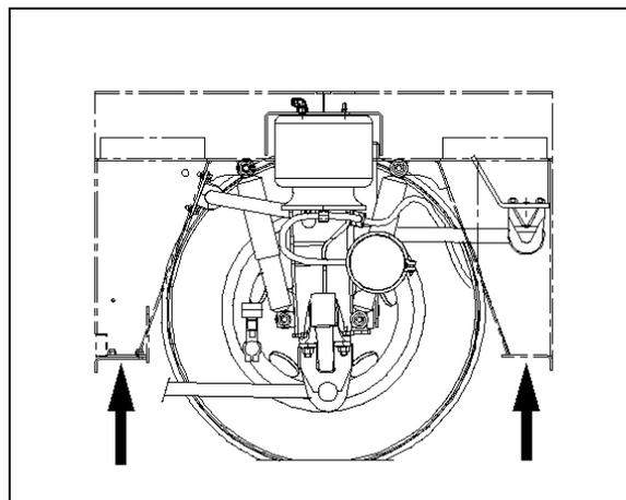
POINTS DE LEVAGE SOUS LE CHÂSSIS AVANT –
