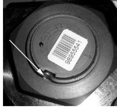
FIGURE 17: FIXING NUT PUNCH MARK
