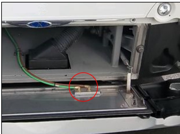
FIGURE 10: FRONT BUMPER AIR LINES 18701
