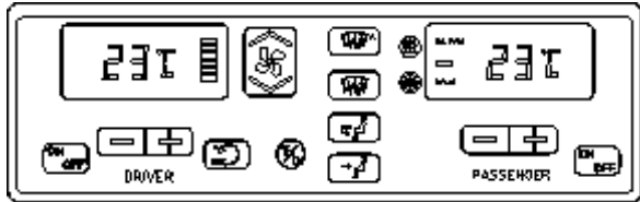
FIGURE 6: CENTRAL HVAC SYSTEM CONTROL UNIT
