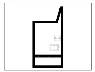
Apply 1/8 x1/4 double face self-adhesive tape onto door frame.
