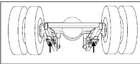
FIGURE 93: JACKING POINTS ON DRIVE AXLE OEH3B762
