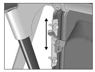
9. Make sure that skid bar only touches slightly bus structure at bottom. The door should not move up when closing.
