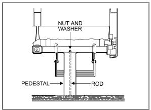
FIGURE 48: SEAT PEDESTAL ASSEMBLY
