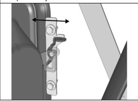
5. Check handle adjustment. Handle must remain tight against its plastic housing.
