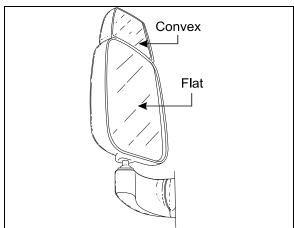
FIGURE 56: REAR VIEW MIRROR (RAMCO)
