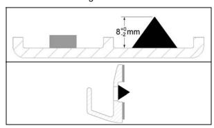
Position and fix vertical molding. Lean vertical molding against lateral molding. Make sure vertical molding lines up with structural tubing.
