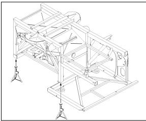
FIGURE 89: FRONT END JACKING POINTS
