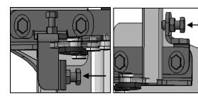
5. To adjust door depth, loosen the screws fixing the hinge to frame assembly and slide the hinge horizontally to move the door in or out. Depth should be calculated at 29mm +/2mm measured from bus frame out or 5mm +1mm if measurement is taken from small square tube on frame.
