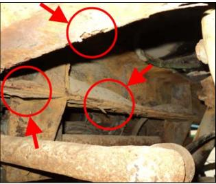
FIGURE 3: METAL FLAKING AND ACCUMULATED SAND
