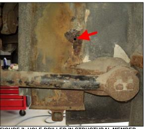
FIGURE 7: HOLE DRILLED IN STRUCTURAL MEMBER
