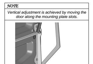
3. Center door in the opening using the retaining rings.
