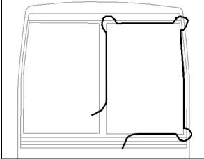
FIGURE 15: WINDSHIELD INSTALLATION USING ROPE
