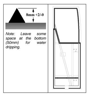
Install and center fiber glass body panel onto door frame leaving an excess of 3mm all around the frame.
