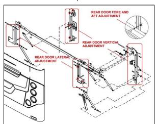
FIGURE 70: ENGINE COMPARTMENT DOOR
