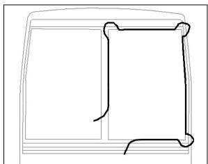
FIGURE 57: WINDSHIELD INSTALLATION USING ROPE
