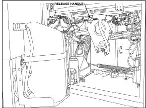
FIGURE 11: FRONT BUMPER RELEASE HANDLE
