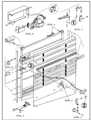
FIGURE 35: ENGINE COMPARTMENT R.H. SIDE DOOR 18635
