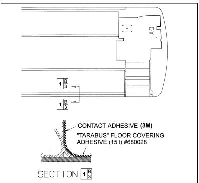
FIGURE 49: TARABUS FLOOR COVERING ADHESIVE APPLICATION
