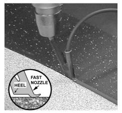
9. Allow cooling down of filler bead (about 5 minutes).
