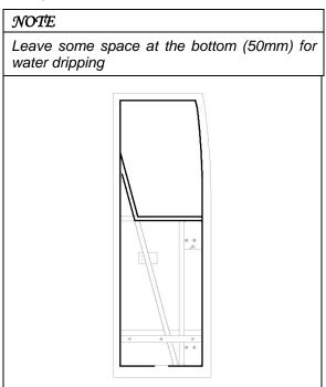
• Apply Sika 255 onto door frame structure.
