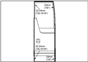
FIGURE 25: SEAL COMPRESSION ADJUSTMENT
