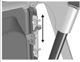
16. Open baggage compartment door and adjust using the cylinder mounting block.
