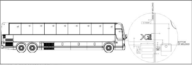
FIGURE 45: SIDE CREST POSITIONING
