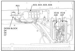
FIGURE 17: ENTRANCE DOOR & WIPER CONTROL PANEL 06619
