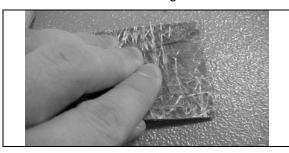
Allow drying for at least **2 hours** then repaint as per paragraph: Minor Repair.
