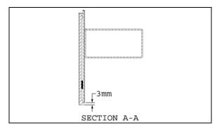
Line-up body panel with window. There must be a gap of 4±2mm between window and body panel.
