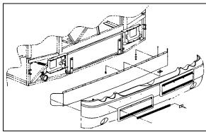
FIGURE 13: FRONT BUMPER REMOVAL
