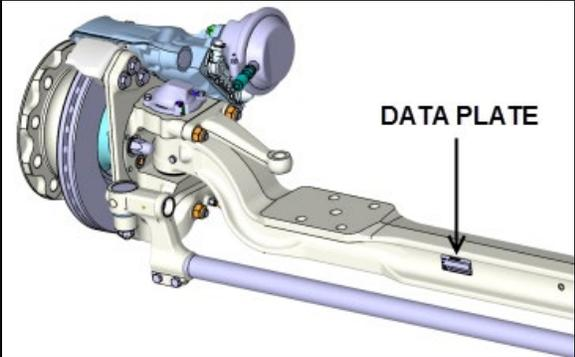
**FIGURE 6: I-BEAM AXLE TYPICAL SERIAL & MODEL NUMBERS** 00008
