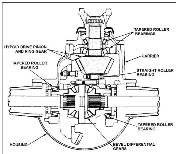
FIGURE 2: DIFFERENTIAL ASSEMBLY
