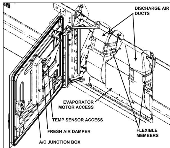
**FIGURE 35: X3 SERIES EVAPORATOR COMPARTMENT**<sup>T22301\_B</sup>
