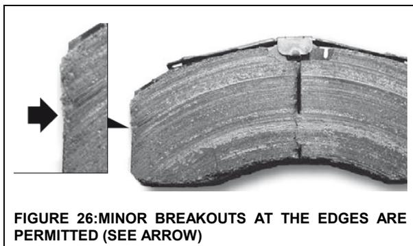
FIGURE 26: MINOR BREAKOUTS AT THE EDGES ARE PERMITTED (SEE ARROW)
