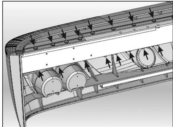
**FIGURE 9: ALUMINUM EXTRUSIONS - BUMPER SKIN REMOVAL**
