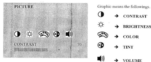
Select the function (e.g. contrast) by pressing the key **SELECT** repeatedly. The setting within the function can be modified with the keys **UP** and **DOWN**.
