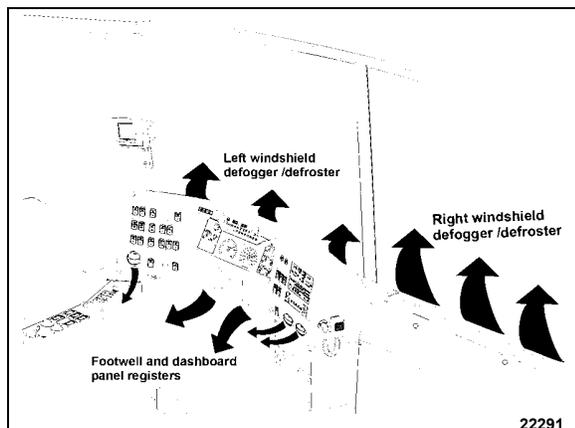
**FIGURE 61: DRIVER'S UNIT AIR CIRCULATION**
