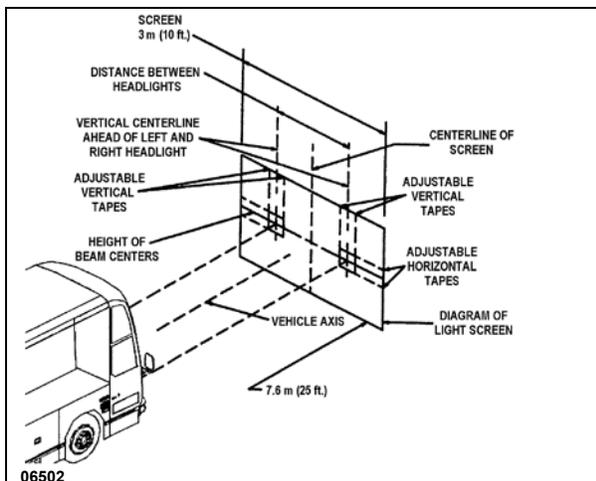
FIGURE 47: HEADLIGHT AIMING SCREEN ALIGNMENT 06502
