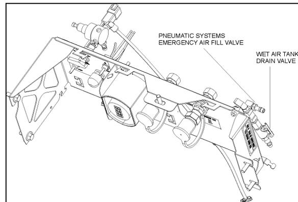
FIGURE 46: REAR VALVE LOCATION ON H3 SERIES<sup>12162</sup>
