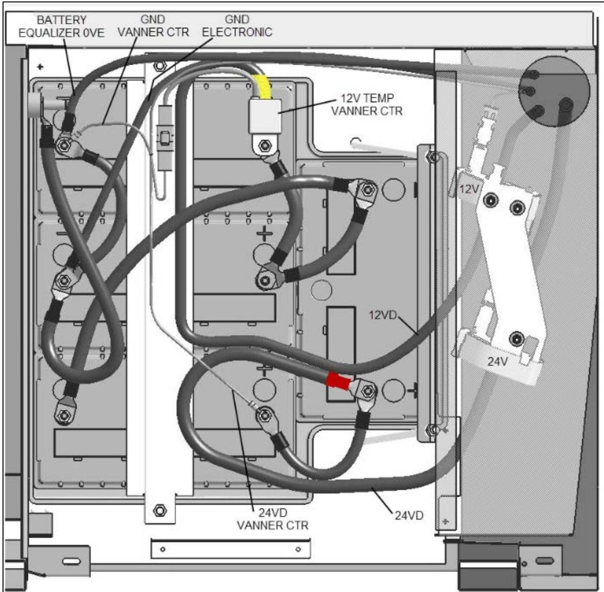
FIGURE 26: H3 SERIES AGM BATTERY CONNECTIONS (PRIME SYSTEM)
