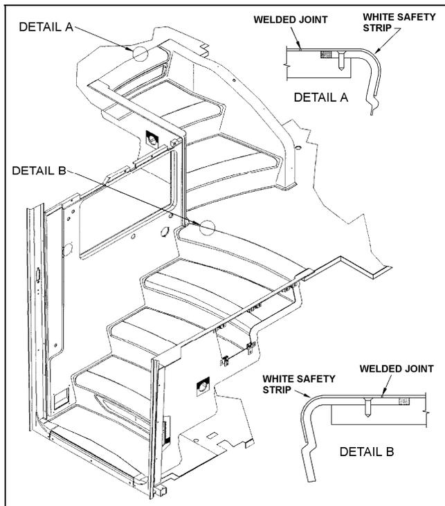
5. Apply contact adhesive (3M) (684655 or 684654) onto both surfaces to glue (fiberglass and back of white safety strip). Drying time: 4 to 5 minutes.
