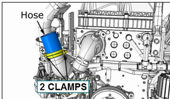
FIGURE 10: COOLANT LINE AT PUMP INLET
