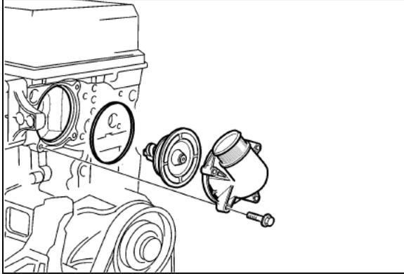
FIGURE 5: VOLVO D13 THERMOSTAT HOUSING
