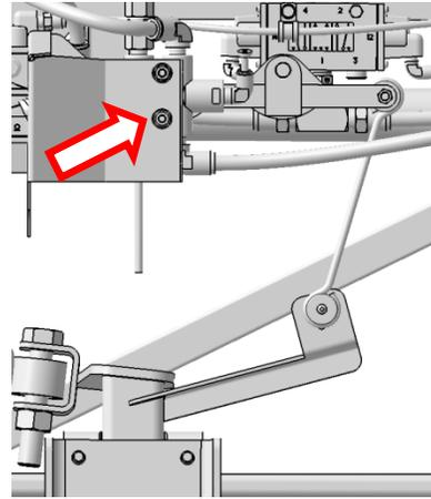
6. Rotate the valve body to increase or decrease the clearance as shown (the mounting bracket has a slotted hole).
