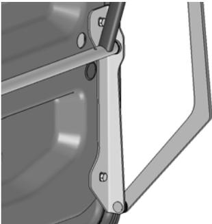
3. Center door in the opening using the retaining rings.
