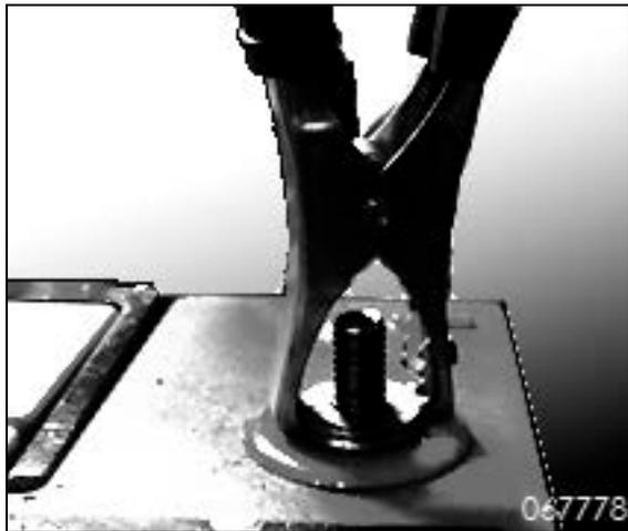
FIGURE 29 ALLIGATOR CLAMP POSITION- TYPICAL AGM BATTERY
