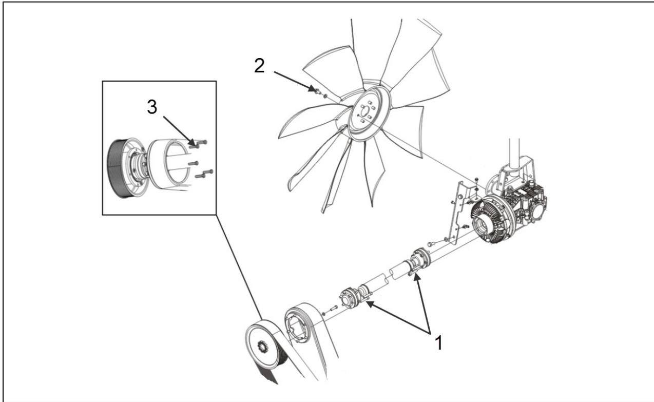
**COOLING FAN DRIVE MECHANISM**
