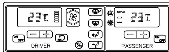
FIGURE 64: CONTROL UNIT - CENTRAL HVAC SYST 22276
