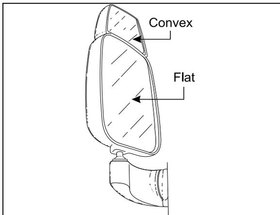
FIGURE 56: REAR VIEW MIRROR (RAMCO)
