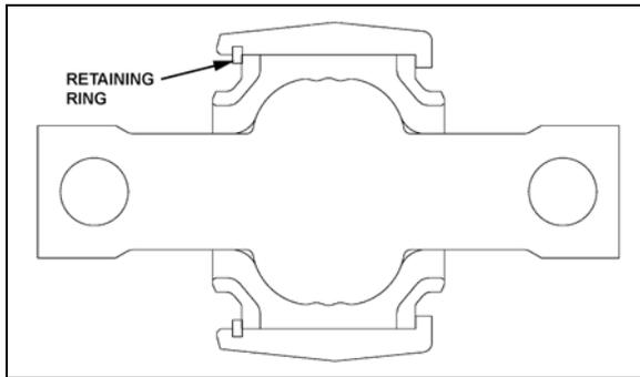
FIGURE 30: UPPER A-ARM BALL PIN BUSHING
