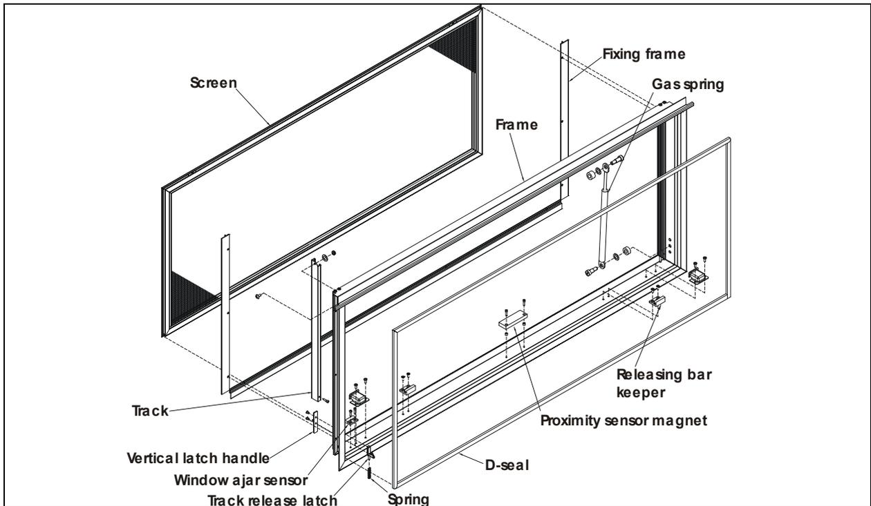
FIGURE 61: ELECTRIC AWNING WINDOW EXPLODED VIEW (FRAME) 18586
