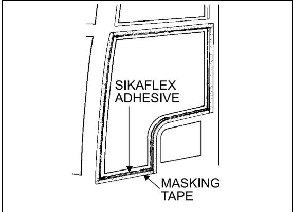
FIGURE 37: ADHESIVE-MOUNTED WINDOW 18081
