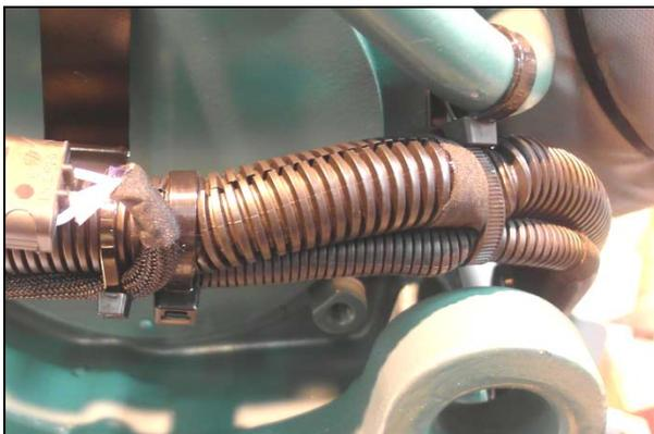
Figure 10: starter cables in a corrugated protective sheath.
