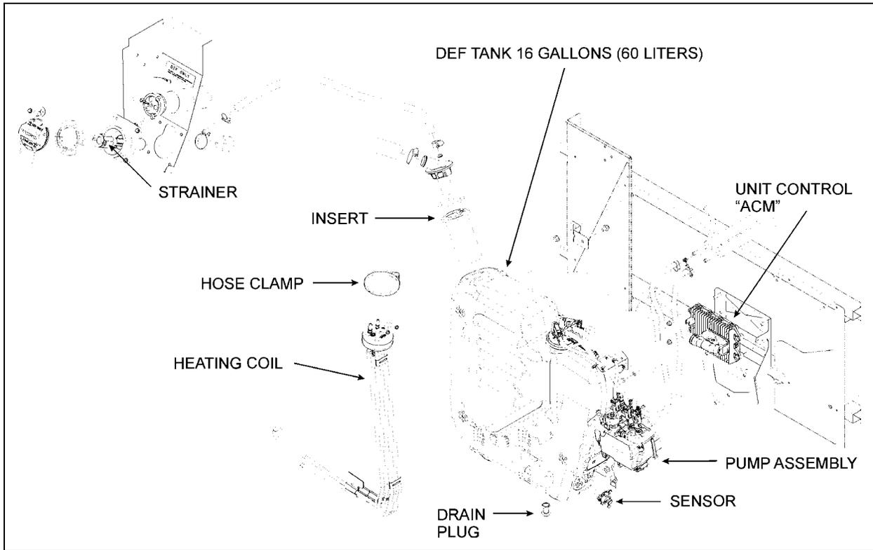
FIGURE 10: H SERIES DEF TANK AND PUMP
