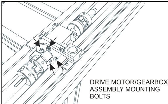
FIGURE 20: DRIVE MOTOR/GEARBOX ASSEMBLY MOUNTING BOLTS
