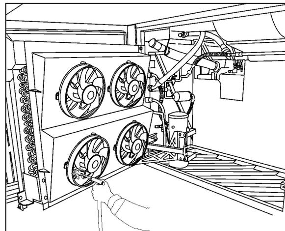
**FIGURE 15: CLEANING PASSENGER'S UNIT CONDENSER COIL WITH LOW-PRESSURE AIR JET** 22362
