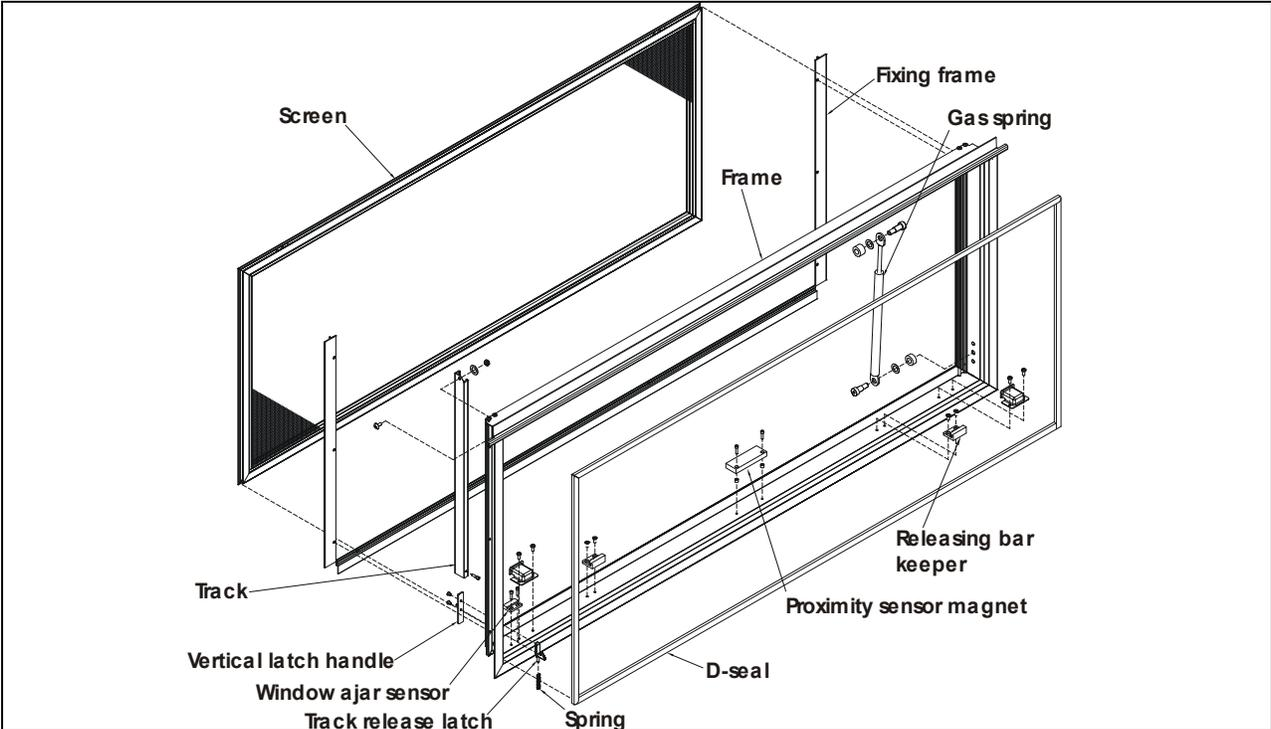
FIGURE 38: ELECTRIC AWNING WINDOW EXPLODED VIEW (FRAME)
