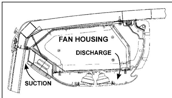
FIGURE 63: OVERHEAD COMPARTMENT VENTILATION SYSTEM 22211
