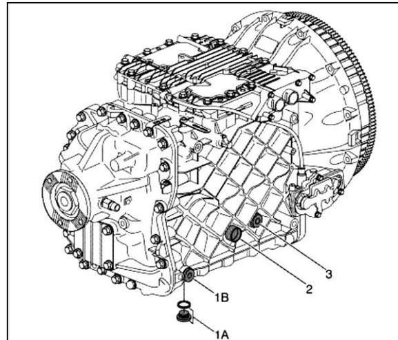
FIGURE 17: I-SHIFT TRANSMISSION OIL CHANGE
