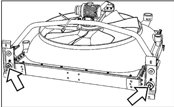
FIGURE 33: REMOVING FASTENERS
