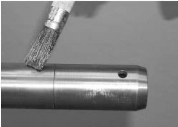
FIGURE 10: APPLY GLEITMO 805 GREASE
