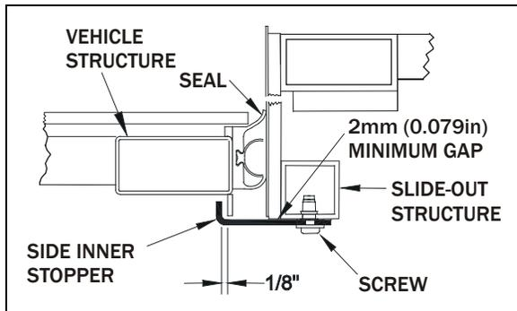
FIGURE 5: SIDE INNER STOPPER ADJUSTMENT
