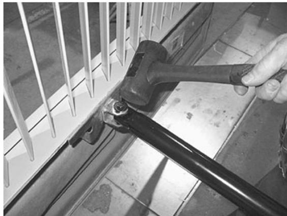
FIGURE 64: DOOR LATERAL ADJUSTMENT
