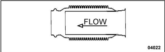
FIGURE 2: FLEXIBLE COUPLING
