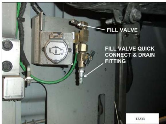
FIGURE 6: REAR VALVE LOCATION (typical)
