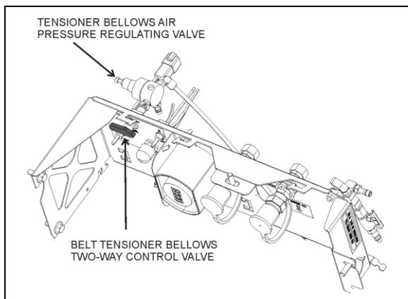
FIGURE 26: BELT TENSIONER CONTROL VALVE - H3 SERIES
