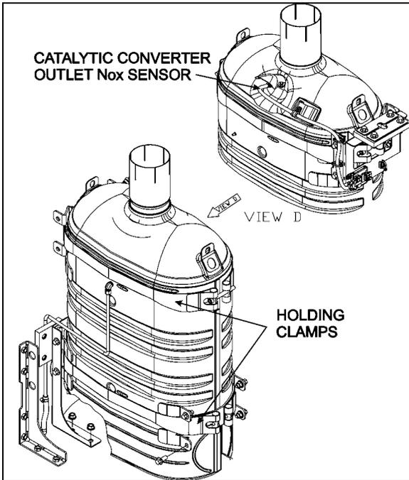
FIGURE 5: CATALYTIC CONVERTER
