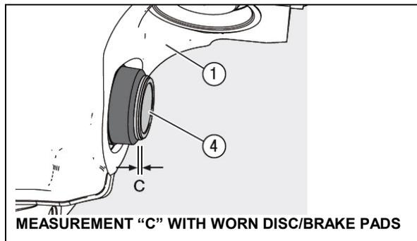
FIGURE 23: BRAKE PAD WEAR CHECK ON DRIVE AXLE
