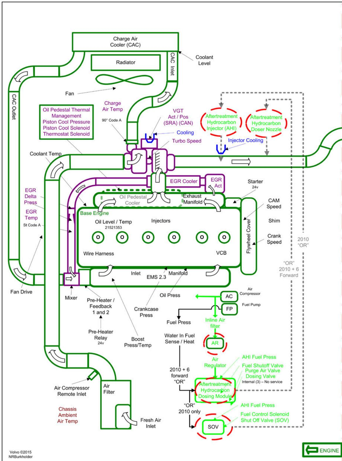
FIGURE 4: 2010-2015 ENGINE & EXHAUST AFTERTREATMENT SYSTEM DIAGRAM (1 OF 2)
