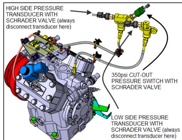
FIGURE 30: PRESSURE TRANSDUCERS
