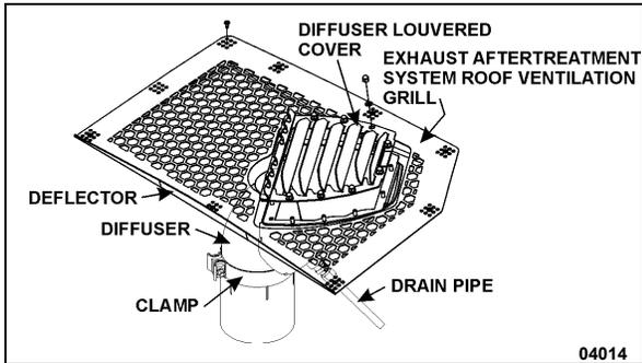
**FIGURE 6: DIFFUSER ASSEMBLY**
