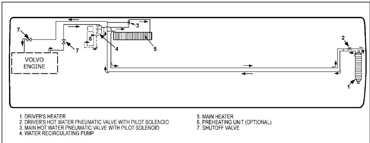
FIGURE 5: X3 SERIES CENTRAL HVAC SYSTEM – HEATING CIRCUIT
