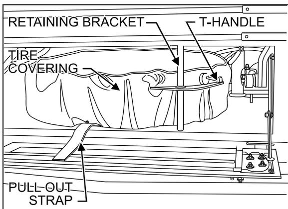
**FIGURE 29: X3 SERIES SPARE WHEEL AND TIRE**
