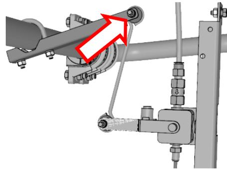
6. Using a hammer, tap gently on the arm secured to the sway bar. Even if the fasteners are properly tightened, it will rotate around the sway bar. Rotate the arm secured to the sway bar to increase or decrease the clearance as shown.
