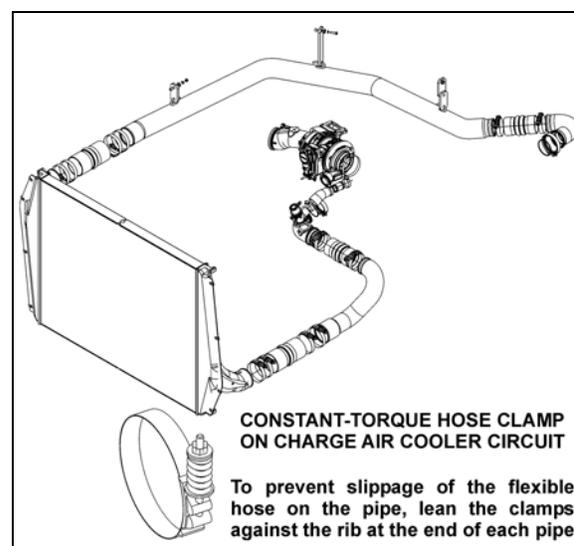
FIGURE 12: CHARGE AIR COOLER HOSE CLAMPS
