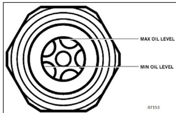
FIGURE 18: SIGHT GLASS FOR CHECKING OIL LEVEL
