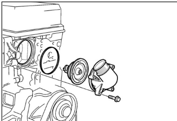
**FIGURE 13: VOLVO D13 THERMOSTAT HOUSING**
