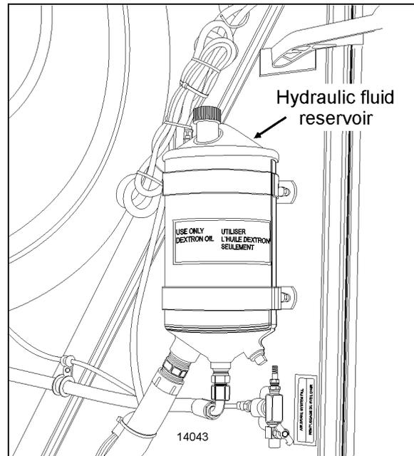
**FIGURE 25: HYDRAULIC FLUID RESERVOIR LOCATION****13.2.1 Oil Level Check Procedure**
