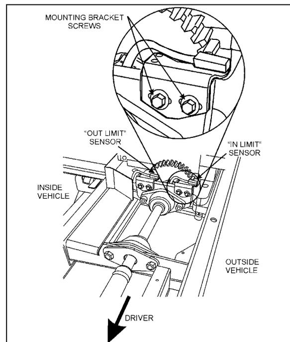
FIGURE 39: SLIDE-OUT SENSORS
