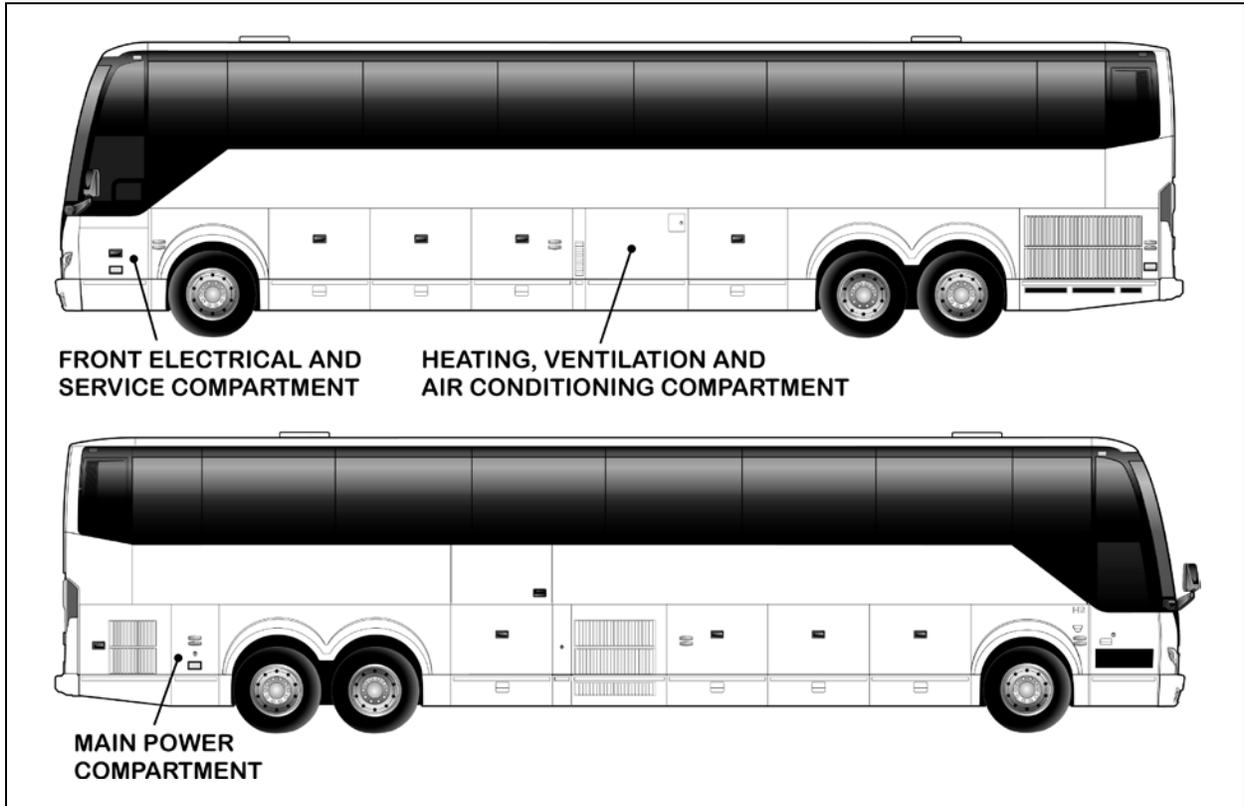
FIGURE 17: ELECTRICAL COMPARTMENTS
