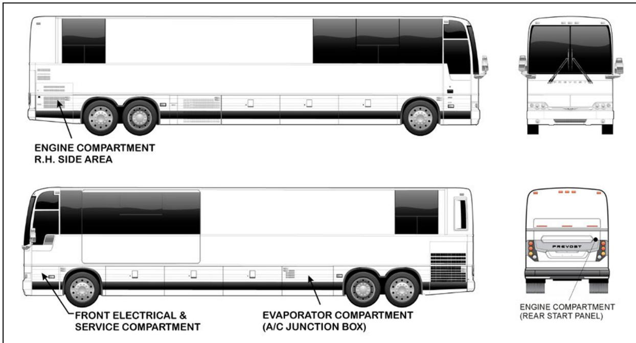
FIGURE 7: ELECTRICAL COMPARTMENTS (X3-45 VIP COMMERCIAL BUS SHELL)
