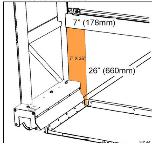
FIGURE 61: "NO DRILLING" ZONE (FORE AND AFT)
