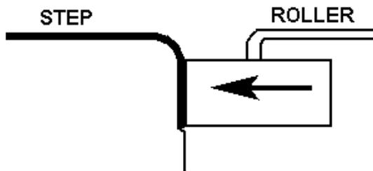
**GLUING OF WHITE SAFETY STRIP BETWEEN STEP AND “TARABUS” FLOOR COVERING**
