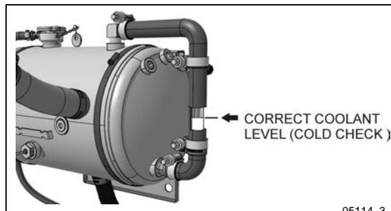
**FIGURE 14: SURGE TANK IN ENGINE COMPARTMENT**
