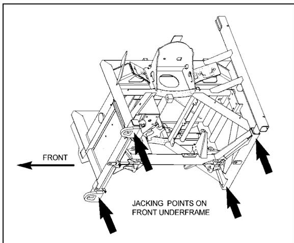
FIGURE 80: JACKING POINTS ON FRONT UNDERFRAME – IFS 18530
