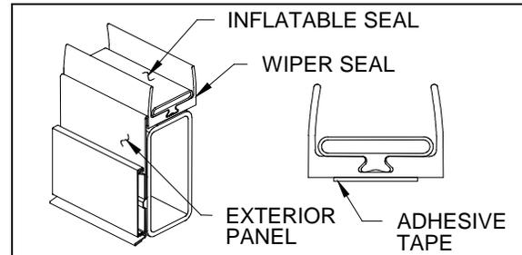
FIGURE 33: SEAL ASSEMBLY
