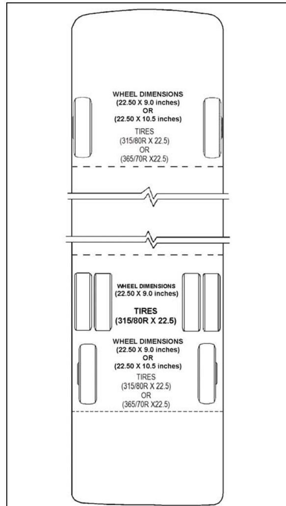
FIGURE 2: WHEEL ARRANGEMENT
