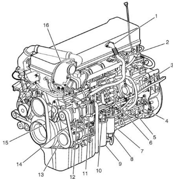
**FIGURE 2: D13H ENGINE OVERVIEW, ALTERNATOR SIDE (TYPICAL)**
