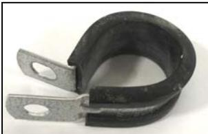
Figure 18: P-clamps are no longer used to secure power cables, but they can nevertheless be found on coaches of older generations. The piece of rubber that protects cable against the P-clamp steel loop must absolutely be in place. Replace any P-clamps where the rubber piece is missing, broken or likely to separate from the steel loop.
