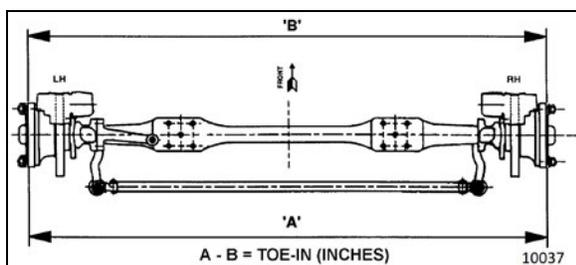
FIGURE 5: TOE-IN MEASUREMENT
