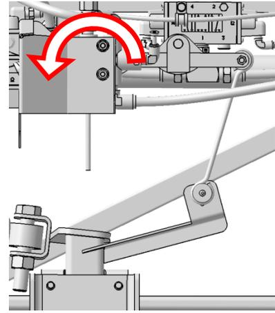
7. Allow 15 minutes to the air system to settle before measuring the resulting clearance. Repeat previous step if necessary.
