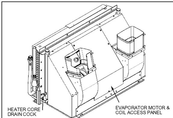
**FIGURE 18: PASSENGER'S UNIT EVAPORATOR COIL**
