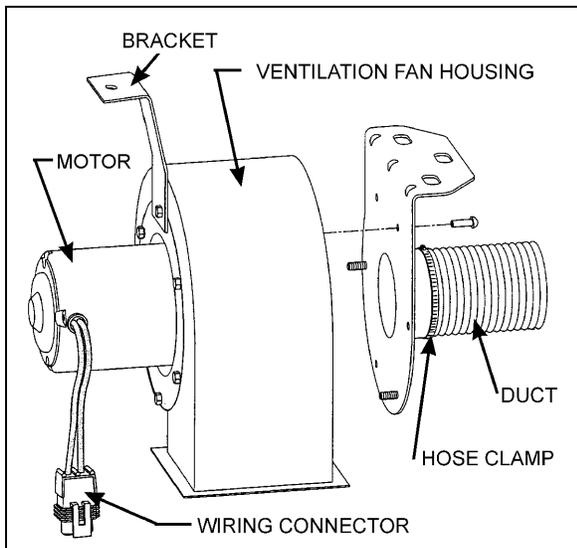
FIGURE 24: VENTILATION FAN INSTALLATION 23222
