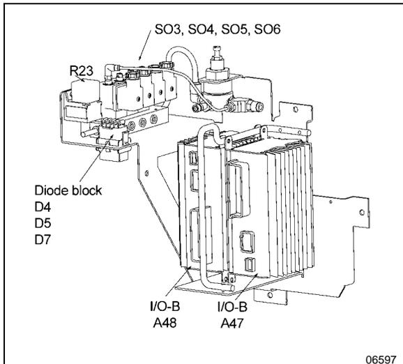
FIGURE 23 : PNEUMATIC ACCESSORY PANEL
