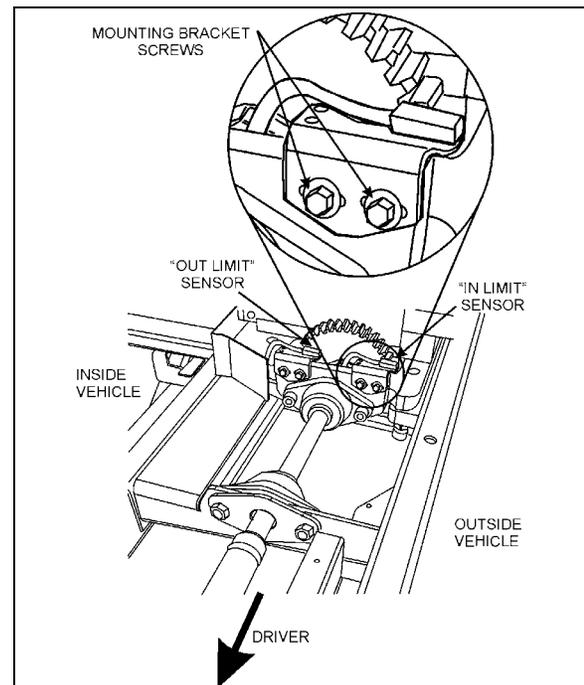
FIGURE 39: SLIDE-OUT SENSORS
