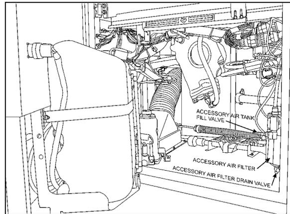
FIGURE 49: FRONT VALVE LOCATION ON X3 SERIES
