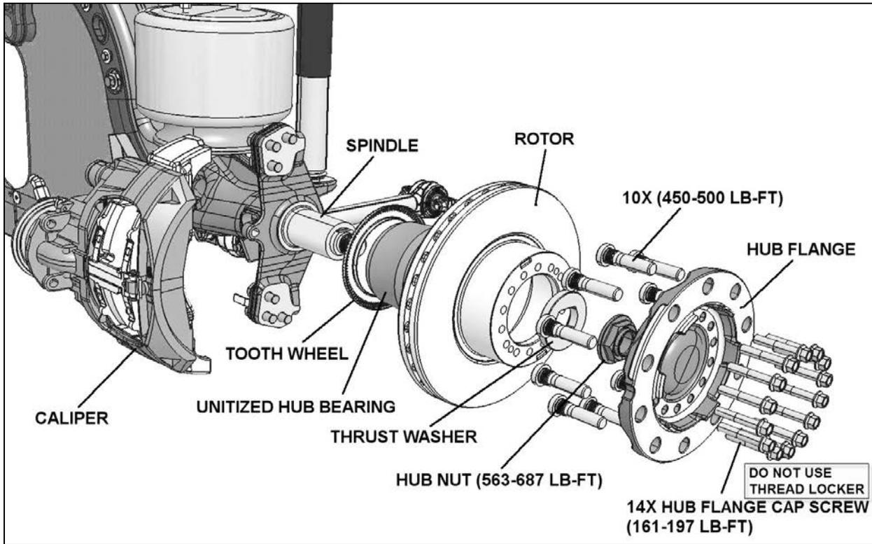
FIGURE 7: TAG AXLE HUB AND ROTOR ASSEMBLY
