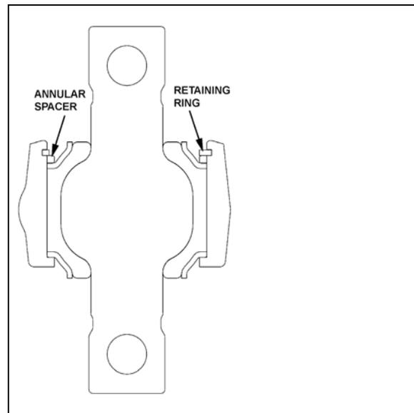
FIGURE 29: LOWER A-ARM BALL PIN BUSHING 16047
