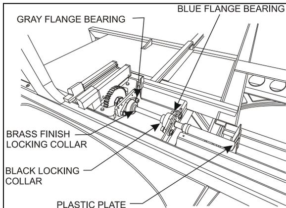
FIGURE 23: MECHANICAL COMPONENTS (TYPICAL)
