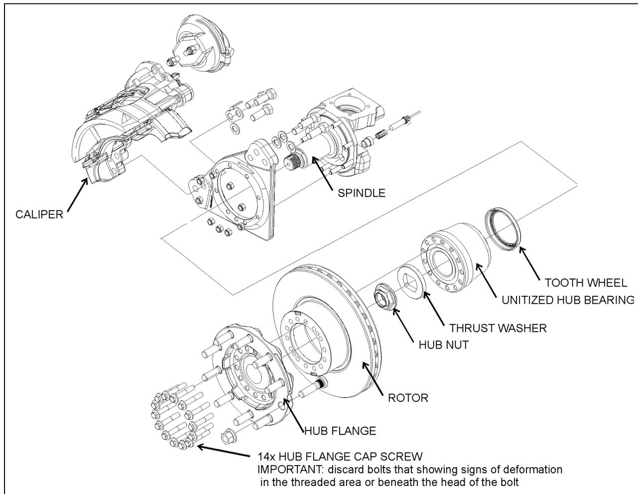
FIGURE 17: FRONT AXLE HUB AND ROTOR ASSEMBLY
