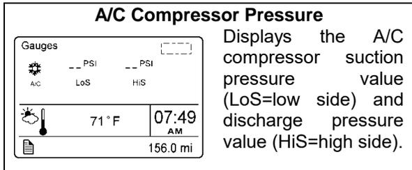
Displays the A/C compressor suction pressure value (LoS=low side) and discharge pressure value (HiS=high side).
