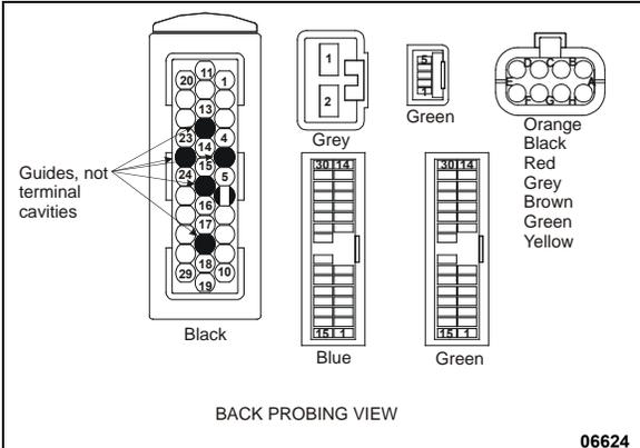
FIGURE 4: MULTIPLEX MODULE CONNECTOR PIN-OUT
