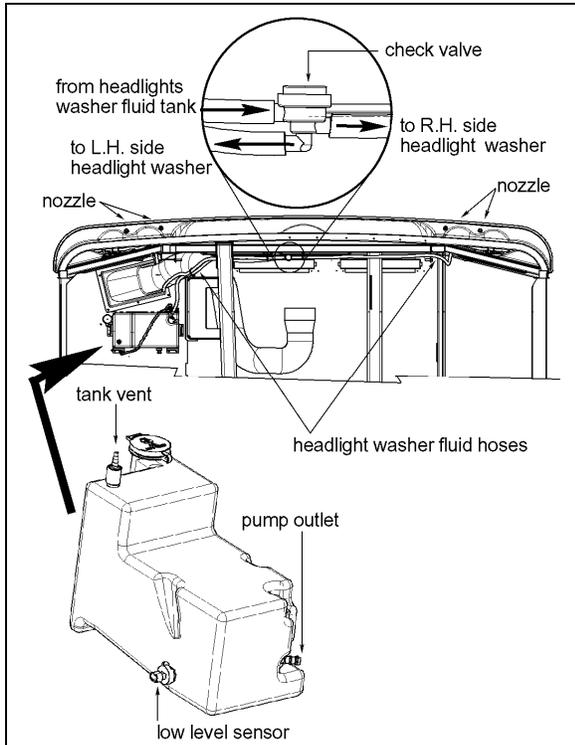
FIGURE 30: HEADLIGHTS CLEANING SYSTEM 23380
