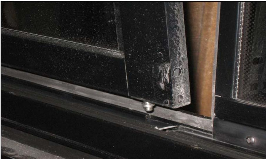
**FIGURE 65: DISENGAGING THE BOTTOM OF THE SASH**
