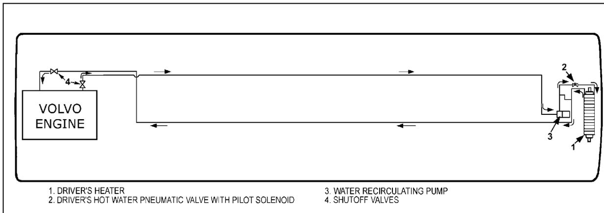
FIGURE 11: X3 SERIES SMALL HVAC SYSTEM - HEATING CIRCUIT
