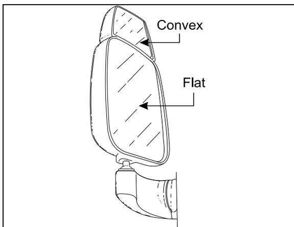
FIGURE 14: REAR VIEW MIRROR (RAMCO)
