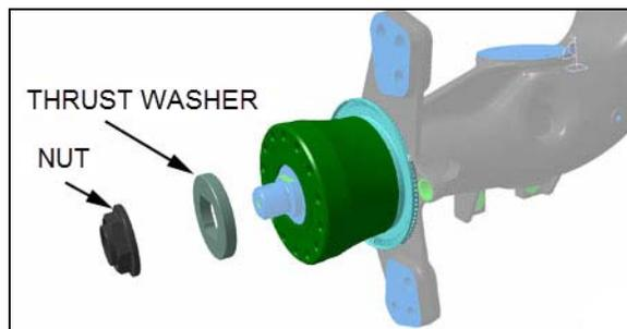
FIGURE 12: INSTALL THRUST WASHER AND HUB NUT
