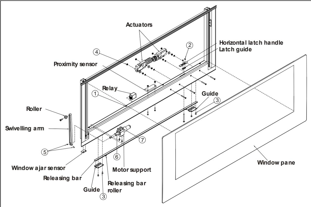
FIGURE 39: ELECTRIC AWNING WINDOW EXPLODED VIEW (SASH)
