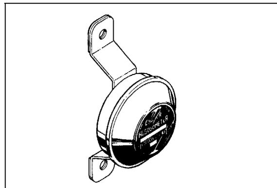
FIGURE 18: HUBODOMETER
