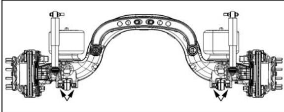
FIGURE 94: JACKING POINTS ON TAG AXLE OE H3B764
