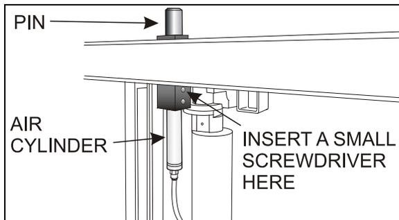
FIGURE 10: SECURITY PIN AIR CYLINDER REMOVAL
