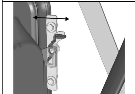
5. Check handle adjustment. Handle must remain tight against its plastic housing.
