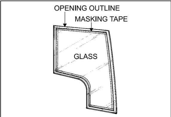
FIGURE 36: ADHESIVE-MOUNTED WINDOW 18080
