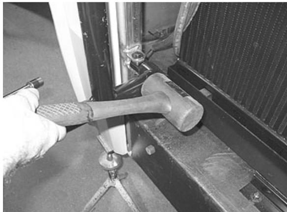
FIGURE 63: PANTOGRAPH ARM ADJUSTMENT
