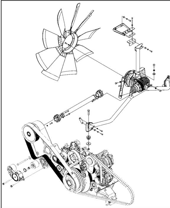
FIGURE 21: COOLING FAN DRIVE MECHANISM
