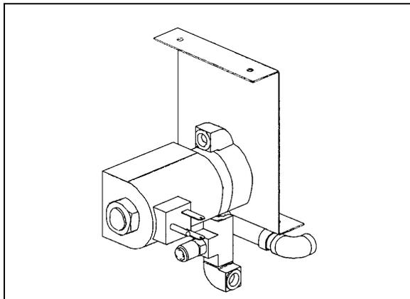
FIGURE 30: AIR HORN VALVE
