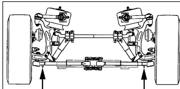
FIGURE 91: JACKING POINTS ON IND. SUSPENSION 16095
