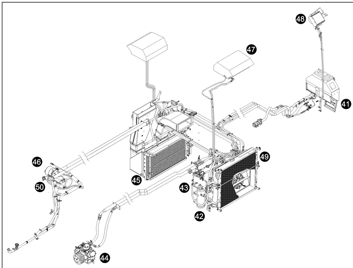
FIGURE 2: LUBRICATION AND SERVICING POINTS – HVAC UNIT
