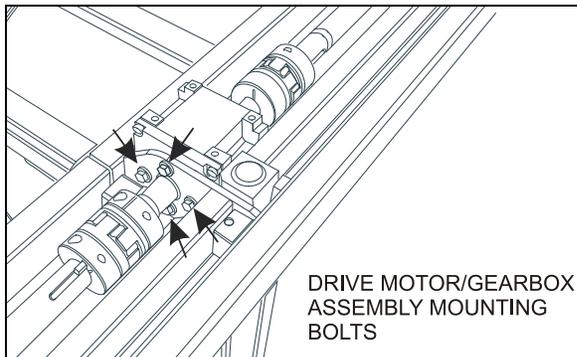
FIGURE 20: DRIVE MOTOR/GEARBOX ASSEMBLY MOUNTING BOLTS
