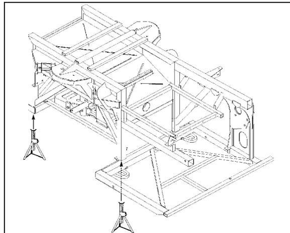
FIGURE 89: FRONT END JACKING POINTS 18592
