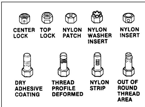
FIGURE 14: SELF-LOCKING FASTENERS
