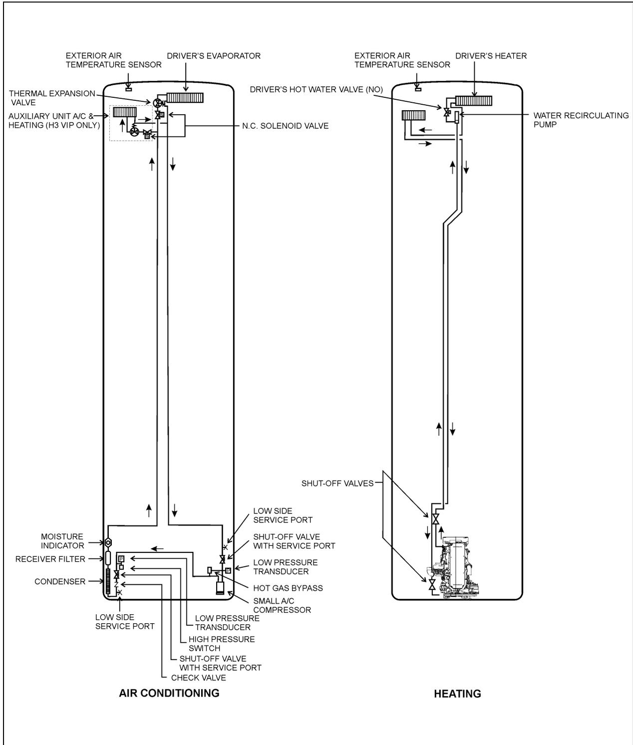
FIGURE 7: SMALL HVAC SYSTEM – HEATING AND AIR CONDITIONING
