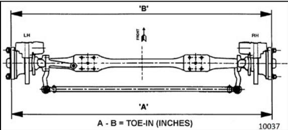
FIGURE 41: TOE-IN MEASUREMENT
