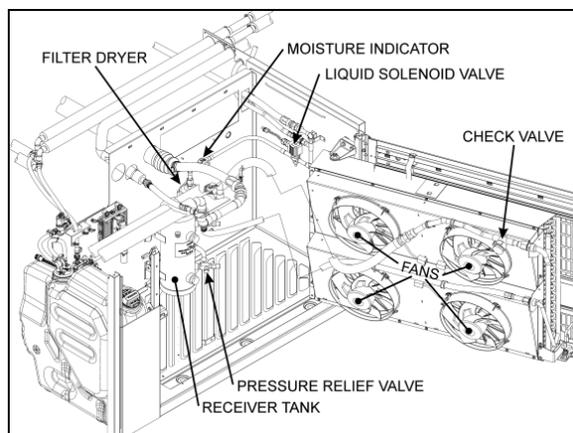
FIGURE 41: X3 SERIES CONDENSER COMPARTMENT<sup>22299</sup>
