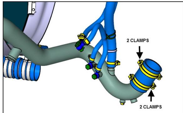
FIGURE 7: COOLANT LINE CONNECTED TO PUMP OUTLET
