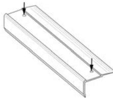
7. Clean top of step nosing using Sika 205 (refer to Section B).
