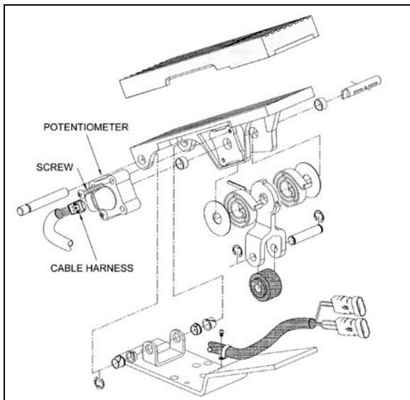
FIGURE 13: ELECTRONIC FOOT PEDAL ASSEMBLY 3035
