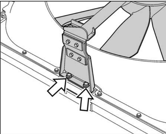
FIGURE 19: REMOVING UPPER FAN DRIVE SUPPORT BRACKET
