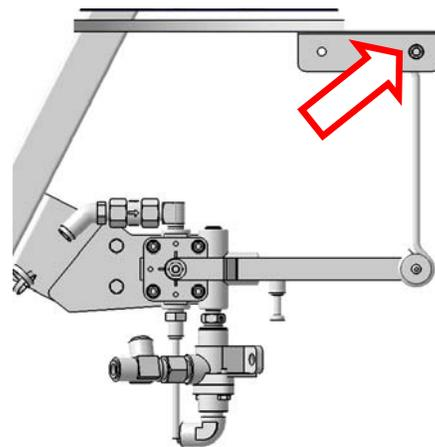
5. Loosen the lower mounting bolt shown.
