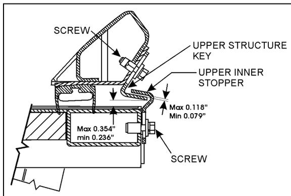
FIGURE 6: UPPER INNER STOPPERS ADJUSTMENT
