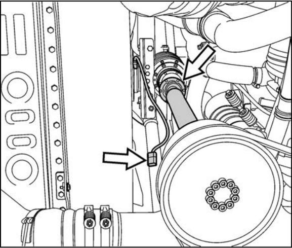
FIGURE 16: DISCONNECTING FAN DRIVE SHAFT
