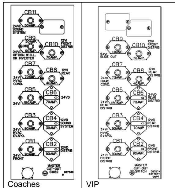
FIGURE 3: MAIN BREAKER PANELS – H3 SERIES
