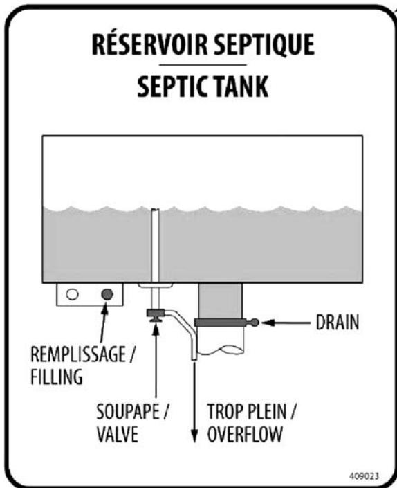
FIGURE 27: SUMP TANK &amp; F/W TANK SERVICE VALVES
