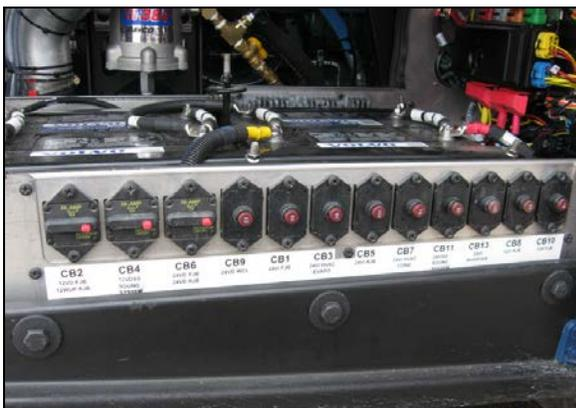
FIGURE 10: REAR ELECTRICAL JUNCTION PANEL
