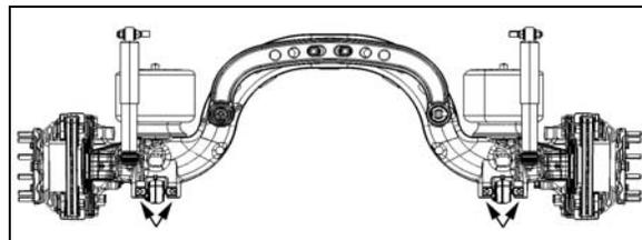
FIGURE 85: JACKING POINTS ON TAG AXLE
