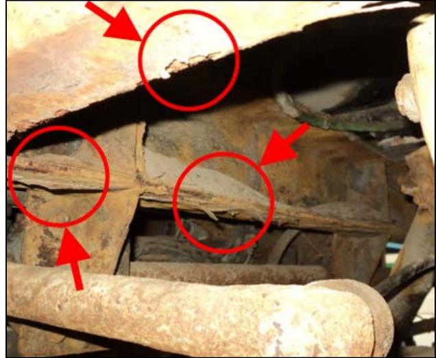
**FIGURE 3: METAL FLAKING AND ACCUMULATED SAND**
