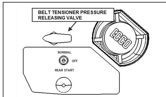
FIGURE 27: BELT TENSIONER CONTROL VALVE – X3 SERIES
