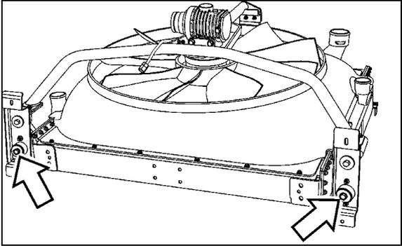
FIGURE 18: REMOVING FASTENERS
