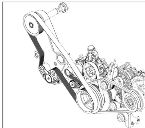
FIGURE 38: PULLEYS ARRANGEMENT 05146
