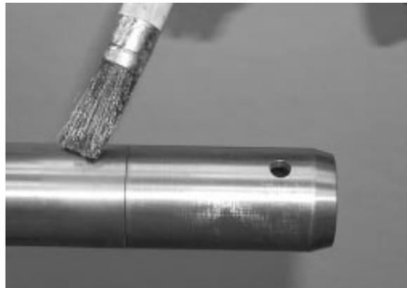
**FIGURE 19: APPLY GLEITMO 805 GREASE**
