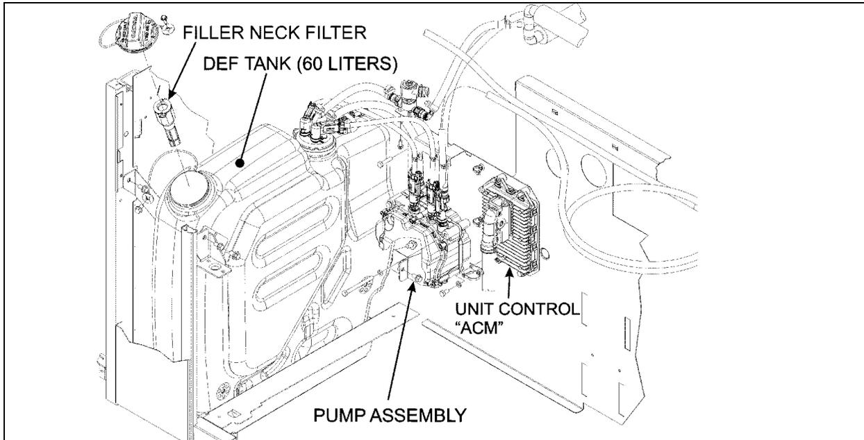
FIGURE 11 X SERIES DEF TANK AND PUMP
