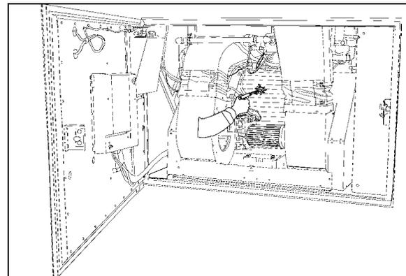
FIGURE 14: EVAPORATOR COIL CLEANING WITH LOW-PRESSURE AIR JET 22373
