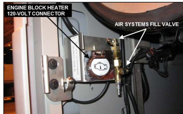
FIGURE 47: REAR VALVE LOCATION ON X3 SERIES
