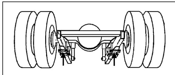
FIGURE 84: JACKING POINTS ON DRIVE AXLE 18085
