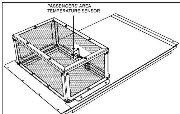
FIGURE 65: THERMISTOR SENSOR
