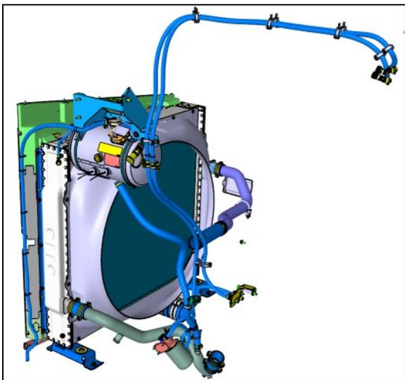
FIGURE 5: COOLANT FLOW TO RADIATOR (VOLVO D13)
