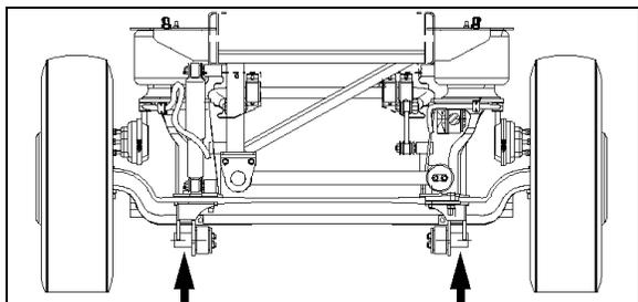
FIGURE 82: JACKING POINTS ON FRONT AXLE – I BEAM AXLE 10000
