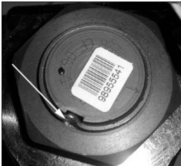
**FIGURE 20: FIXING NUT PUNCH MARK** 16098
