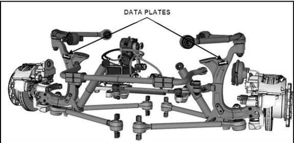
**FIGURE 5: IFS TYPICAL SERIAL & MODEL NUMBERS** 16136
