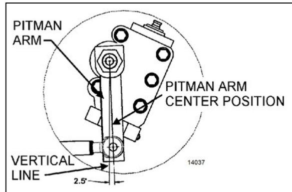
FIGURE 18: I-BEAM FRONT AXLE PITMAN ARM ADJUSTMENT
