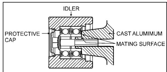
FIGURE 23: IDLER MOUNTED ON THE CAST ALUMINUM SUPPORT
