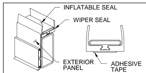
FIGURE 33: SEAL ASSEMBLY
