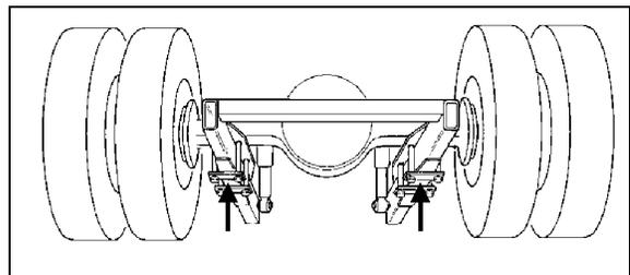
FIGURE 93: JACKING POINTS ON DRIVE AXLE OEH3B762
