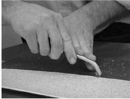
5. Add (about 6 inches) some length to the required length of filler bead to make the joint then cut.
