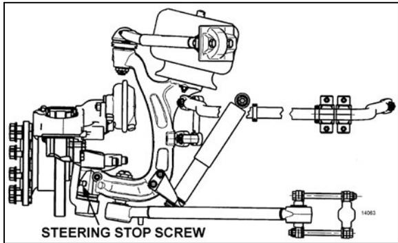
FIGURE 16: STEERING STOP SCREW ON IFS
