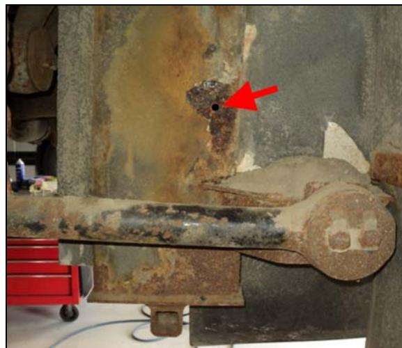
FIGURE 7: HOLE DRILLED IN STRUCTURAL MEMBER
