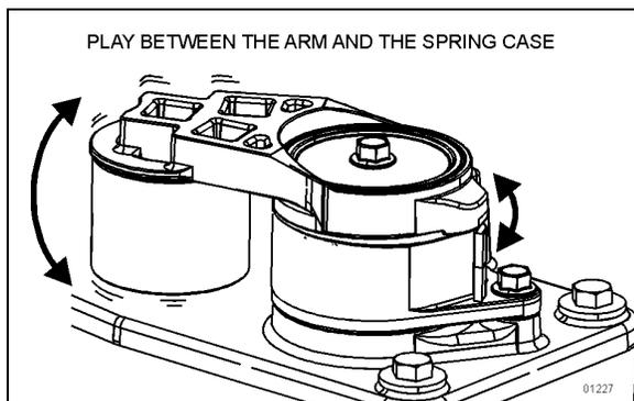
**FIGURE 16: CHECKING BUSHING WEAR**
