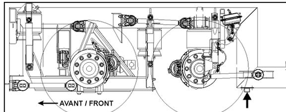
FIGURE 90: REAR END JACKING POINTS
