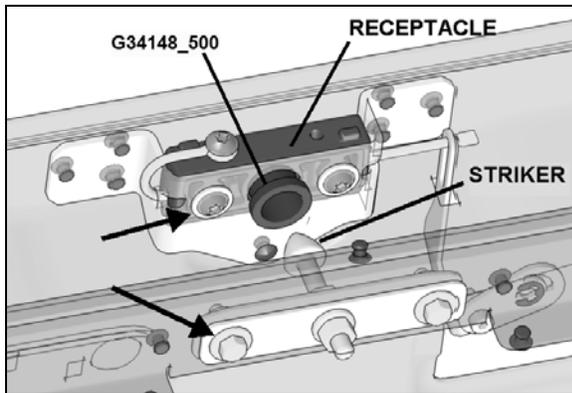
2. Close the door to center the latch mechanism.
