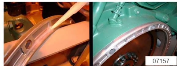
FIGURE 11: SPACER INSTALLATION
