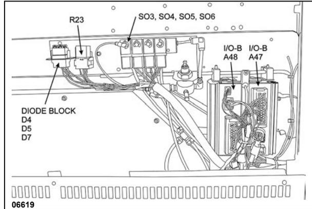
FIGURE 15: ENTRANCE DOOR & WIPER CONTROL PANEL
