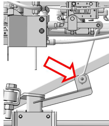
5. Loosen the lower mounting bolt shown.
