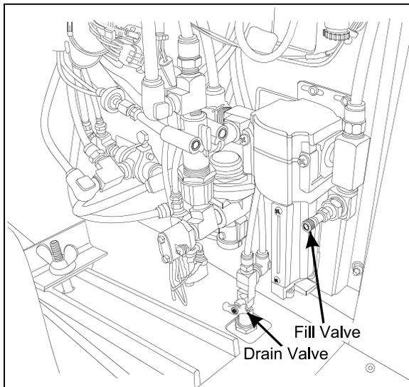
FIGURE 48: FRONT VALVE LOCATION ON H3 SERIES
