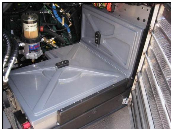
FIGURE 8: REAR ELECTRICAL PANEL, JUNCTION PANEL & BATTERY COMPARTMENT
