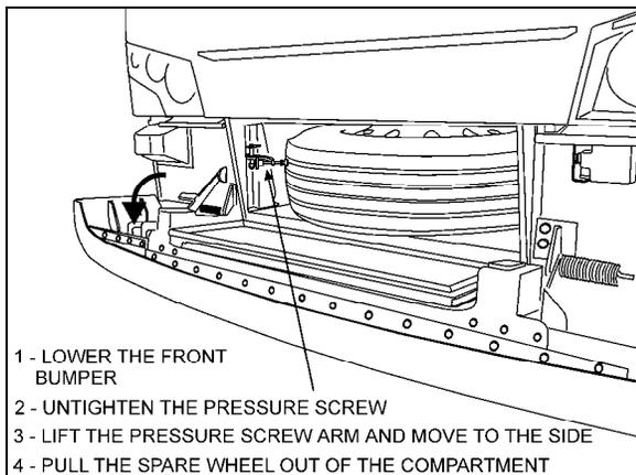
**FIGURE 30: H3 SERIES SPARE WHEEL AND TIRE**
