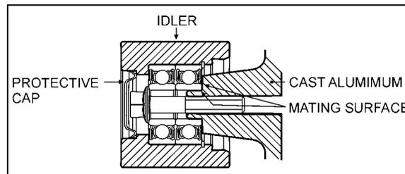
FIGURE 39: IDLER MOUNTED ON THE CAST ALUMINUM SUPPORT
