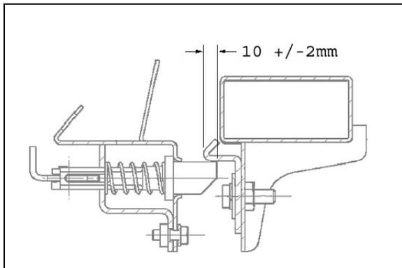
FIGURE 68: DOOR LATCHES ADJUSTMENT
