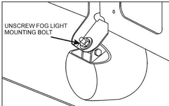
FIGURE 65: FOG LIGHT MOUNTING BOLT
