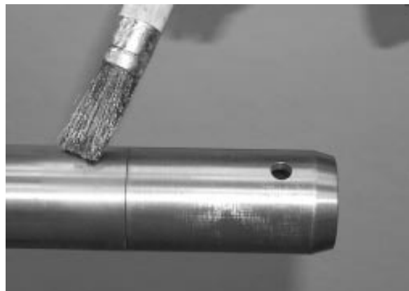
FIGURE 19: APPLY GLEITMO 805 GREASE
