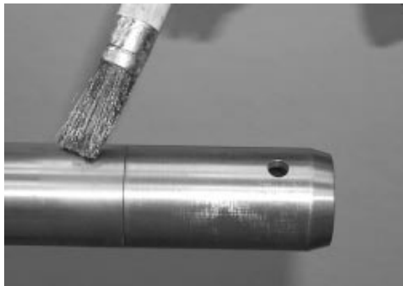
FIGURE 10: APPLY GLEITMO 805 GREASE
