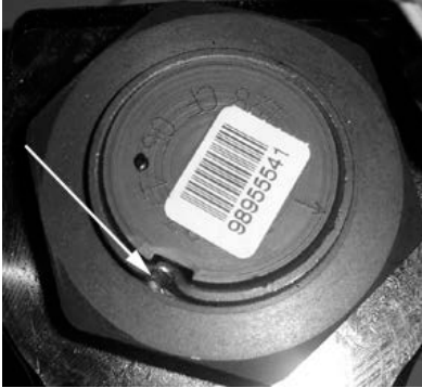
FIGURE 13: FIXING NUT PUNCH MARK
