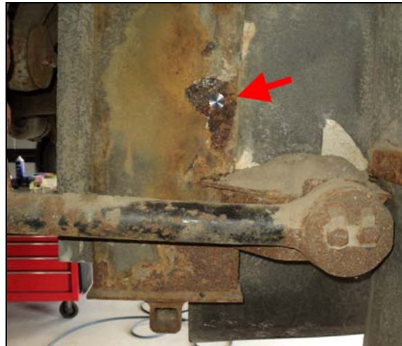
FIGURE 6: CLEANED SPOT ON STRUCTURAL MEMBER
