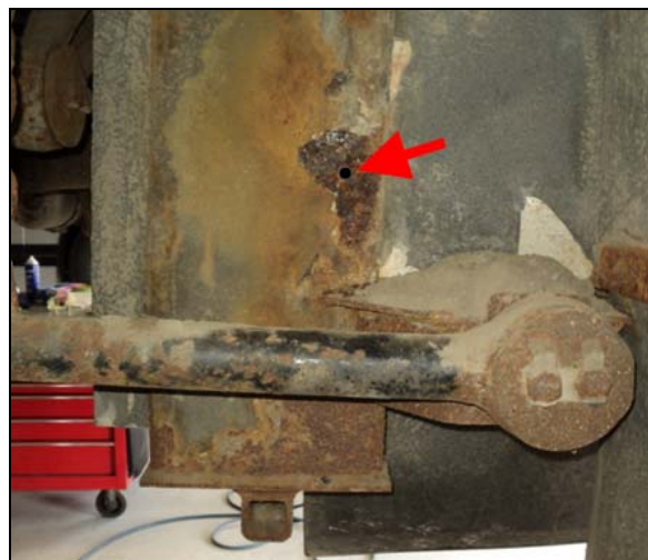
FIGURE 7: HOLE DRILLED IN STRUCTURAL MEMBER
