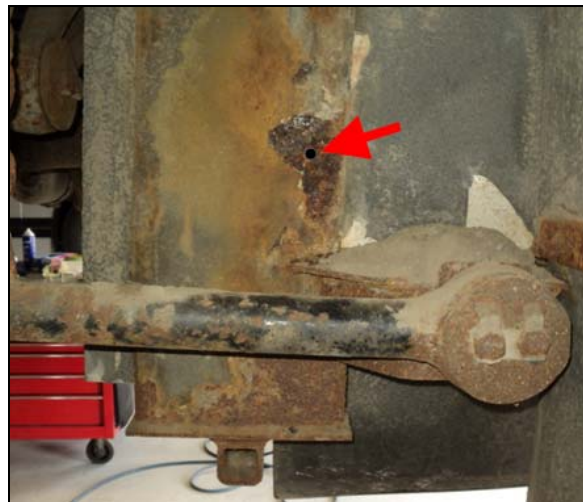
FIGURE 7: HOLE DRILLED IN STRUCTURAL MEMBER
