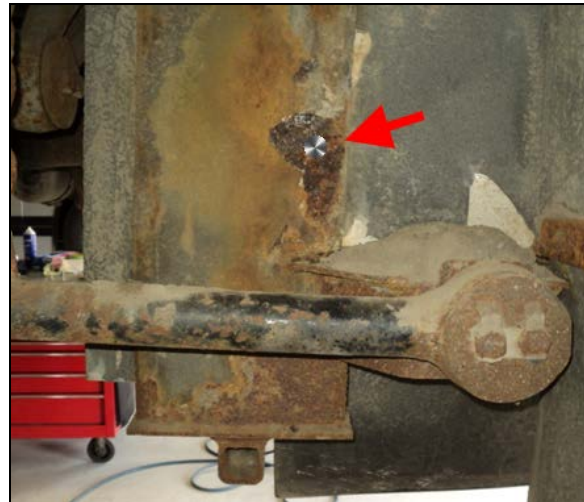
FIGURE 6: CLEANED SPOT ON STRUCTURAL MEMBER
