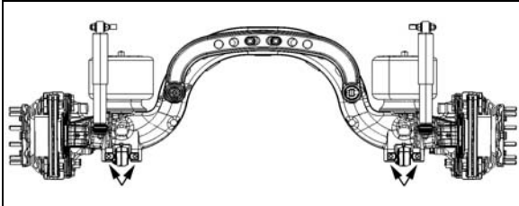
FIGURE 94: JACKING POINTS ON TAG AXLE OE H3B764
