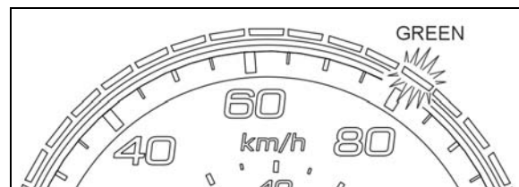
THE CRUISE SET SPEED IS 80 km/h
