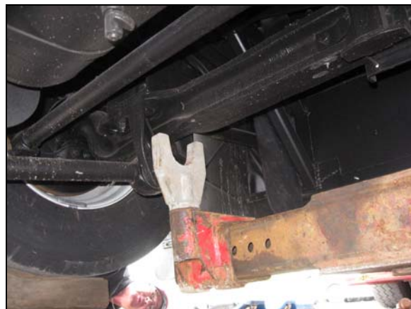
LIFTING FROM UNDER THE FRONT AXLE
