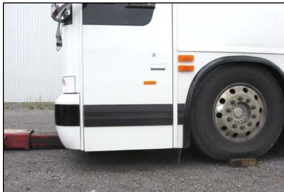
Tow eyes as lifting point
